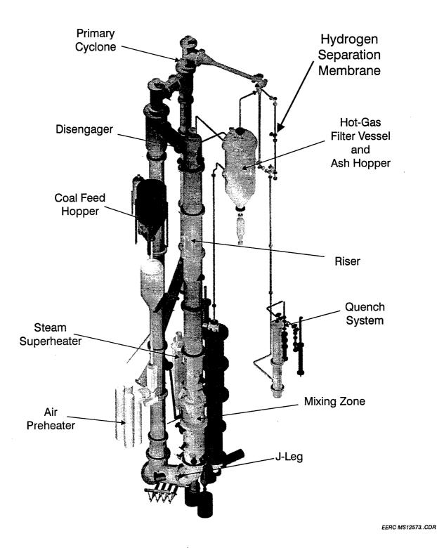
Figure 1. TRDU and hot-gas filter vessel in the EERC gasification tower.
