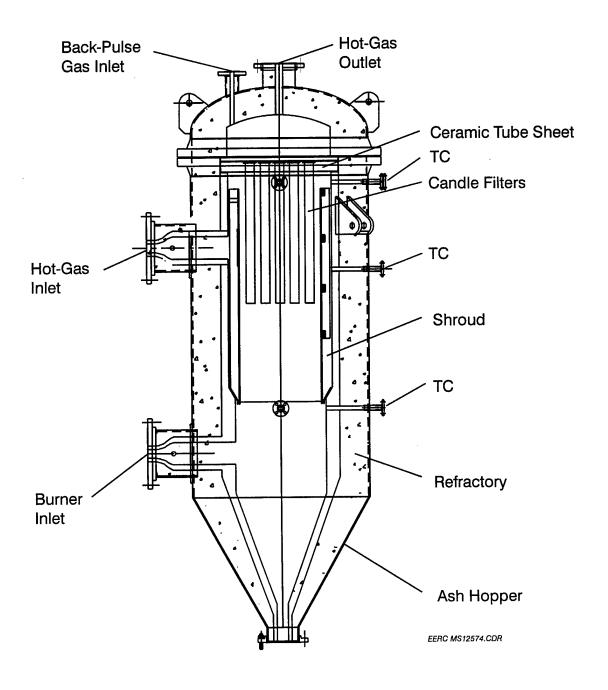
Figure 2. Schematic of the filter vessel design with internal refractory, tube sheet and shroud.
