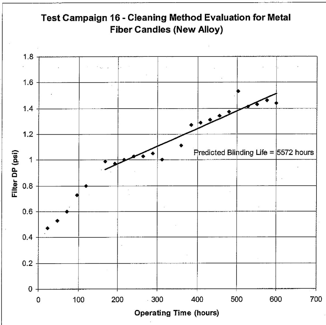
**Figure 4.2.17.1: Test Campaign 16 - Cleaning Method Evaluation for Metal Fiber Candles (New Alloy)**
