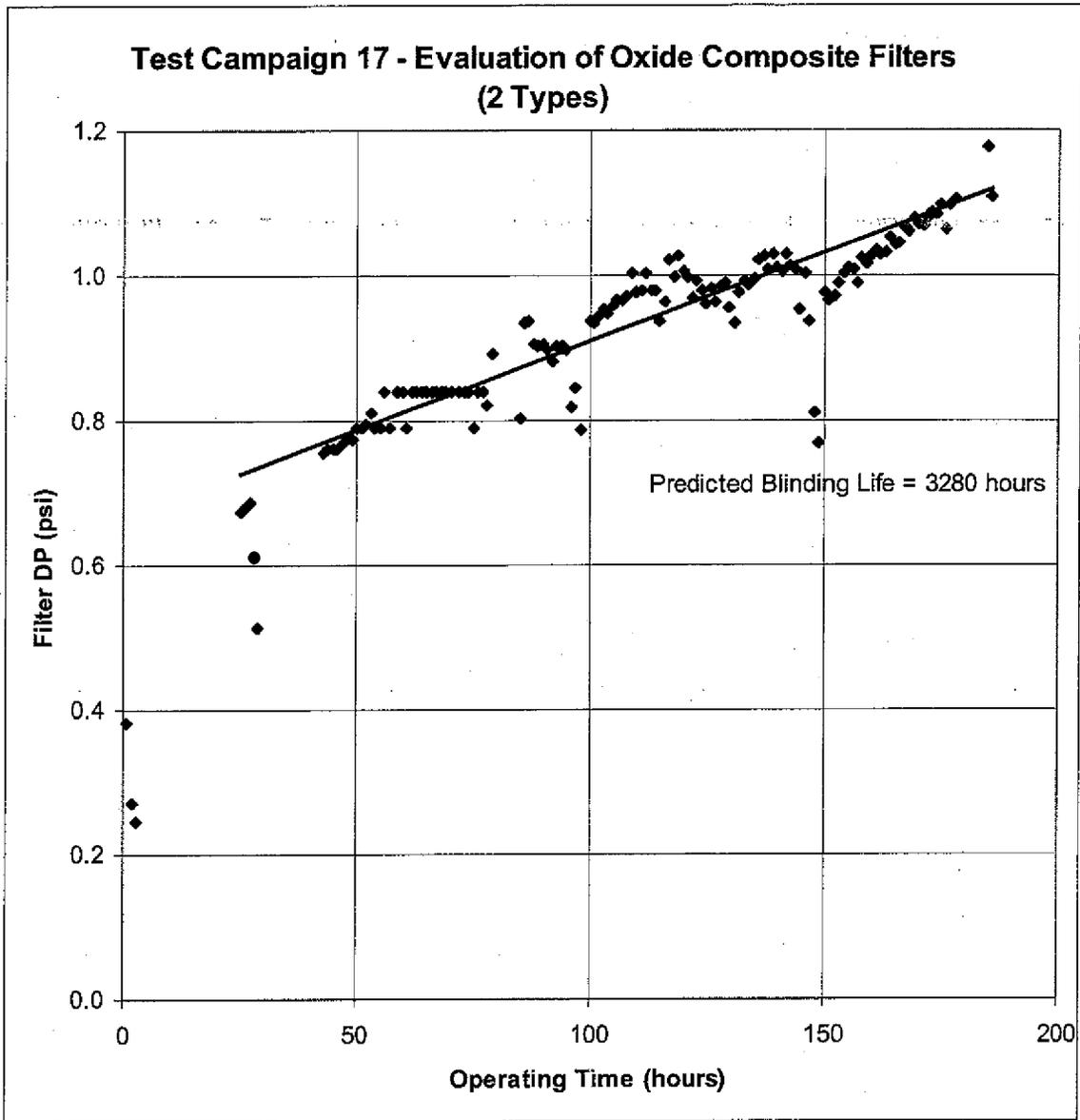
Figure 4.2.18.1: Test Campaign 17 - Evaluation of Oxide Composite Filters (2 Types)
