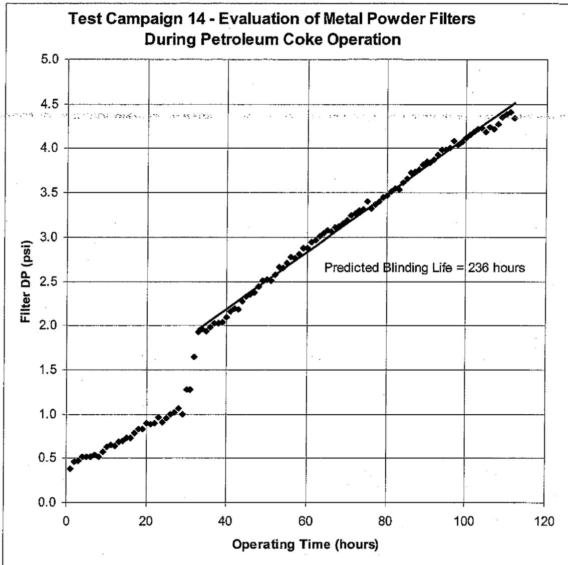
Figure 4.2.15.1: Test Campaign 14 - Evaluation of Metal Powder Filters During Petroleum Coke Operation
