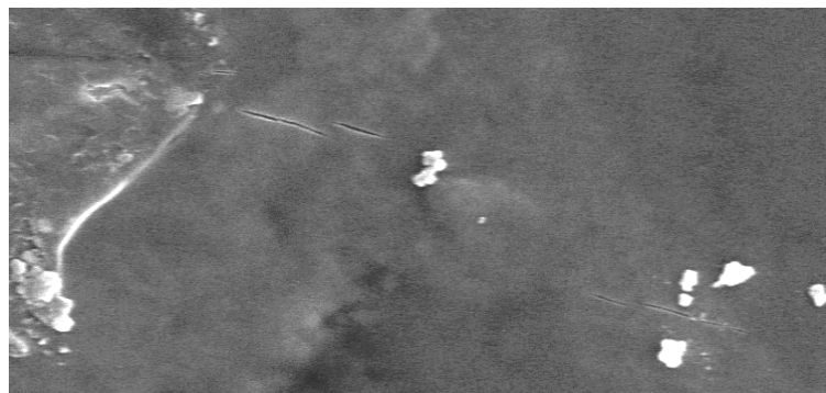
Figure 13. Crack bridging by dense region in the dual phase membrane.
