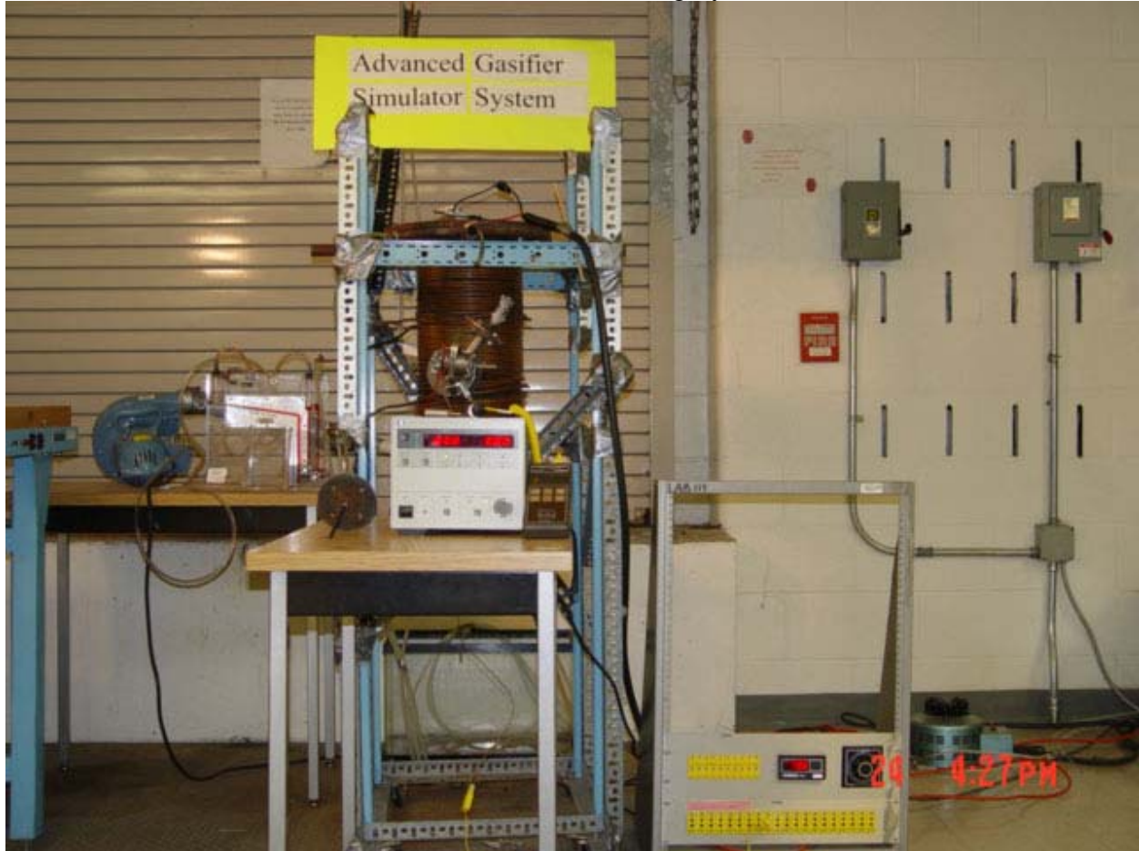
Figure 1. The Pictorial View of the Gasifier Simulator Test Facility With the Water Introducing System
