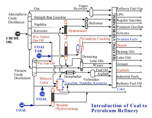
Figure 1. Possible integration of coal into existing refineries.
