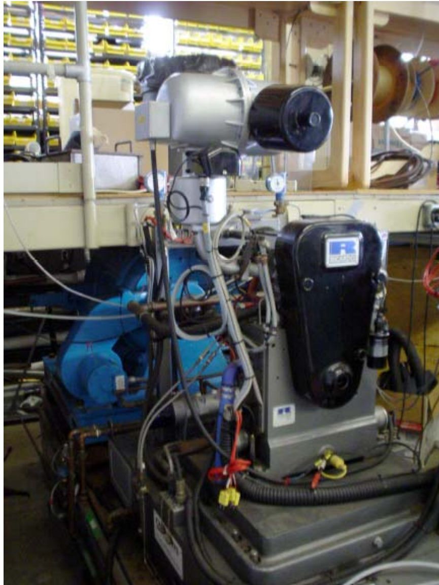
Figure 2 Ricardo "Hydra" Single-Cylinder Research Engine and Bedplate in the Diesel Combustion and Emissions Laboratory
