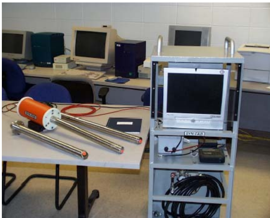
Figure 13. High-Temperature In-Furnace Camera System
