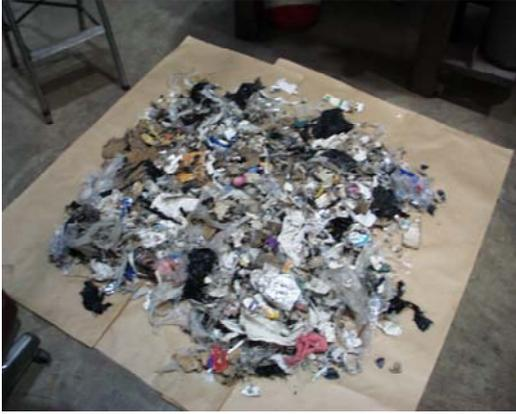
Figure B1: Paper, cardboard, and plastic film fraction in RDF
