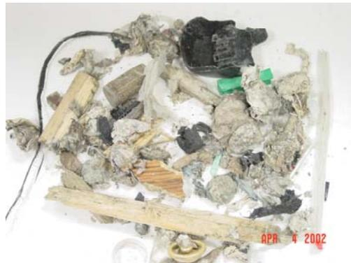
Figure B10: Combustibles in reject fraction from air-classification
