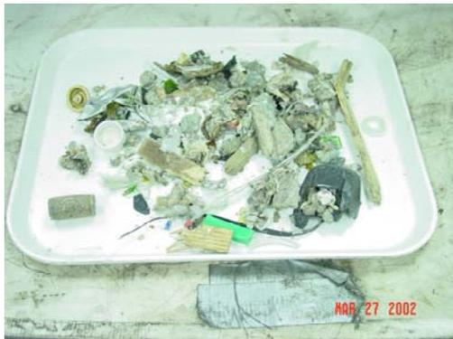
Figure B9: Heavy (reject) fraction from air-classification
