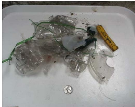
Figure B4: Container plastic fraction in RDF
