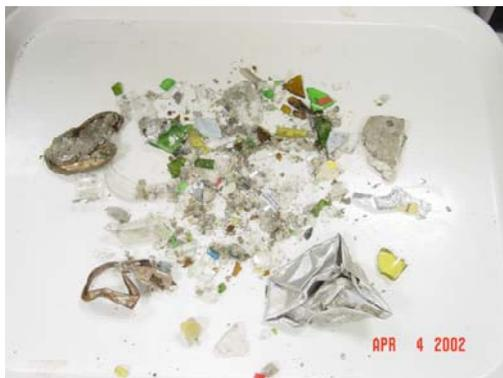
Figure B11: Non-combustibles in reject fraction from air-classification
