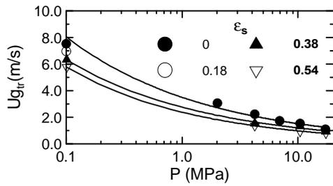
Figure 4. Effects of pressure and particle on the bubbling-jetting transition.
