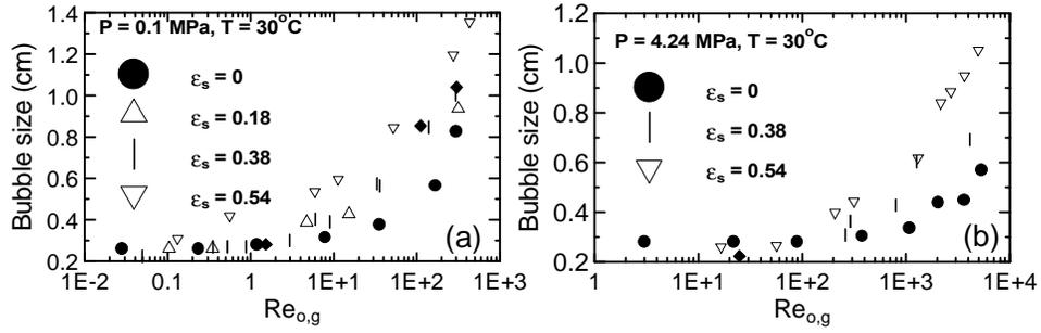
Figure 2. Effect of particles on the initial bubble size at various  $Re_{o,g}$ : (a)  $P = 0.1$  MPa; (b)  $P = 4.24$  MPa.
