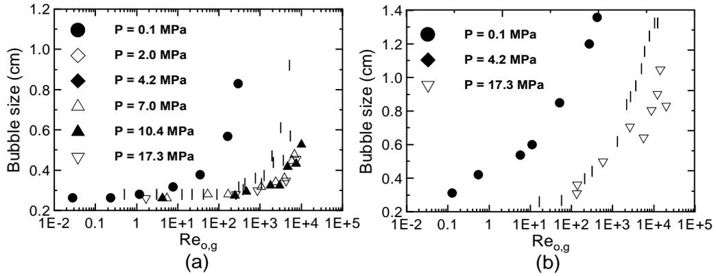
Figure 3. Pressure effects on the bubble formation (a) in liquid; (b) in liquid-solid suspensions,  $\epsilon_s = 0.54$ .
