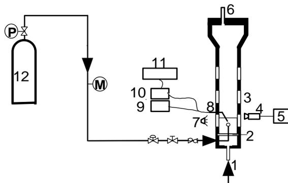
Figure 1. Schematic of the experimental setup. (1. Liquid inlet; 2. Perforated plate distributor; 3. Quartz windows; 4. High Speed Video camera; 5. TV and VCR; 6. Gas and liquid outlet; 7. Lighting; 8. Optical fiber probe; 9. Light source; 10. Photomultiplier; 11. Data acquisition system; 12. Nitrogen cylinder.)
