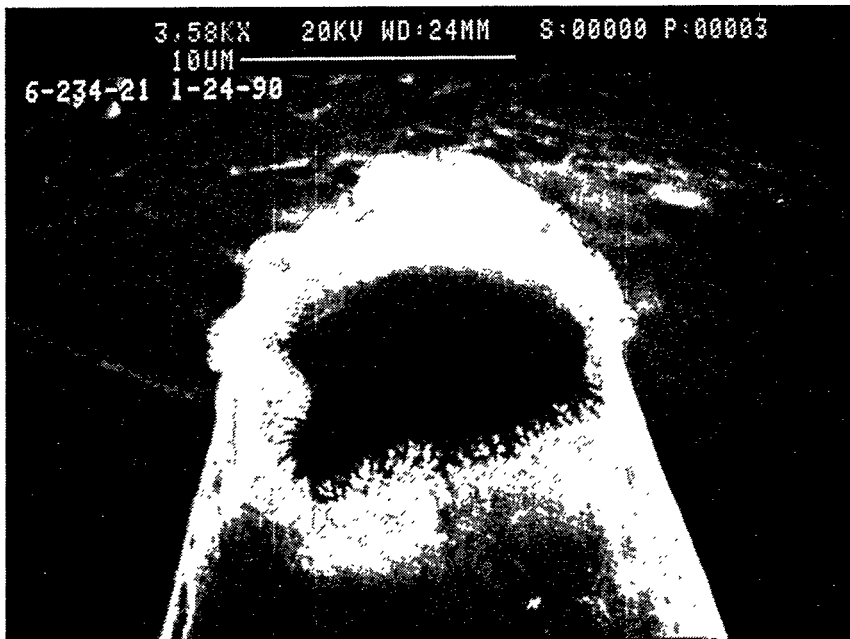
(b) Volcano after activation using a mixture of acetone, toluene, and butyl benzene.
