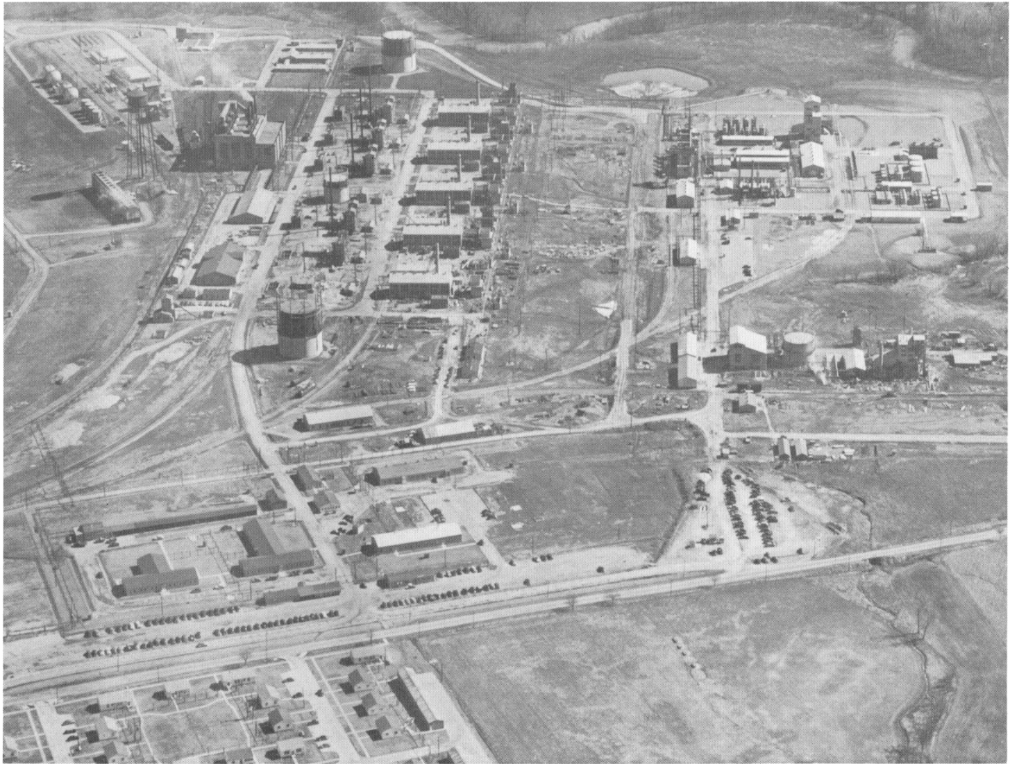
Figure 39. - Air view of coal-to-oil demonstration plants at Louisiana, Mo. Missouri Ordnance Works, upper left; hydrogenation plant, upper right; gas-synthesis plant, lower right; administration buildings and employee housing development, lower left.
