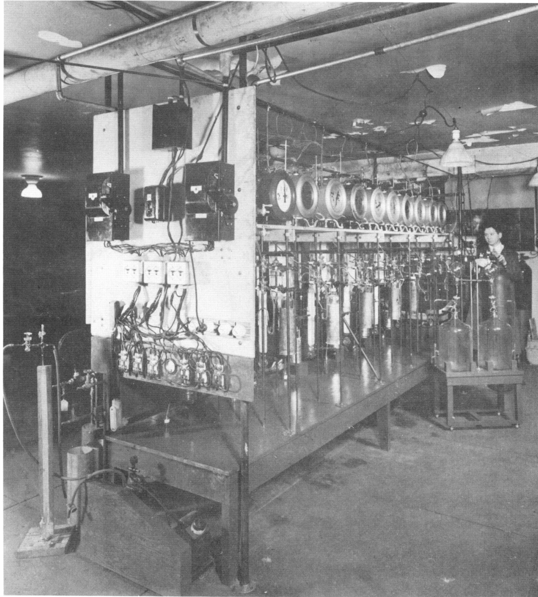
Figure 35.- Catalyst testing units. Rear view.
