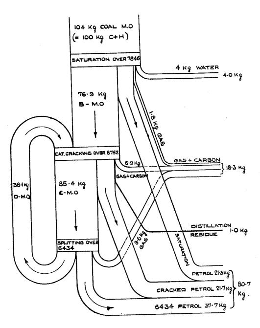
Other schemes cut out splitting hydrogenation completely and the middle oil component of the crude catalytically cracked product is recycled to the saturation hydrogenation stage. In this case the final petrol product tends to be too unsaturated and petrol from catalytic cracking has to be subjected either to a hydrogenation saturation process or to acid treatment.
