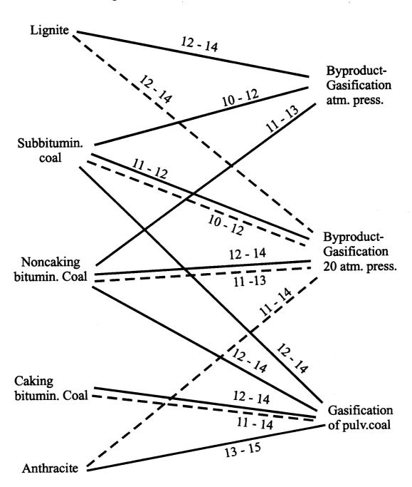
The following fields of application of the three principal methods of gasification can be clearly recognized:
