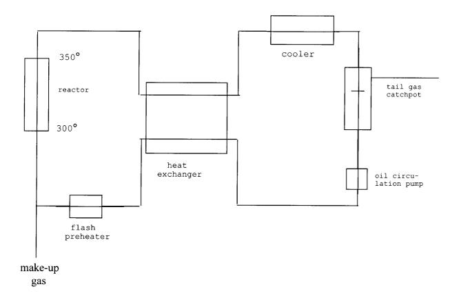
Depending on the temperature in the catchpot, the tail gas will carry some of the lighter boiling constituents, which can be returned into the oil circuit at any desired place, depending on the details of the production. The circulation oil can be set for a selected boiling range by suitable measures, in particularly by the catchpot temperature.
