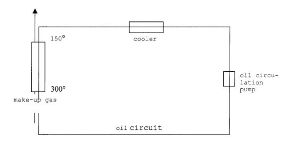
The wetting of the catalyst with oil does not merely result in maintaining definite measured catalyst temperature, but also regulates to a great extent the activity of the catalyst. The most active centers of the catalyst will have their activity reduced, which will
