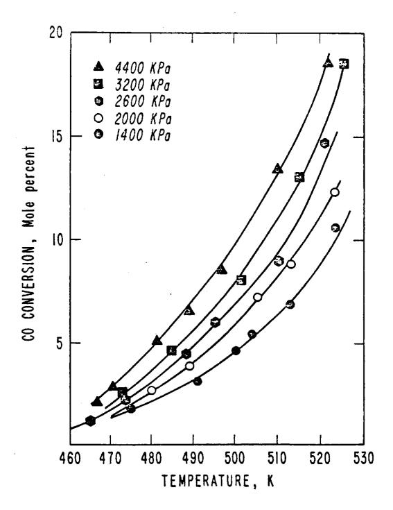
Effect of Temperature on Carbon Dioxide Yield Diluted Bed, Pseudo Slurry Reactor Pressure = 1400, 2600 and 4400 KPa;  $H_2/\text{CO} = 2/1; \text{ Space Velocity} = 1 \text{ cm}^3\text{g}^{-1}\text{s}^{-1};$  Heat Transfer Liquid Flow Rate (n-C16) = 0.103 cm $^3$ s<sup>-1</sup>.
