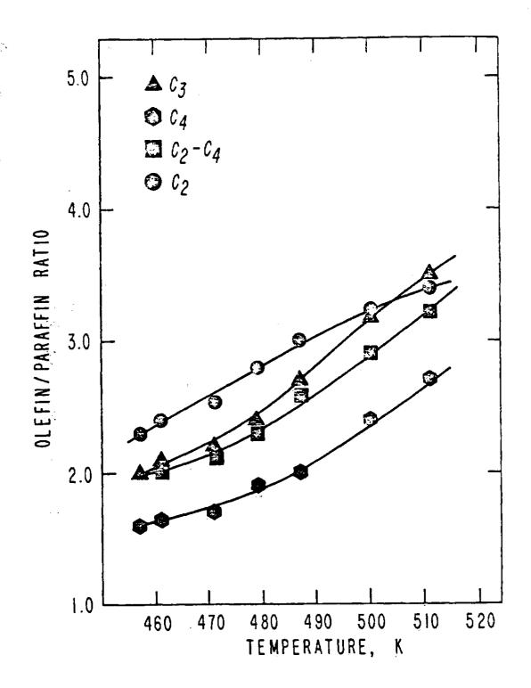
As the total reactor pressure increased the olefin to paraffin ratio of the  $\rm C_3$  and  $\rm C_4$  hydrocarbon fractions decreased and that of the  $\rm C_2$  hydrocarbon fraction increased.
