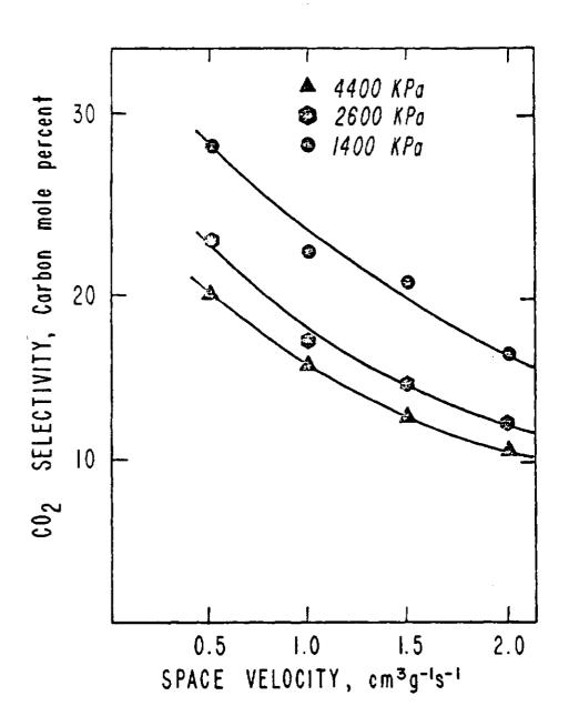
Effect of Space Velocity on Product Distribution Diluted Bed, Pseudo Slurry Reactor Temperature = 503 K;  $H_2/CO = 2/1$ ; Pressure = 1400 KPa; Heat Transfer Liquid Flow Rate  $(n-C16) = 0.103 \text{ cm}^3 \text{s}^{-1}$ .
