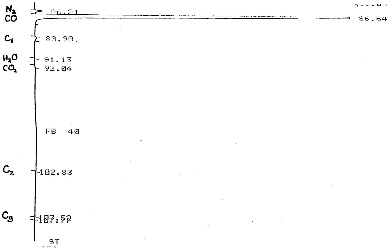
Figure 8. Typical Fixed Gases Analysis.
