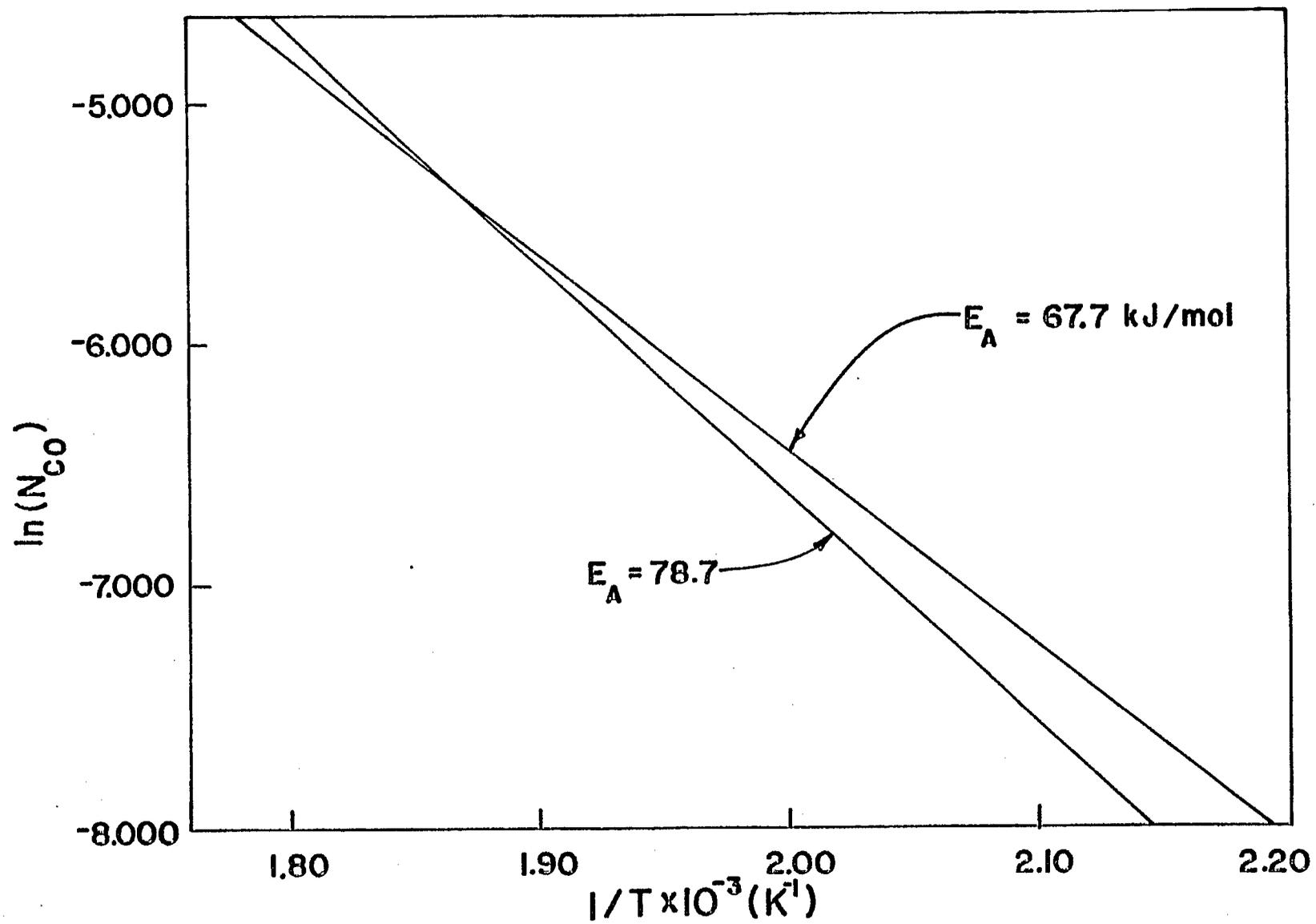
Figure 12. Activation Energy Plot for Co-B-A-101.
