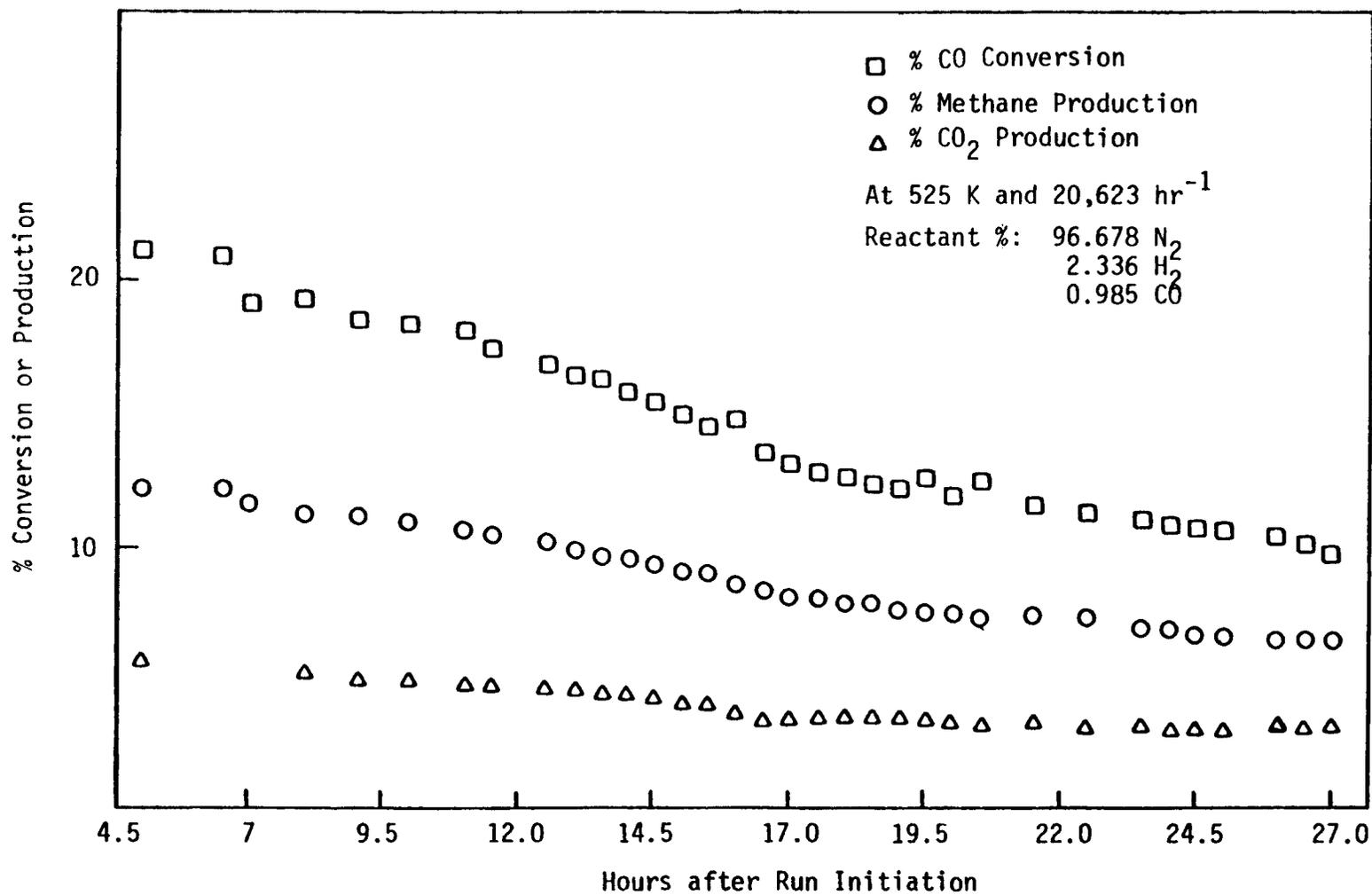
Figure 10. Percent CO Conversion, Percent CH<sub>4</sub> and CO<sub>2</sub> Production vs. Reaction Time for Co-B-A-101.
