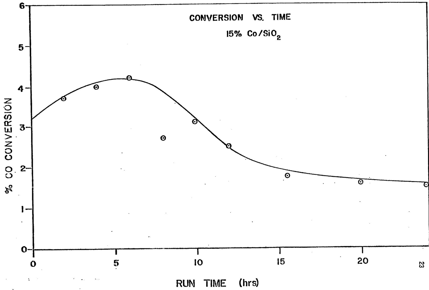
Figure 9. Percent CO Conversion vs. Reaction Time for Co-S-102.
