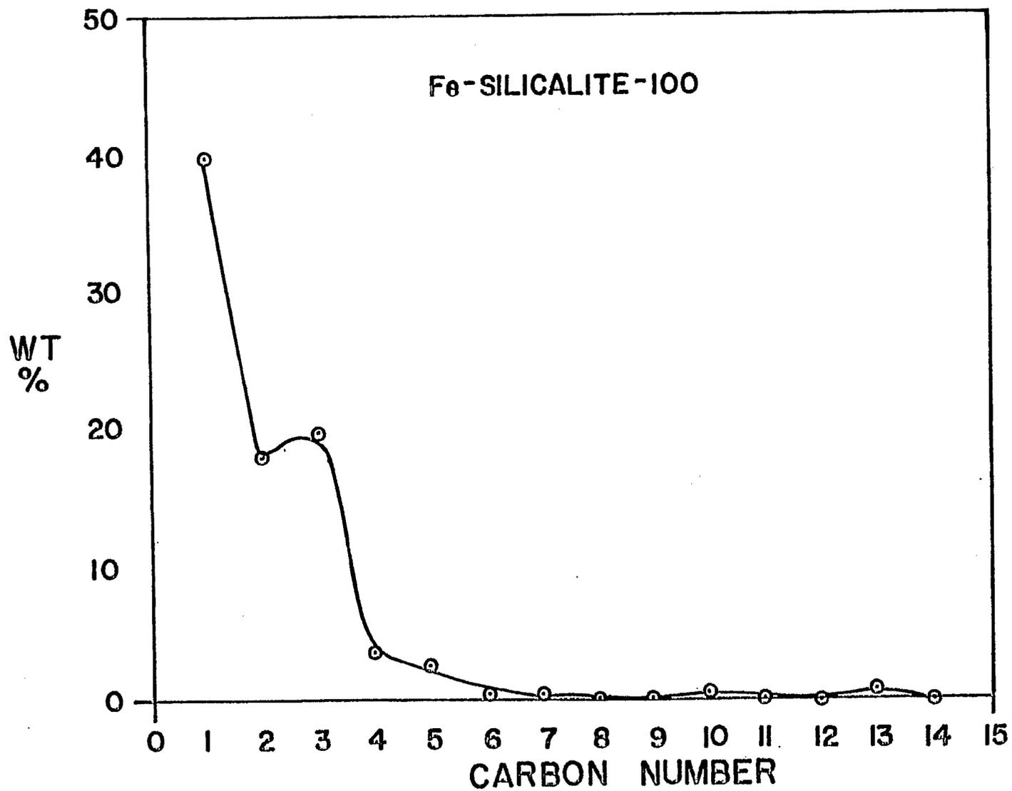
Figure 18. Product Distribution for Fe-Silicalite-100.
