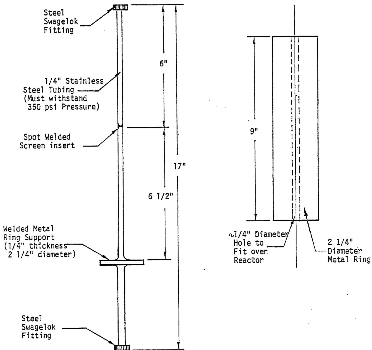
Figure 3. High Pressure Fischer-Tropsch Reactor.
