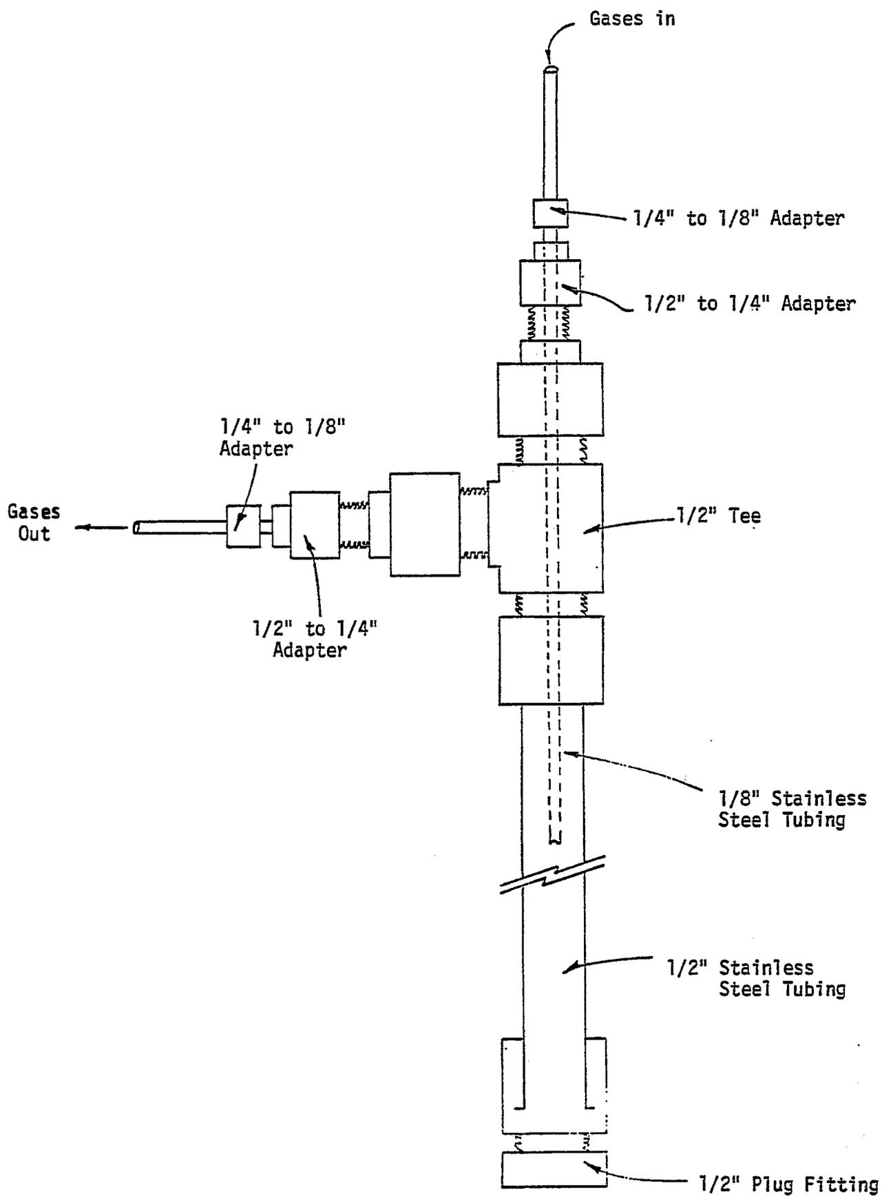
Figure 4. Liquid and Wax Trap.
