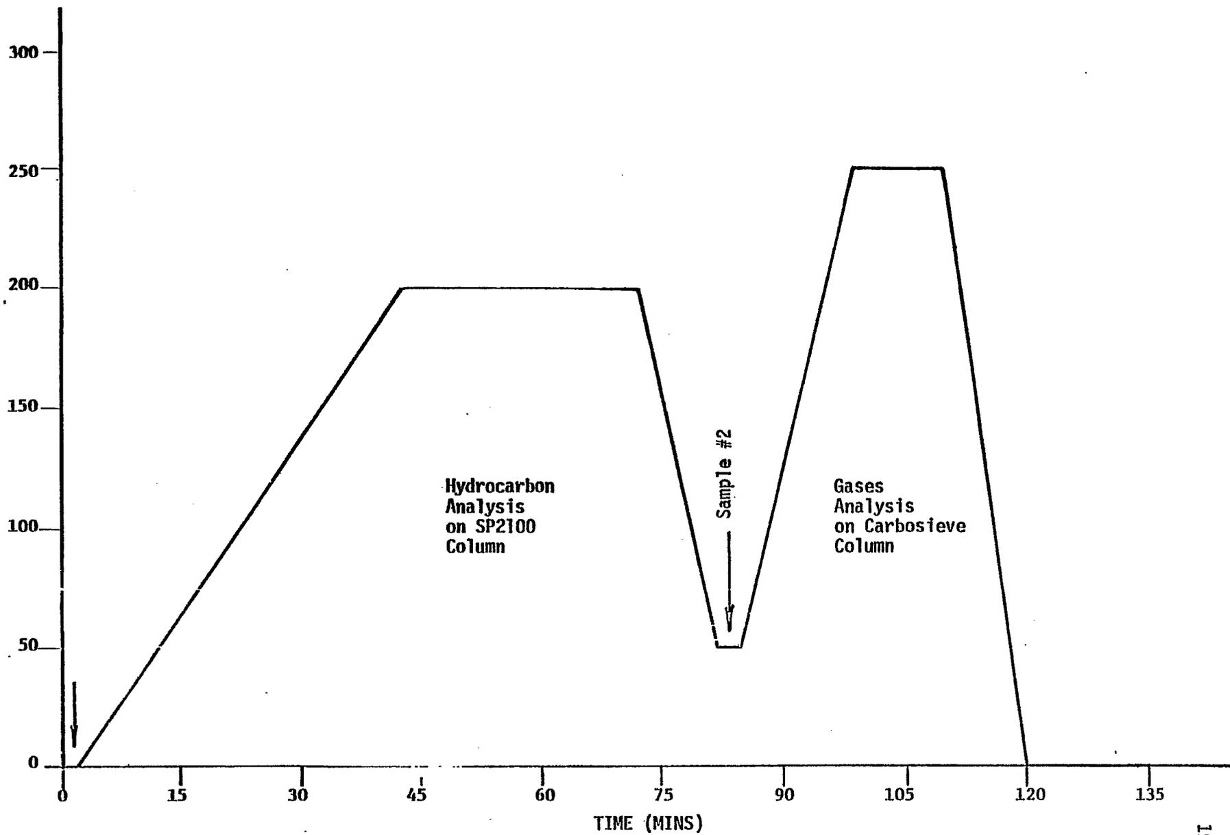
Figure 6. Temperature Program and Sampling Scheme for Chromatographic Analysis.
