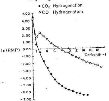
GHSV=1000 $h^{-1}$ , H<sub>2</sub>:CO or CO<sub>2</sub>=1:1., T=200°C., P=320psig. 2% Ru. Activated with flowing H<sub>2</sub> for 20h at 200°C.
