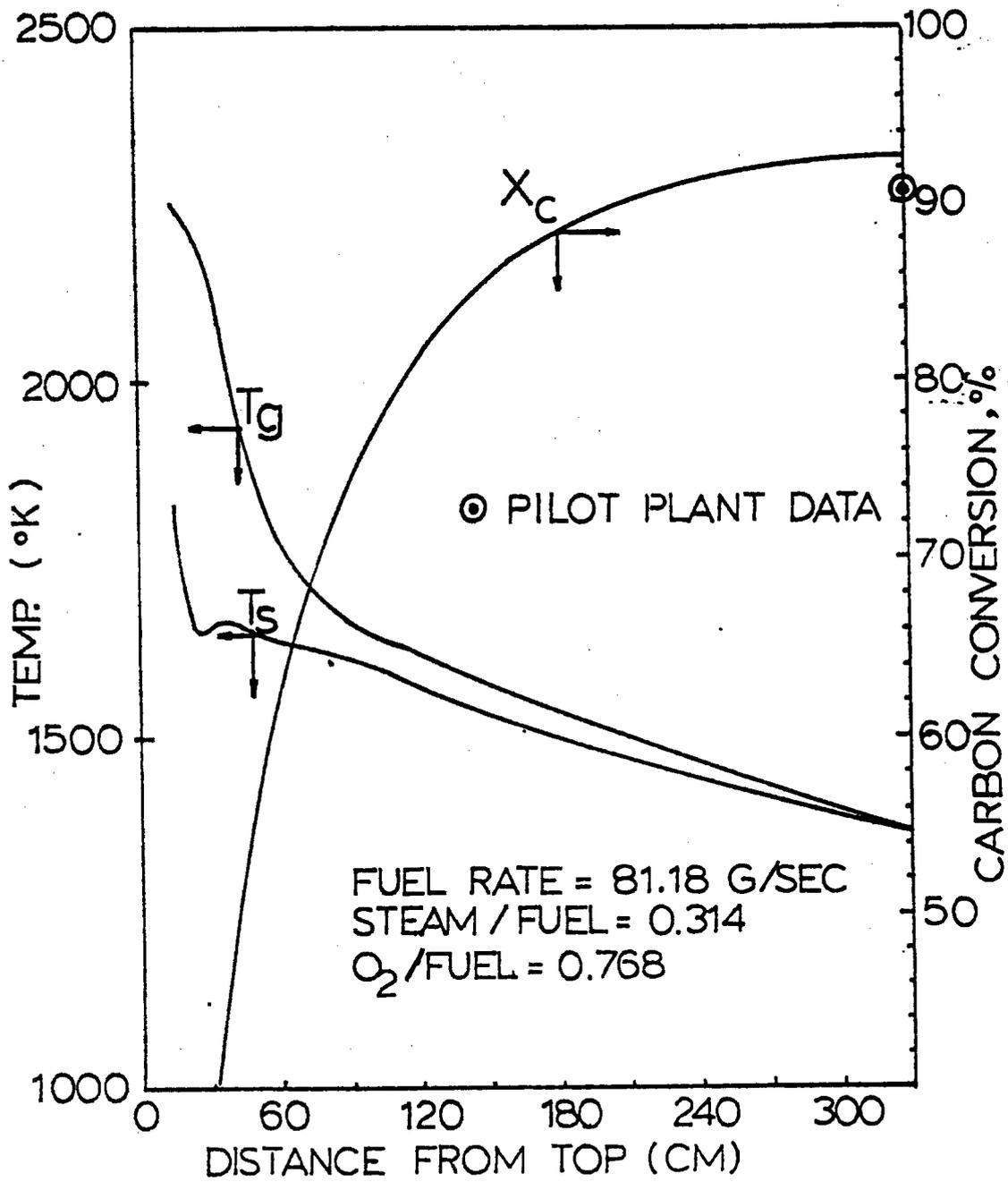
FIGURE 15(A) CALCULATED TEMPERATURE PROFILES AND CARBON CONVERSION PROFILE IN TEXACO PILOT PLANT GASIFIER FOR I-2 RUN
