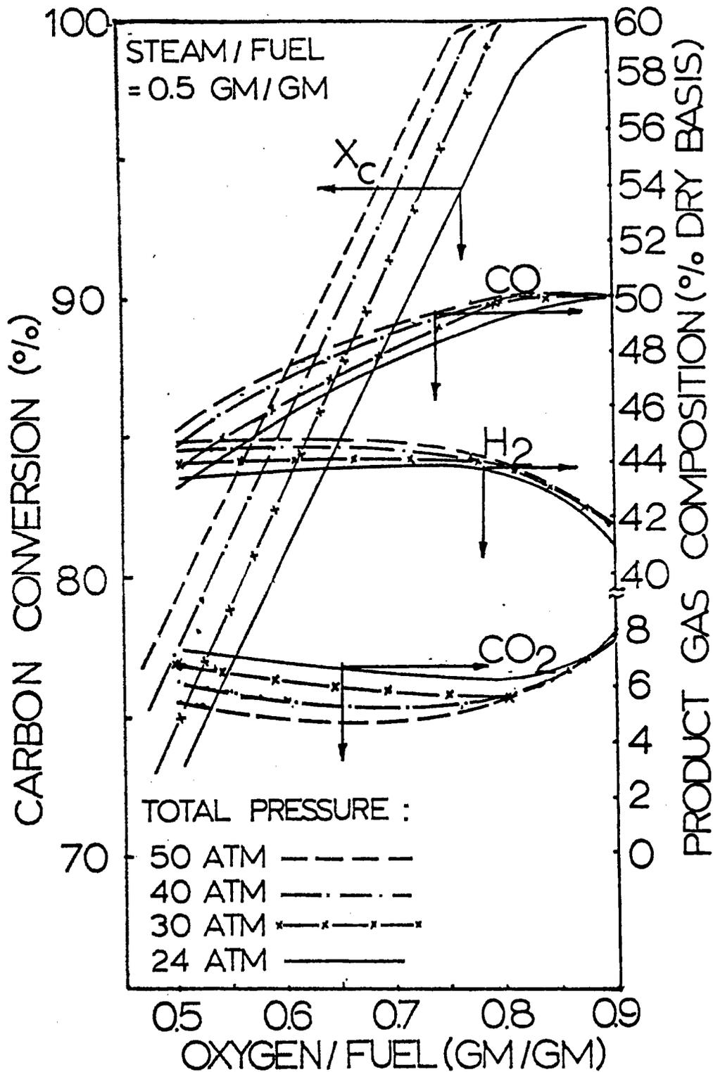
FIGURE 34 EFFECT OF TOTAL PRESSURE ON CARBON CONVERSION AND MAJOR PRODUCT GAS COMPOSITION AT VARIOUS OXYGEN/FUEL RATIOS WITH STEAM/FUEL = 0.5 GM/GM FEEDING H-COAL RESIDUE FROM ILLINOIS NO. 6 COAL IN THE TEXACO PILOT PLANT GASIFIER
