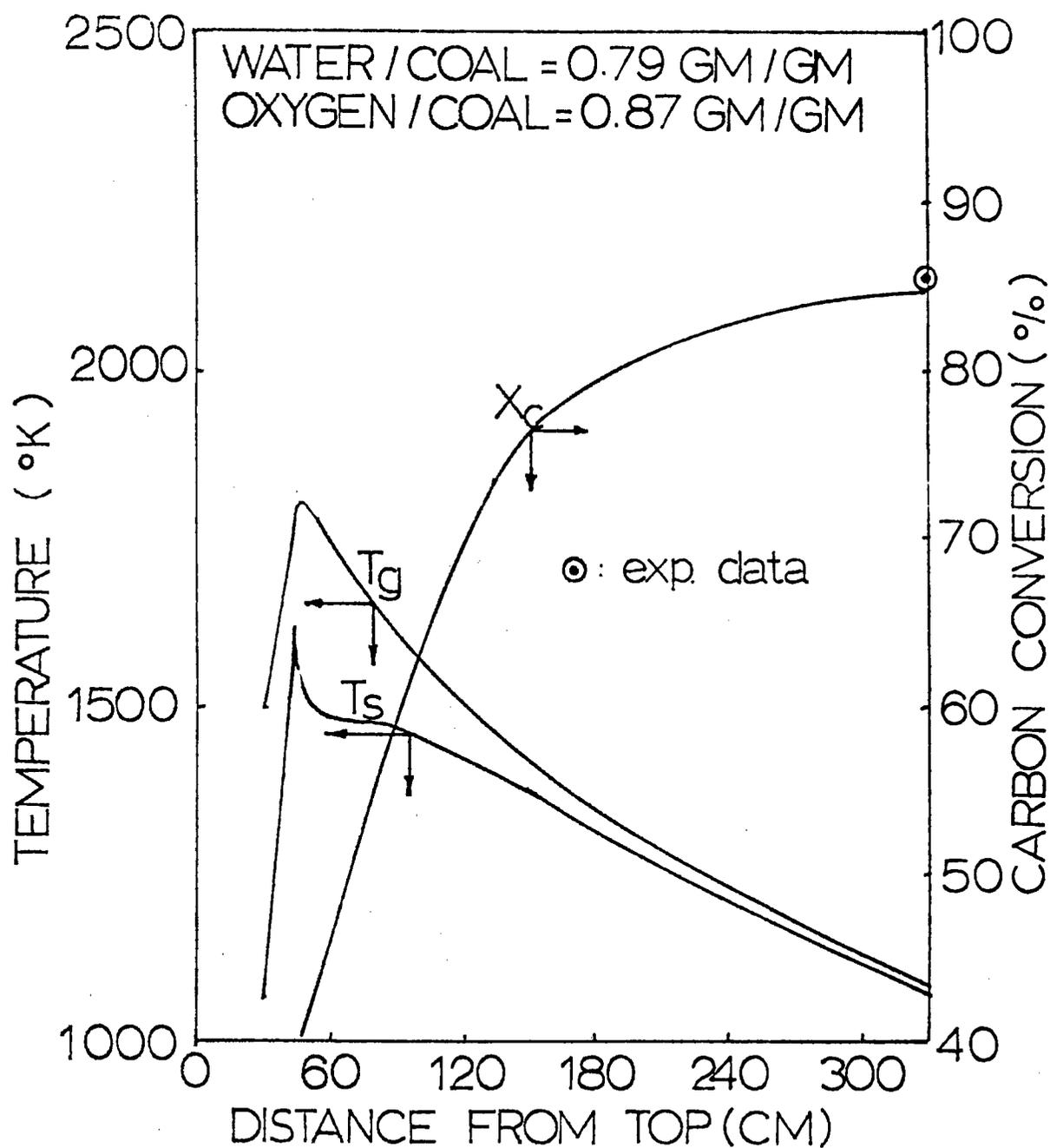
FIGURE 20(A) CALCULATED TEMPERATURE AND CARBON CONVERSION PROFILES IN TEXACO'S PILOT PLANT GASIFIER USING EASTERN COAL AS FEEDSTOCK IN COAL-WATER SLURRY RUNS
