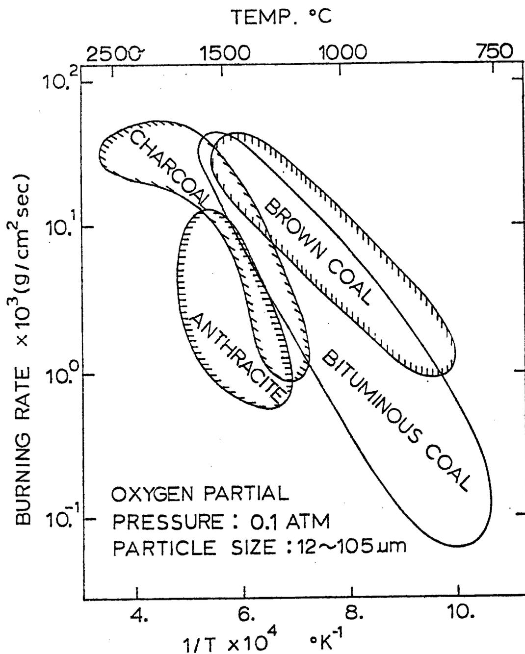
FIGURE 4. COMBUSTION RATES FOR VARIOUS COALS NEAR CHEMICAL CONTROLLING REGIME [25,26,36,37,38,20]
