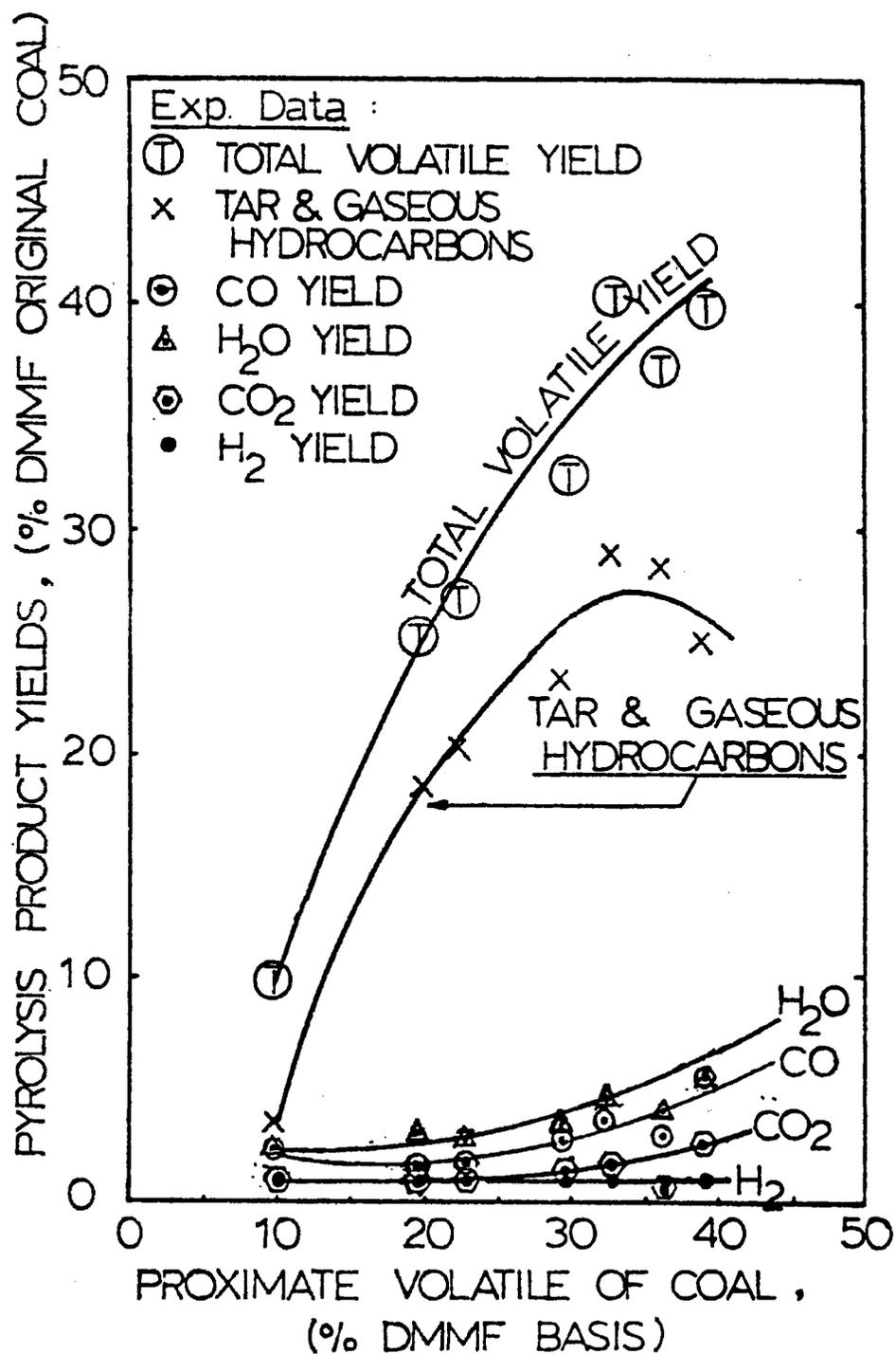
FIGURE 2. PRODUCT YIELDS OF COAL PYROLYSIS, SUMMARIZED FROM DATA OF LOISON AND CHAUVIN [8], AT  $10^3$  °C/SEC TO  $1050$  °C.
