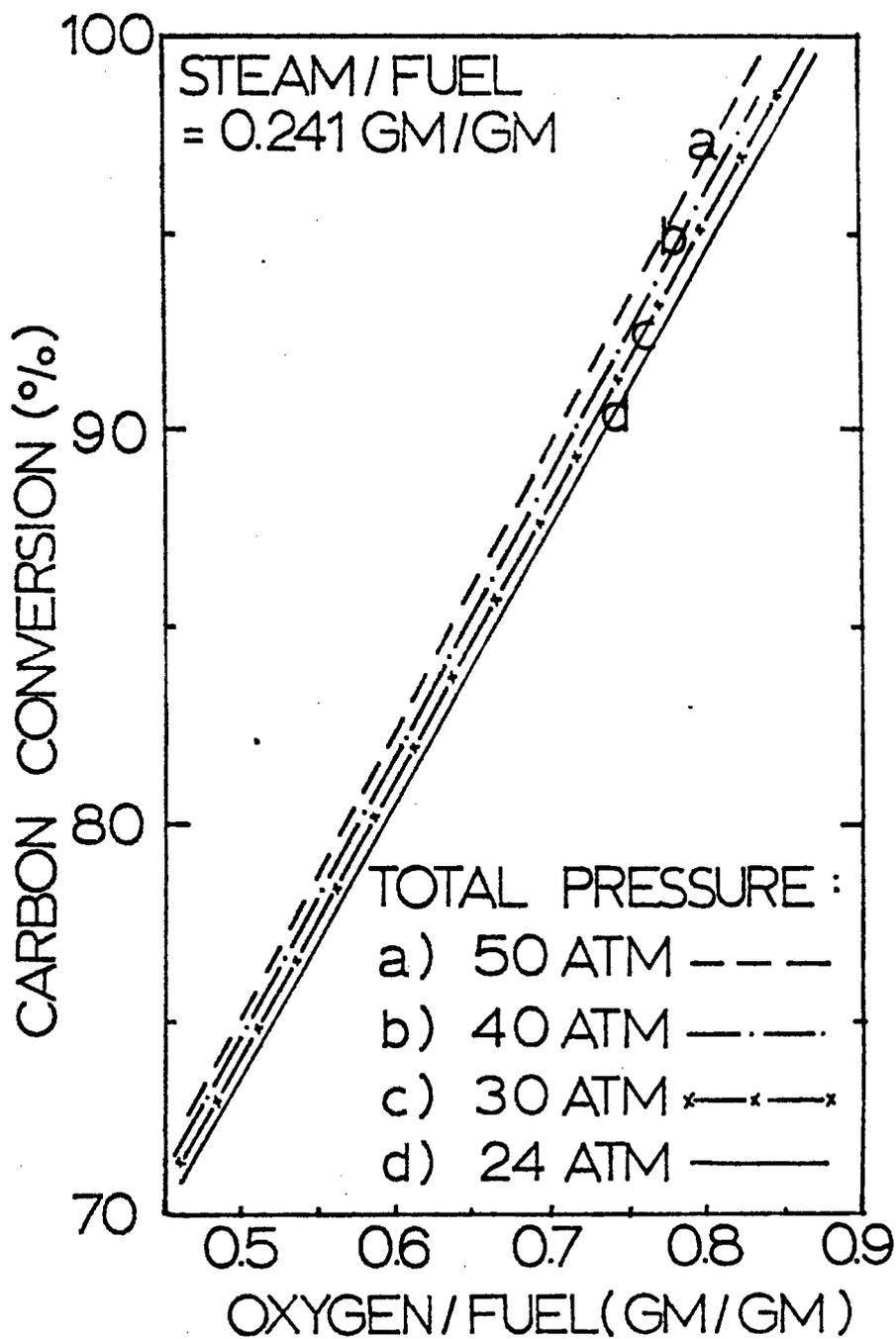
FIGURE 36 EFFECT OF TOTAL PRESSURE ON CARBON CONVERSION AT VARIOUS OXYGEN/FUEL RATIOS WITH STEAM/FUEL = 0.241 GM/GM FEEDING H-COAL RESIDUE FROM ILLINOIS NO. 6 COAL IN THE TEXACO PILOT PLANT GASIFIER.
