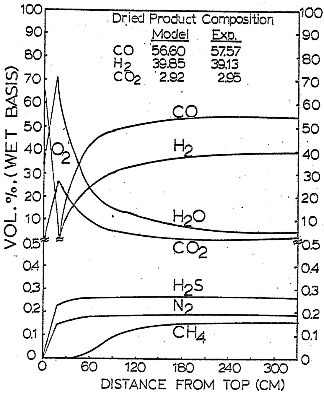
FIGURE:14(B) CALCULATED PRODUCT GAS COMPOSITION PROFILES (WET BASIS) IN TEXACO PILOT PLANT GASIFIER FOR I-1 RUN
