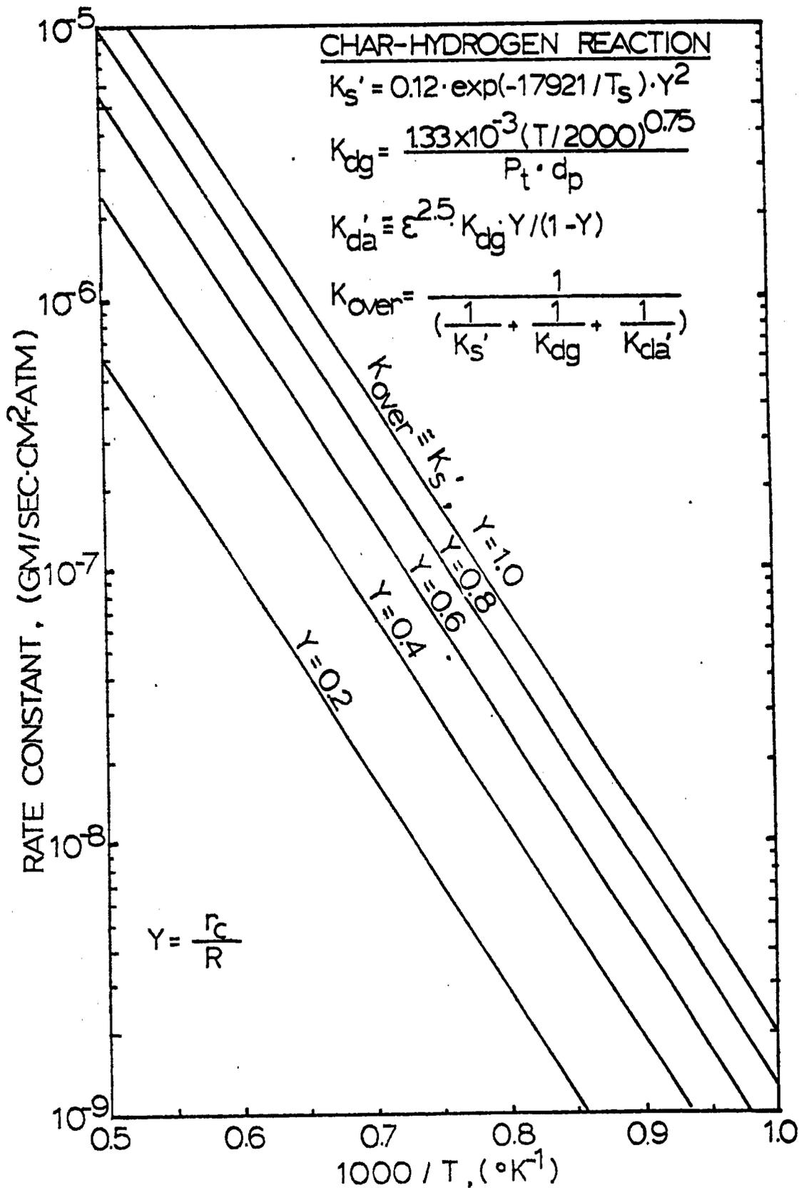
FIGURE 13. CALCULATED OVERALL CONSTANTS FOR CHAR-HYDROGEN REACTION BASED ON THE UNREACTED-CORE SHRINKING MODEL
