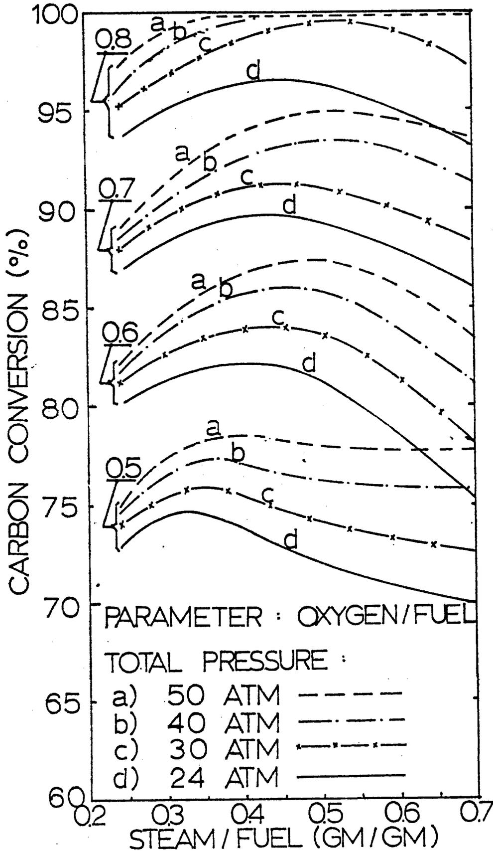
FIGURE 32. EFFECT OF TOTAL PRESSURE ON CARBON CONVERSION AT VARIOUS FEEDING RATIOS USING H-COAL RESIDUE FROM ILLINOIS NO. 6 COAL IN THE TEXACO PILOT PLANT GASIFIER
