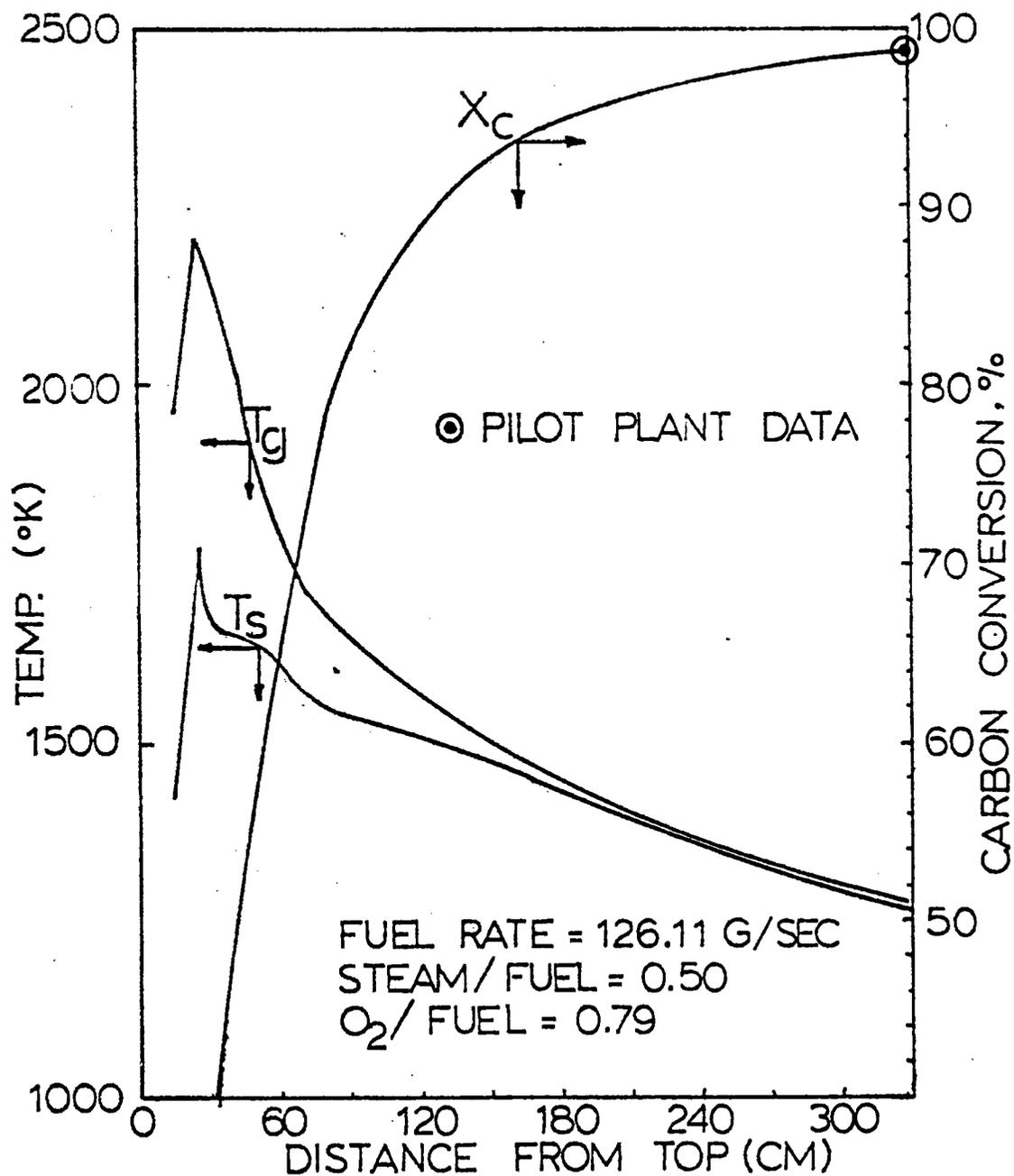
FIGURE 18(A) CALCULATED TEMPERATURE PROFILES AND CARBON CONVERSION PROFILE IN TEXACO PILOT PLANT GASIFIER USING EXXON DSP VACUUM TOWER BOTTOMS AS FEEDSTOCK.
