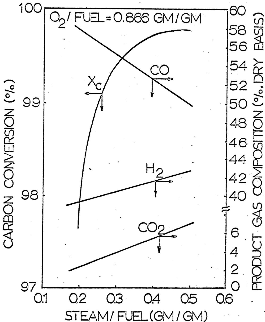
FIGURE 27 EFFECTS OF STEAM/FUEL RATIO ON THE CARBON CONVERSION AND THE MAJOR PRODUCT GAS COMPOSITION AT OXYGEN/FUEL = 0.866 GM/GM (I-1 RUN) FEEDING H-COAL RESIDUE FROM ILLINOIS NO. 6 COAL IN THE TEXACO PILOT PLANT GASIFIER
