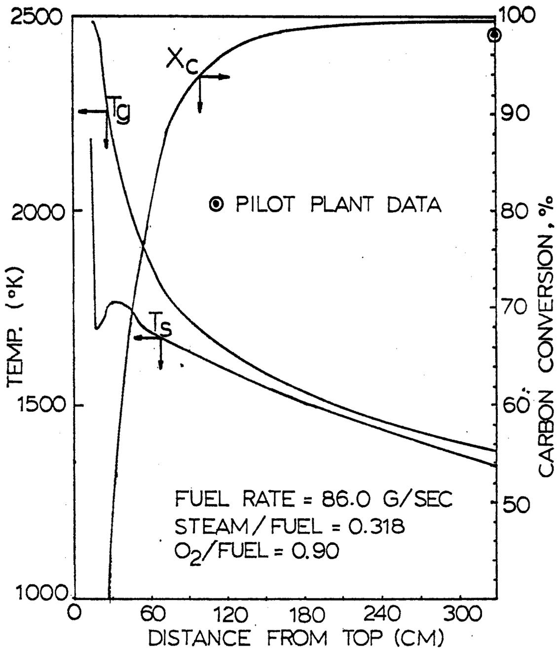
FIGURE 16(A) CALCULATED TEMPERATURE PROFILES AND CARBON CONVERSION PROFILE IN TEXACO PILOT PLANT GASIFIER FOR W-1 RUN
