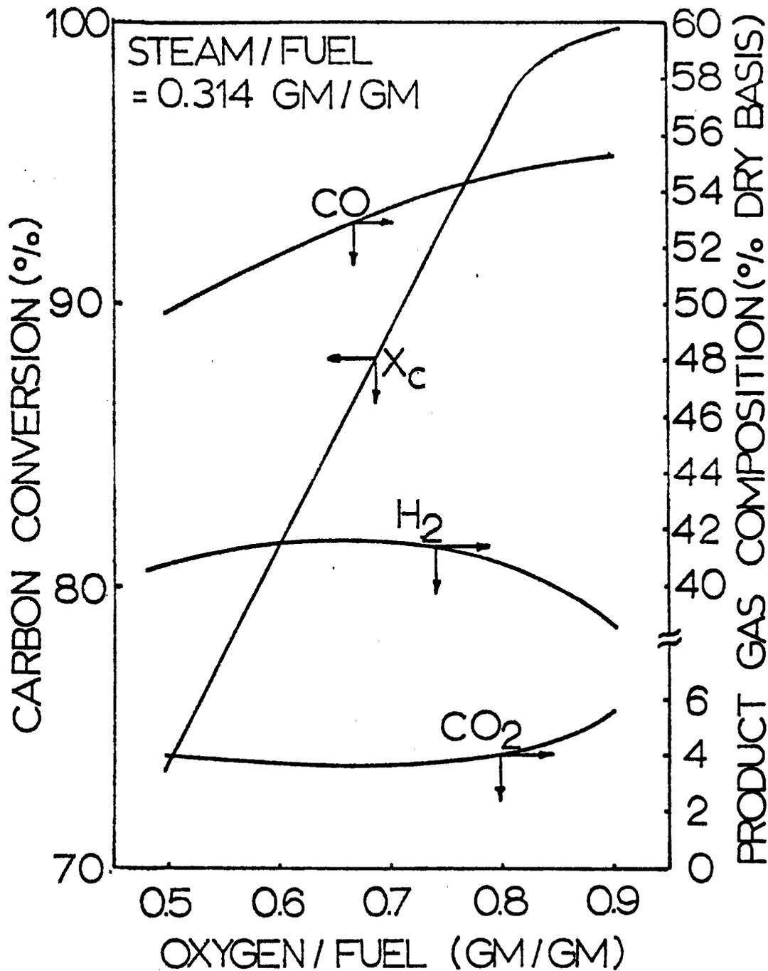
FIGURE 24 EFFECTS OF OXYGEN/FUEL RATIO ON THE CARBON CONVERSION AND THE MAJOR PRODUCT GAS COMPOSITION AT STEAM/FUEL = 0.314 GM/GM (I-2 RUN) FEEDING H-COAL RESIDUE FROM ILLINOIS NO. 6 COAL IN THE TEXACO PILOT PLANT GASIFIER.
