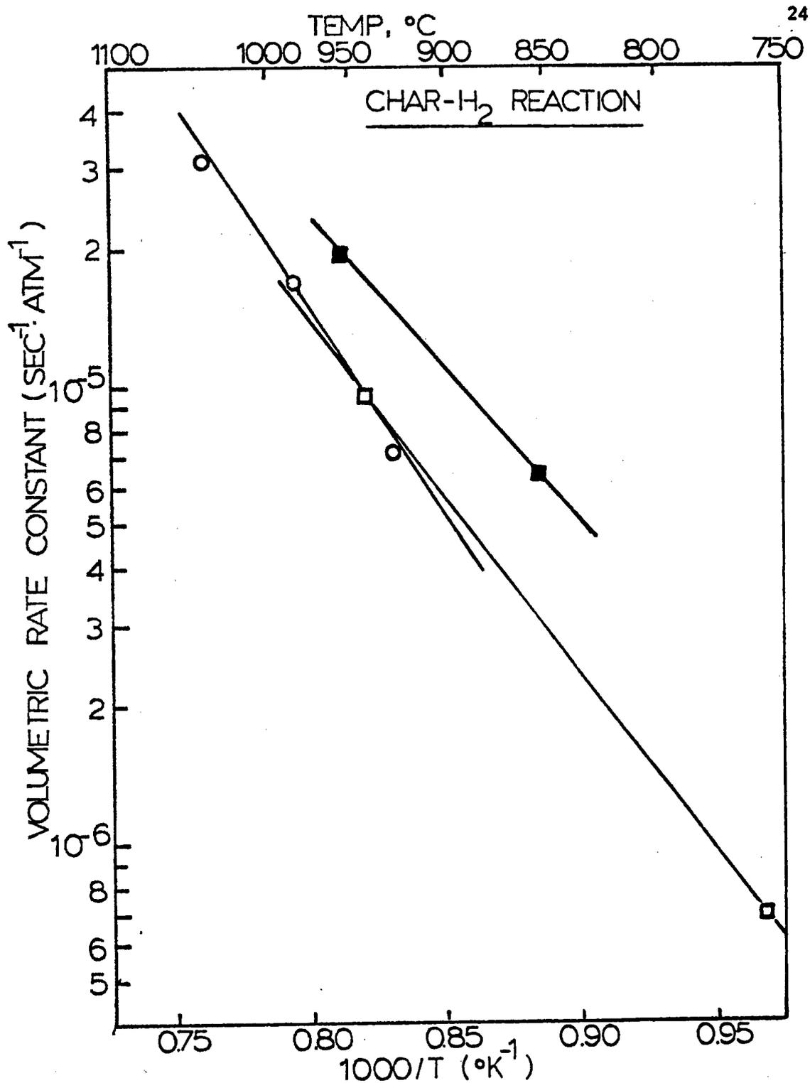
FIGURE 7. ARRHENIUS PLOTS FOR CHAR HYDROGASIFICATION
