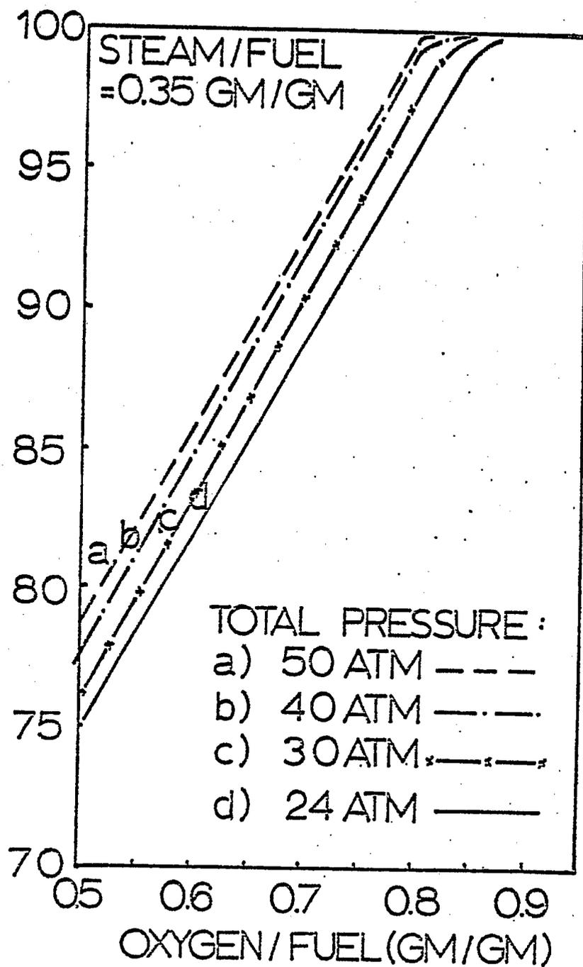
FIGURE 35 EFFECT OF TOTAL PRESSURE ON CARBON CONVERSION AT VARIOUS OXYGEN/FUEL RATIOS WITH STEAM/FUEL = 0.35 GM/GM FEEDING H-COAL RESIDUE FROM ILLINOIS NO. 6 COAL IN THE TEXACO PILOT PLANT GASIFIER.
