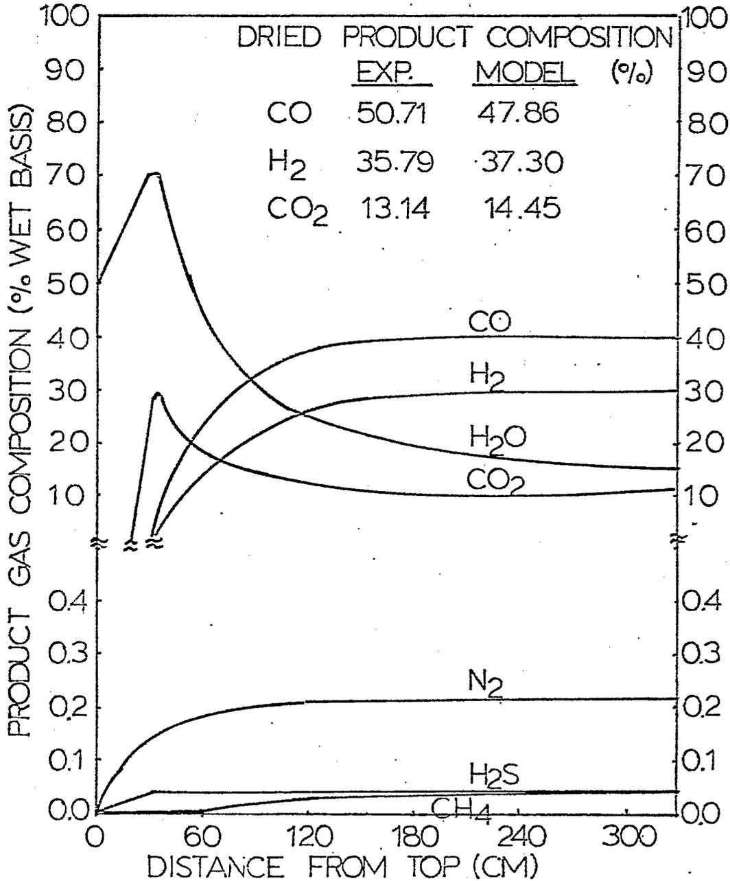
FIGURE 19(B) CALCULATED PRODUCT GAS COMPOSITION PROFILES IN TEXACO'S PILOT PLANT GASIFIER USING WESTERN COAL AS FEEDSTOCK IN COAL-WATER SLURRY RUNS.
