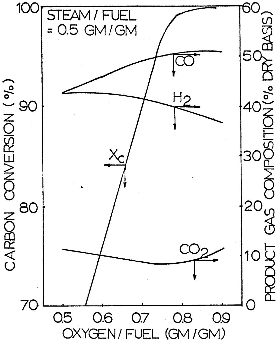
FIGURE 26 EFFECTS OF OXYGEN/FUEL RATIO ON THE CARBON CONVERSION AND THE MAJOR PRODUCT GAS COMPOSITION AT STEAM/FUEL = 0.5 GM/GM FEEDING COAL RESIDUES FROM EXXON DSP VACCUM TOWER BOTTOMS IN THE TEXACO PILOT PLANT GASIFIER
