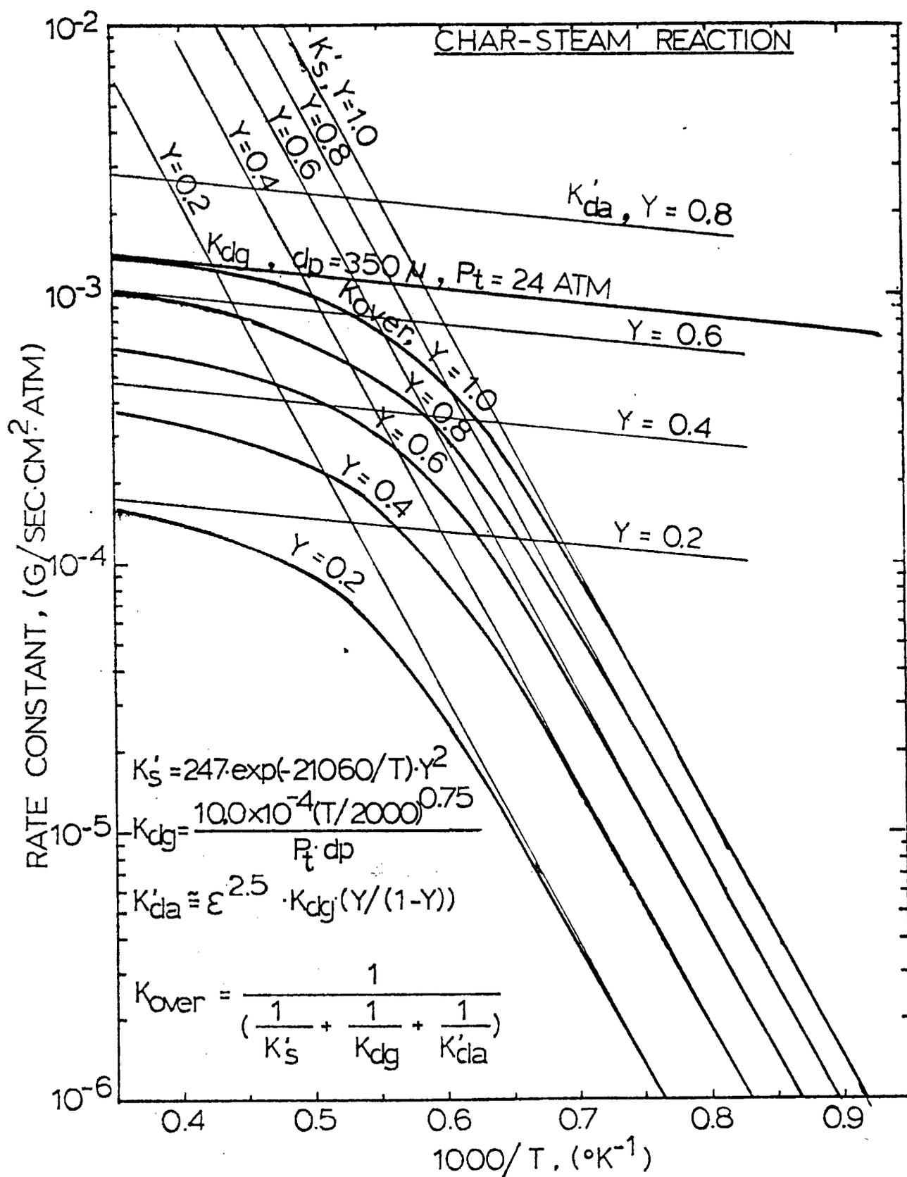
FIGURE 11. CALCULATED OVERALL CONSTANTS FOR CHAR-STEAM REACTION BASED ON THE UNREACTED-CORE SHRINKING MODEL
