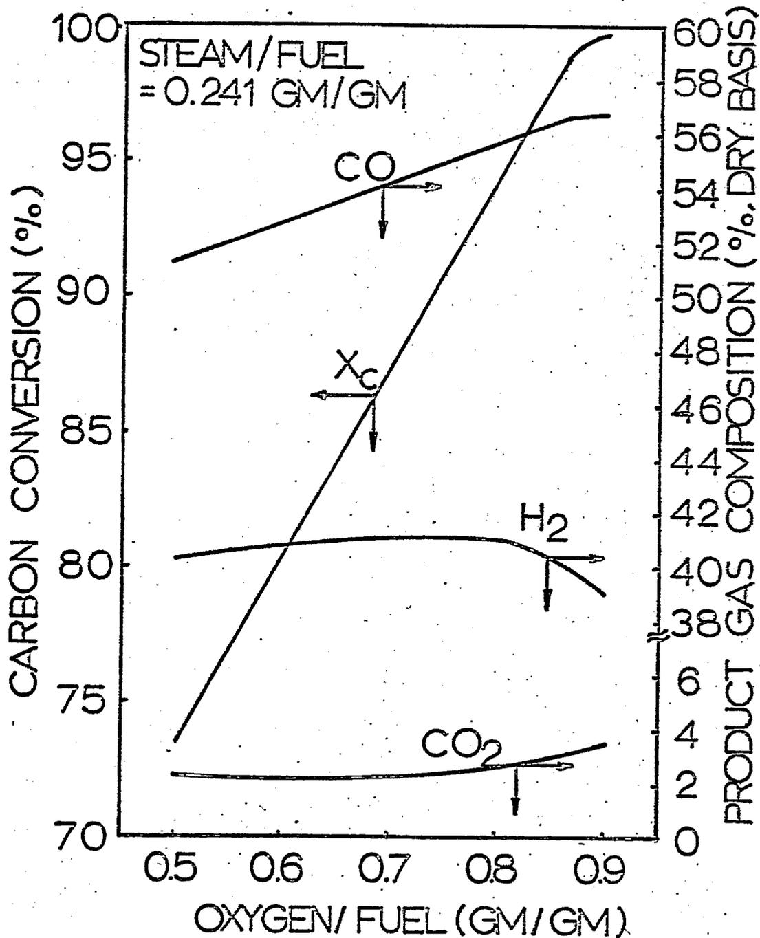
FIGURE 23. EFFECTS OF OXYGEN/FUEL RATIO ON THE CARBON CONVERSION AND THE MAJOR PRODUCT GAS COMPOSITION AT STEAM/FUEL = 0.241 GM/GM (I-1 RUN) FEEDING H-COAL RESIDUE FROM ILLINOIS NO. 6 COAL IN THE TEXACO PILOT PLANT GASIFIER
