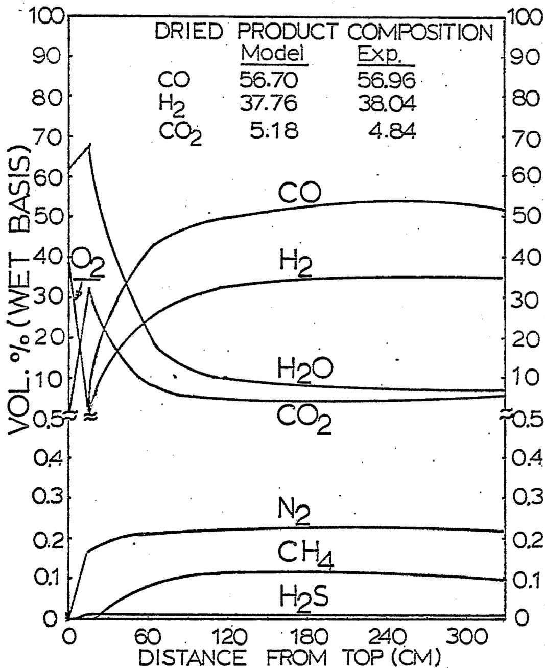
FIGURE 16(B) CALCULATED PRODUCT GAS COMPOSITION PROFILES (WET BASIS) IN TEXACO PILOT PLANT GASIFIER FOR W-1 RUN
