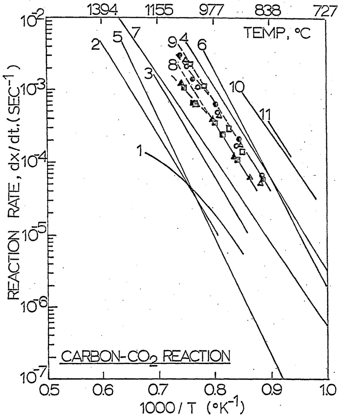
FIGURE 6. ARRHENIUS PLOTS FOR THE REACTION BETWEEN CO AND VARIOUS FORMS OF CARBON (SEE THE LEGEND IN TABLE III) [19]
