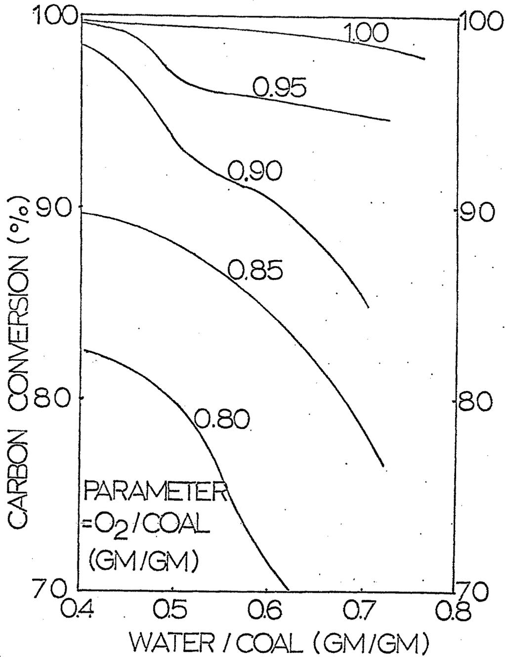
FIGURE 31 EFFECT OF WATER/COAL RATIO ON CARBON CONVERSION AT VARIOUS OXYGEN/COAL RATIO FEEDING WESTERN COAL TEXACO'S PILOT PLANT GASIFIER IN COAL-WATER SLURRY RUNS.
