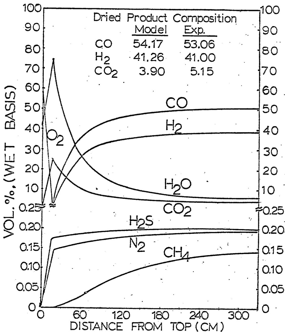
FIGURE 15(B) CALCULATED PRODUCT GAS COMPOSITION PROFILES (WET BASIS) IN TEXACO PILOT PLANT GASIFIER FOR I-2 RUN
