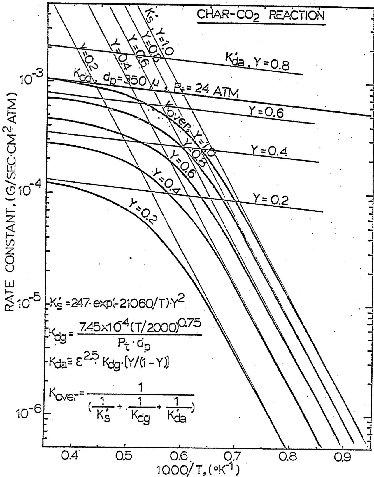
FIGURE 12. CALCULATED OVERALL CONSTANTS FOR CHAR-CARBON DIOXIDE REACTION BASED ON THE UNREACTED-CORE SHRINKING MODEL
