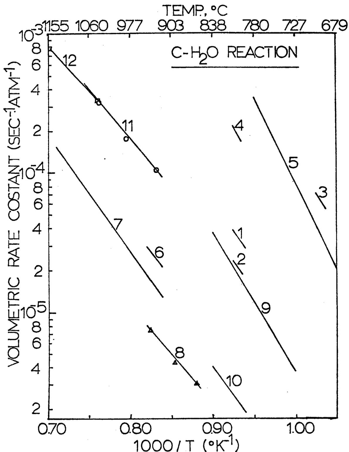
FIGURE 5. ARRHENIUS PLOT FOR THE REACTION OF STEAM WITH VARIOUS FORMS OF CARBON (SEE THE LEGEND IN TABLE II) [19]
