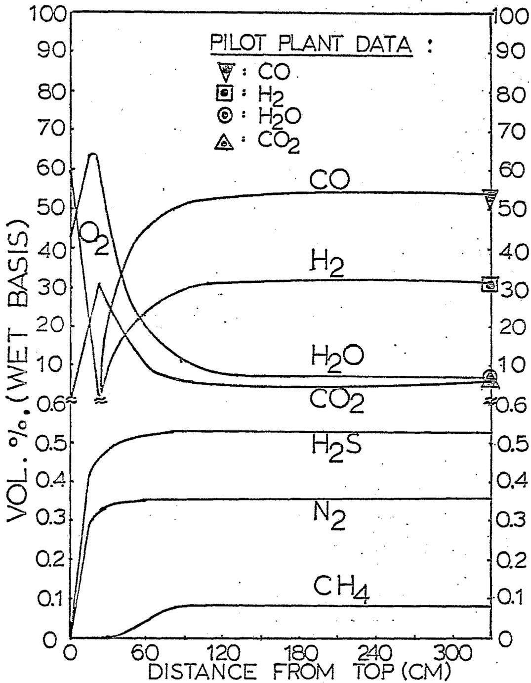
FIGURE 17(B) CALCULATED PRODUCT GAS COMPOSITION PROFILES (WET BASIS) IN TEXACO PILOT PLANT GASIFIER USING SRC II VACUUM FLASH DRUM BOTTOMS AS FEEDSTOCK
