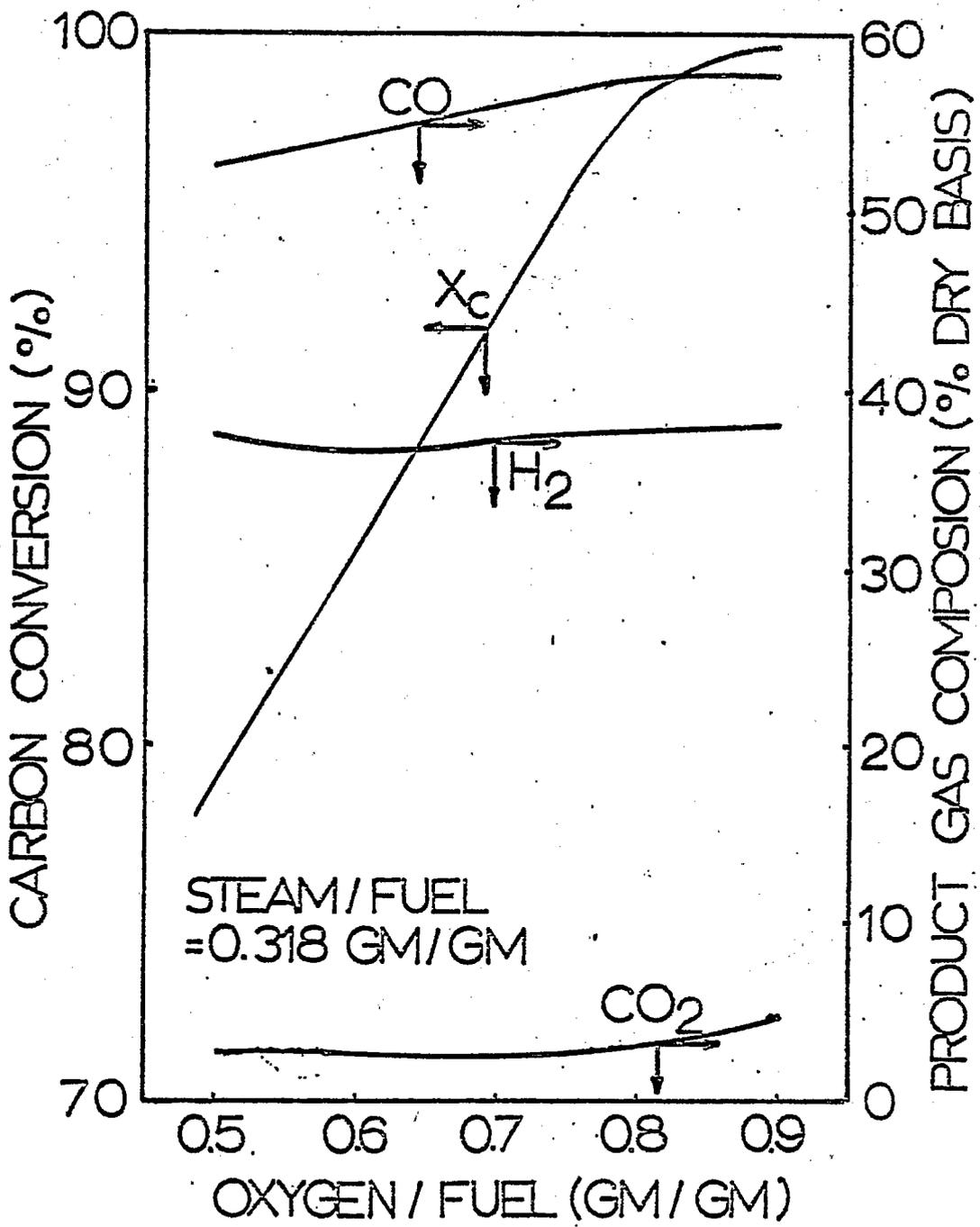
FIGURE 25 EFFECTS OF OXYGEN/FUEL RATIO ON THE CARBON CONVERSION AND THE MAJOR PRODUCT GAS COMPOSITION AT STEAM/FUEL = 0.318 GM/GM (W-1 RUN) FEEDING H-COAL RESIDUE FROM WYODAK COAL IN THE TEXACO PILOT PLANT GASIFIER
