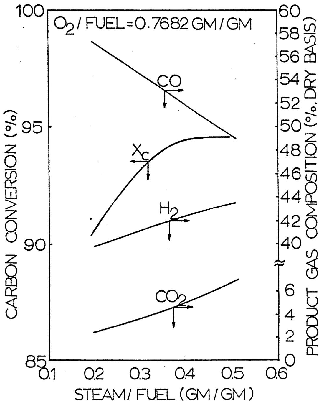
FIGURE 28 EFFECTS OF STEAM/FUEL RATIO ON THE CARBON CONVERSION AND THE MAJOR PRODUCT GAS COMPOSITION AT OXYGEN/FUEL = 0.7682 GM/GM (I-2 RUN) FEEDING H-COAL RESIDUE FROM ILLINOIS NO. 6 COAL IN THE TEXACO PILOT PLANT GASIFIER
