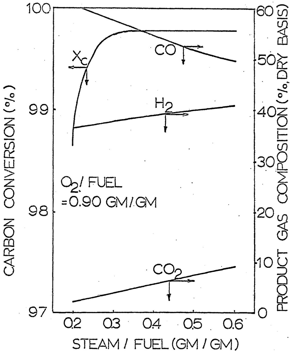
FIGURE 29 EFFECTS OF STEAM/FUEL RATIO ON THE CARBON CONVERSION AND THE MAJOR PRODUCT COMPOSITION AT OXYGEN/FUEL = 0.90 GM/GM (W-1 RUN) FEEDING H-COAL RESIDUE FROM WYODAK COAL IN THE TEXACO PILOT PLANT GASIFIER
