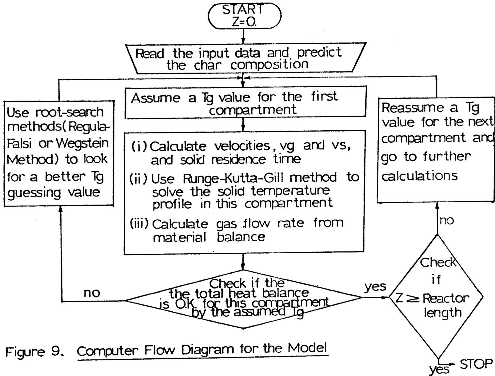
Figure 9. Computer Flow Diagram for the Model
