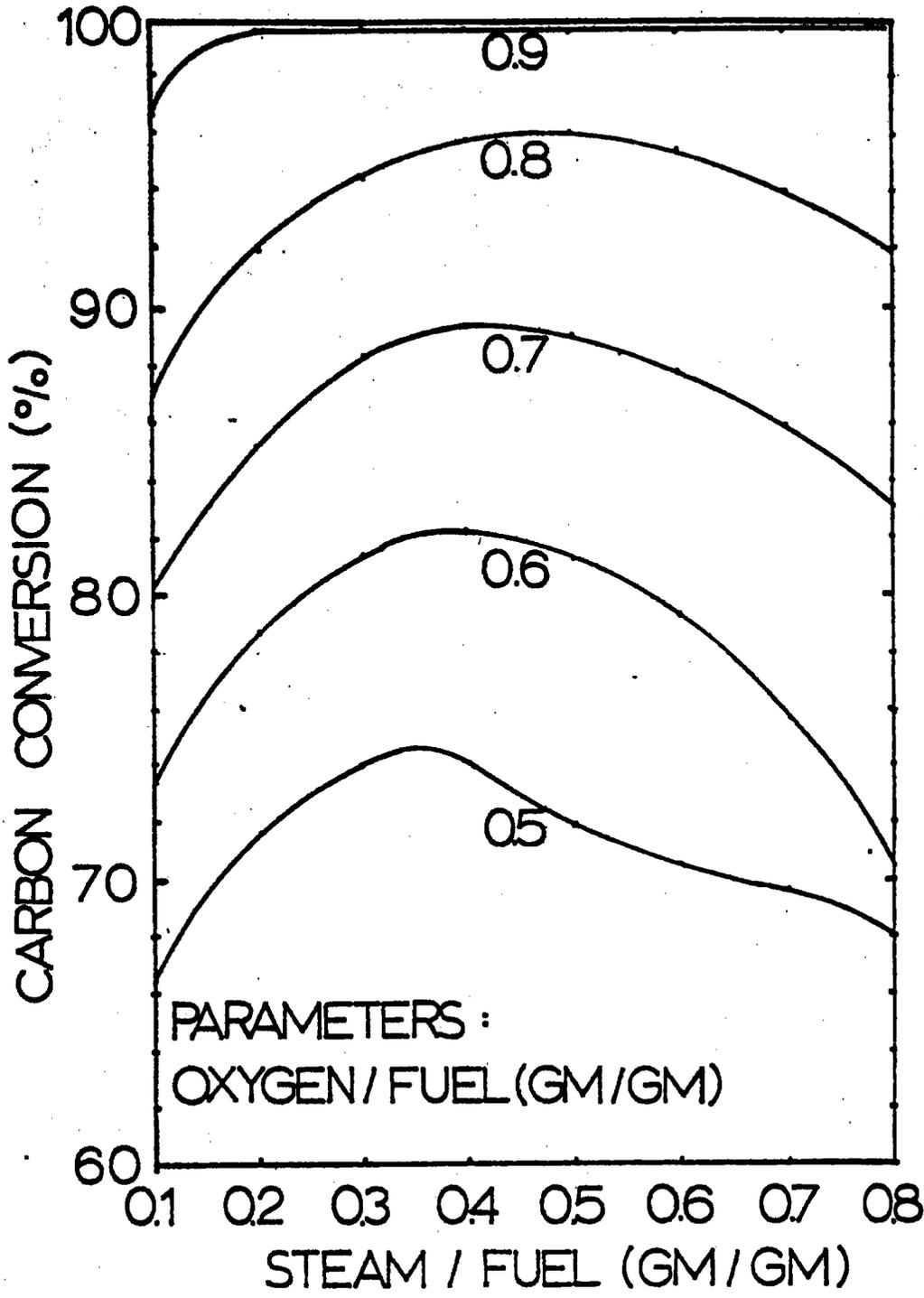
FIGURE 22 EFFECT OF STEAM/FUEL RATIO ON THE CARBON CONVERSION AT VARIOUS OXYGEN/FUEL RATIOS FEEDING THE H-COAL RESIDUE FROM ILLINOIS NO. 6 COAL IN THE TEXACO PILOT PLANT GASIFIER
