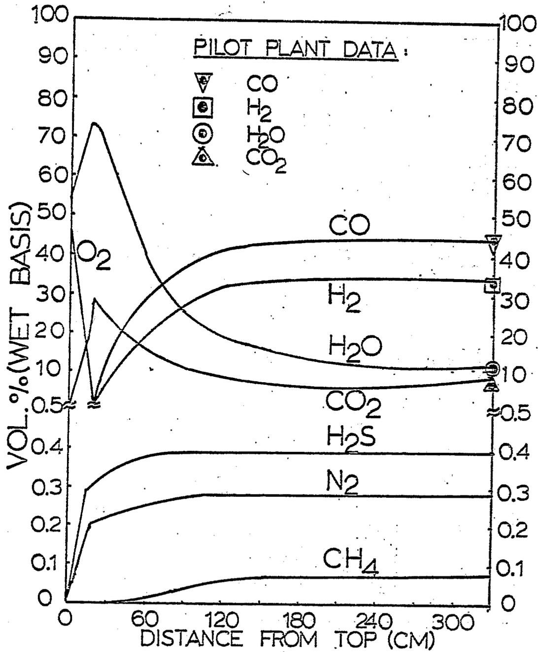
FIGURE 18(B) CALCULATED PRODUCT GAS COMPOSITION PROFILES (WET BASIS) IN TEXACO PILOT PLANT GASIFIER USING EXXON DSP VACUUM TOWER BOTTOMS AS FEEDSTOCK
