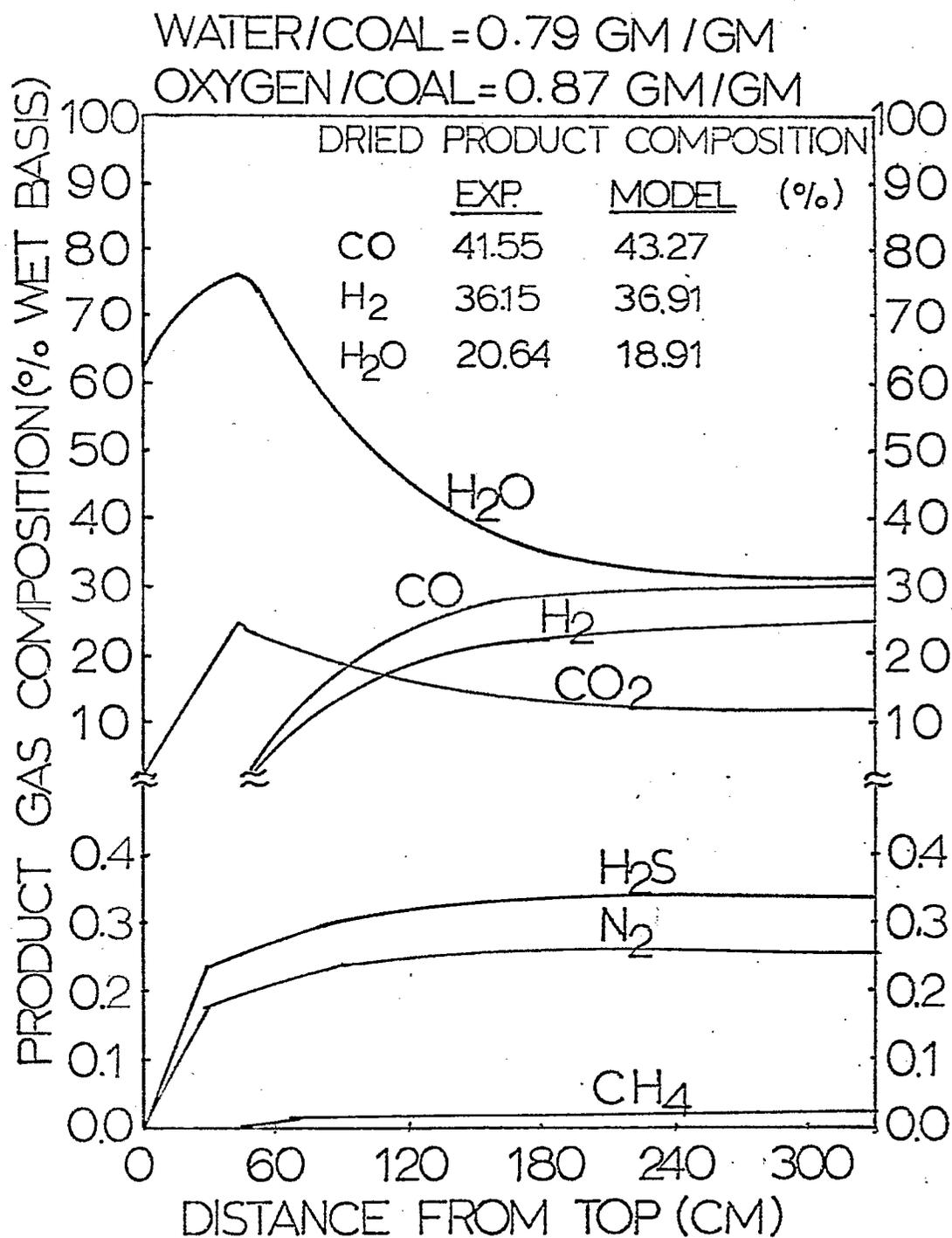
FIGURE 20(B) CALCULATED PRODUCT GAS COMPOSITION PROFILES IN TEXACO'S PILOT PLANT GASIFIER USING EASTERN COAL AS FEEDSTOCK IN COAL-WATER SLURRY RUNS
