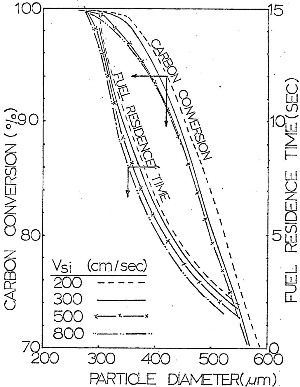
FIGURE 37 EFFECT OF FUEL PARTICLE SIZE ON THE FUEL RESIDENCE TIME AND THE CARBON CONVERSION AT VARIOUS INITIAL SOLID VELOCITIES FEEDING ILLINOIS NO. 6 COAL LIQUEFACTION RESIDUE IN TEXACO PILOT PLANT ENTRAINED GASIFIER.
