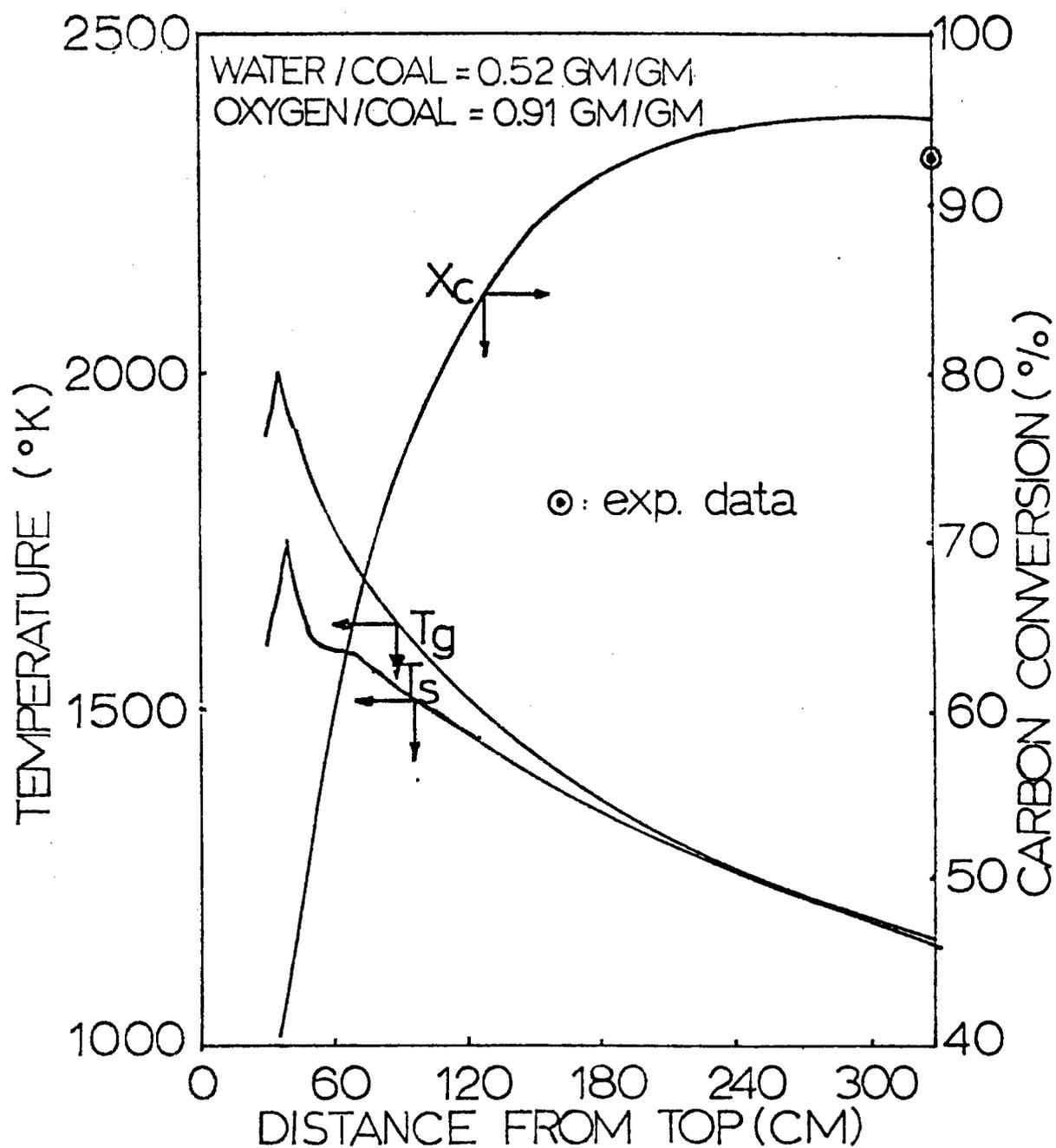
FIGURE 19(A) CALCULATED TEMPERATURE AND CARBON CONVERSION PROFILES IN TEXACO'S PILOT PLANT GASIFIER USING WESTERN COAL AS FEEDSTOCK IN COAL-WATER SLURRY RUNS.
