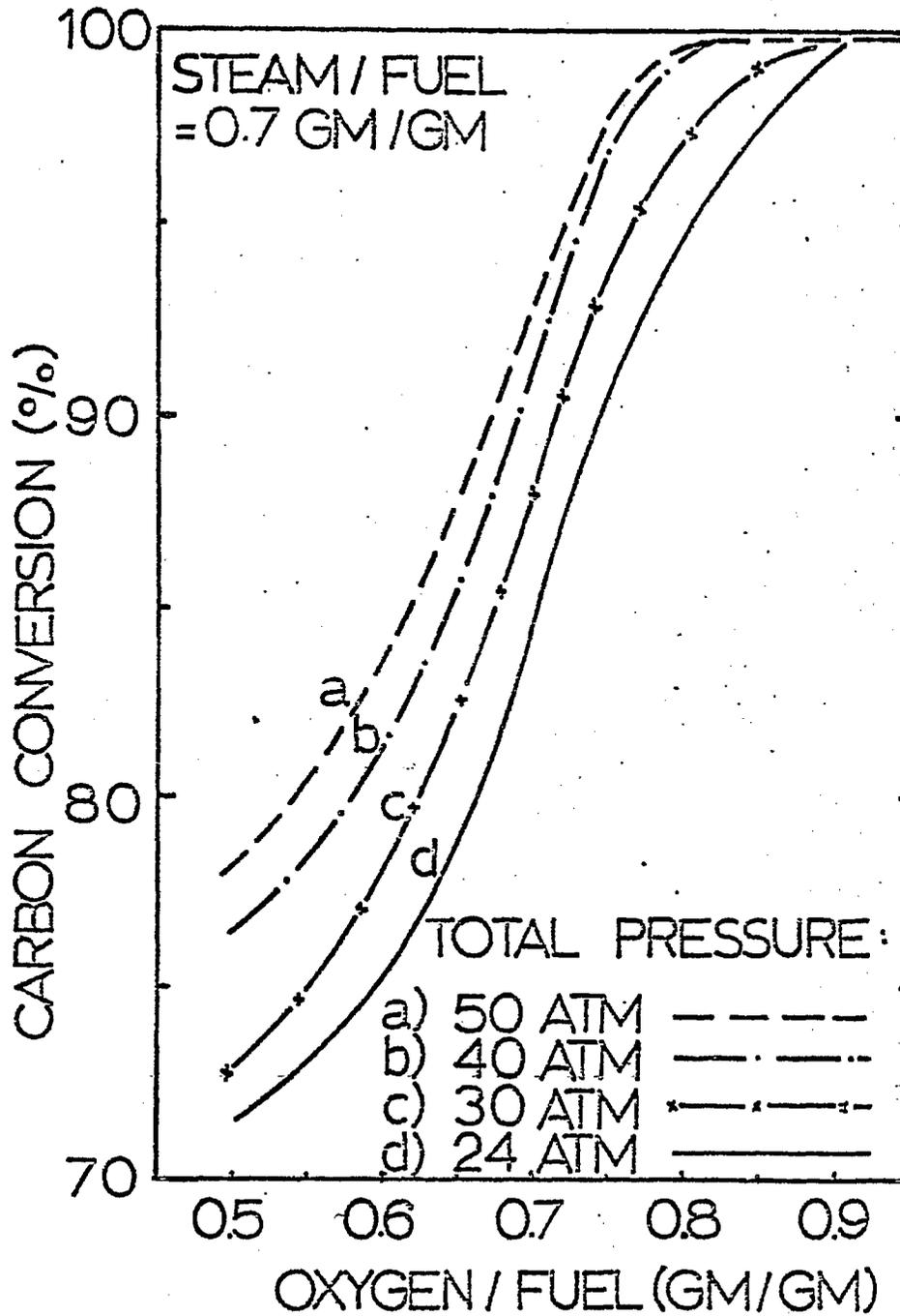
FIGURE 33 EFFECT OF TOTAL PRESSURE ON CARBON CONVERSION AT VARIOUS OXYGEN/FUEL RATIOS WITH STEAM/FUEL = 0.7 GM/GM FEEDING H-COAL RESIDUE FROM ILLINOIS NO. 6 COAL IN THE TEXACO PILOT PLANT GASIFIER.
