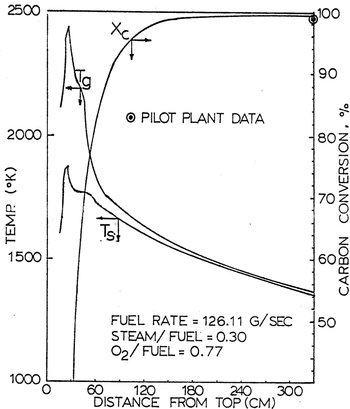
FIGURE 17(A) CALCULATED TEMPERATURE PROFILES AND CARBON CONVERSION PROFILE IN TEXACO PILOT PLANT GASIFIER USING SRC II VACUUM FLASH DRUM BOTTOMS AS FEEDSTOCK
