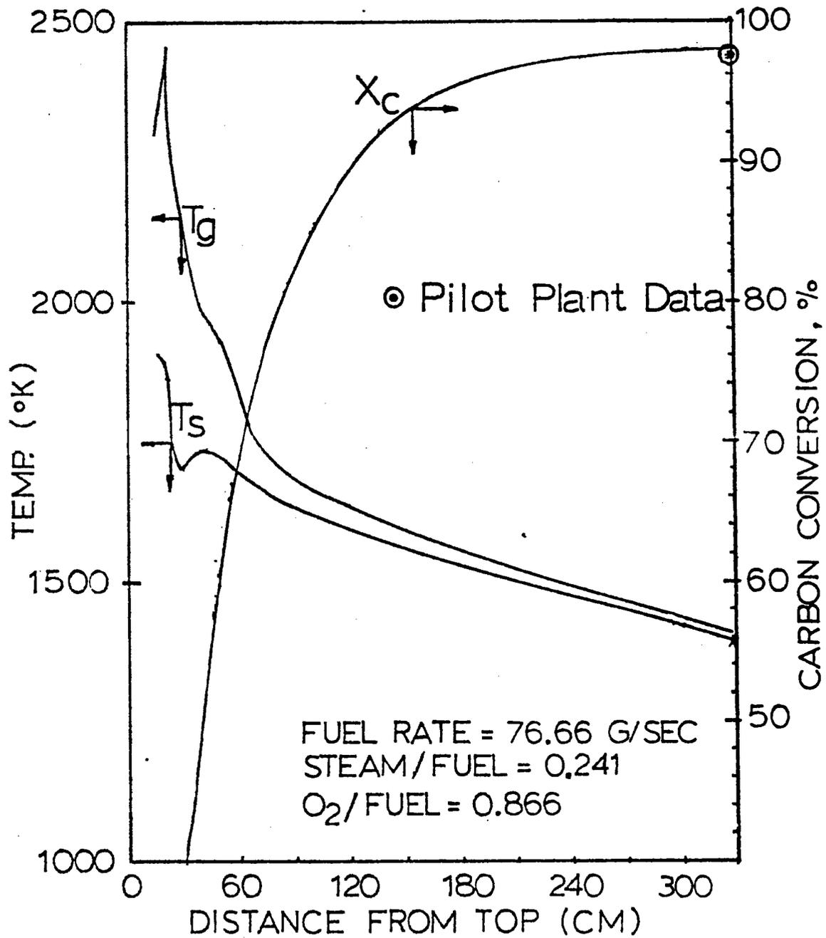
FIGURE 14(A) CALCULATED TEMPERATURE PROFILES AND CARBON CONVERSION PROFILE IN TEXACO PILOT PLANT GASIFIER FOR I-1 RUN.
