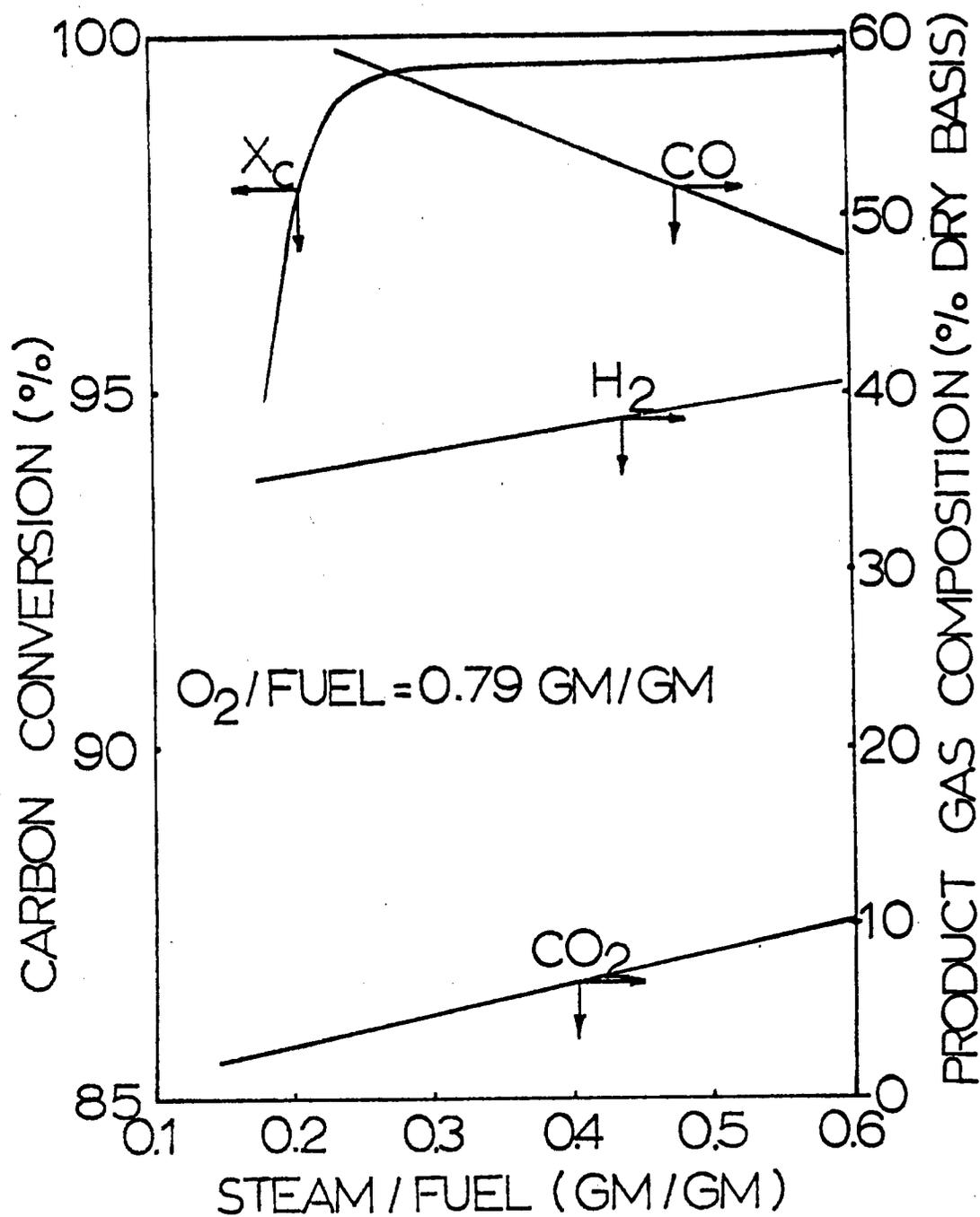
FIGURE 30 EFFECTS OF STEAM/FUEL RATIO ON THE CARBON CONVERSION AND THE MAJOR PRODUCT COMPOSITION AT OXYGEN/FUEL = 0.79 GM/GM FEEDING COAL RESIDUES FROM EXXON DSP VACCUM TOWER BOTTOMS IN THE TEXACO PILOT PLANT GASIFIER
