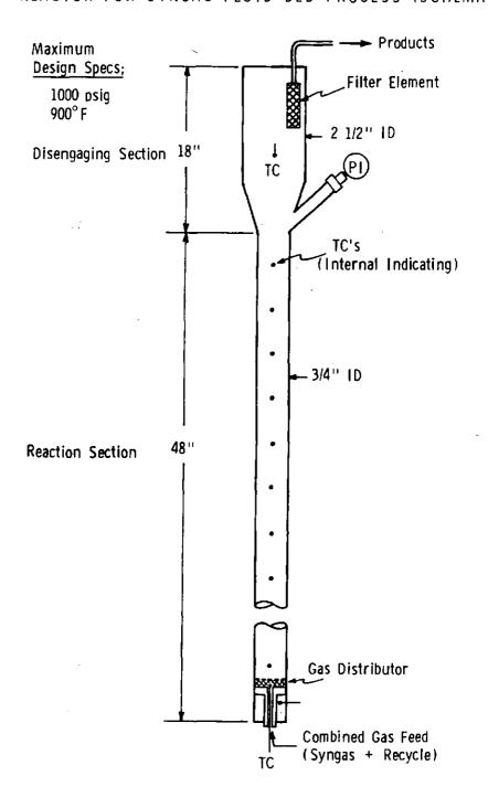
with 18 small orifices. The gas mixture reacted in the fluidized catalyst bed, passed up the reactor to the disengaging zone where it separated from the catalyst, and exited through two, parallel, stainless steel, porous filters where any entrained catalyst dust was removed.
