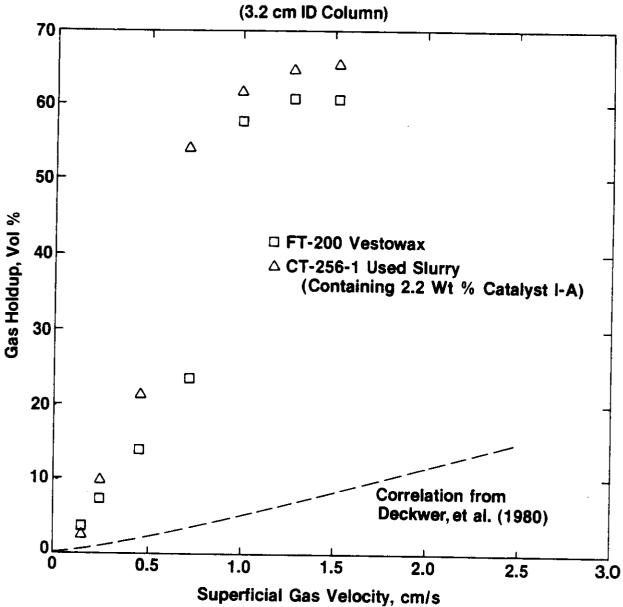
very small gas bubbles distributed throughout the liquid and was topped by a layer of foam. The liquid was clean and it was possible to see through the column. At low superficial gas velocities ( $u_g < 0.72$  cm/s) the foaming was minimal and there was a discernible boundary between the foam and non-foam liquid layers. In this regime the gas holdup appeared to vary linearly with the superficial gas velocity according to the following equation:
