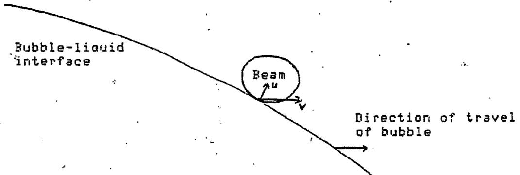
There is a component of bubble velocity which merely moves the bubble surface parallel to the beam 'surface', and thus plays no part in cutting off the beam. Only the component of the bubble velocity perpendicular to the bubble surface at the point of intersection with the beam plays an effective role.
