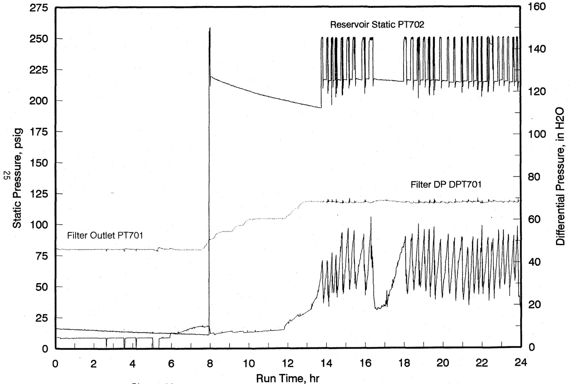
Figure 14. Hot-gas filter vessel pressure profile for 10/05/97.
