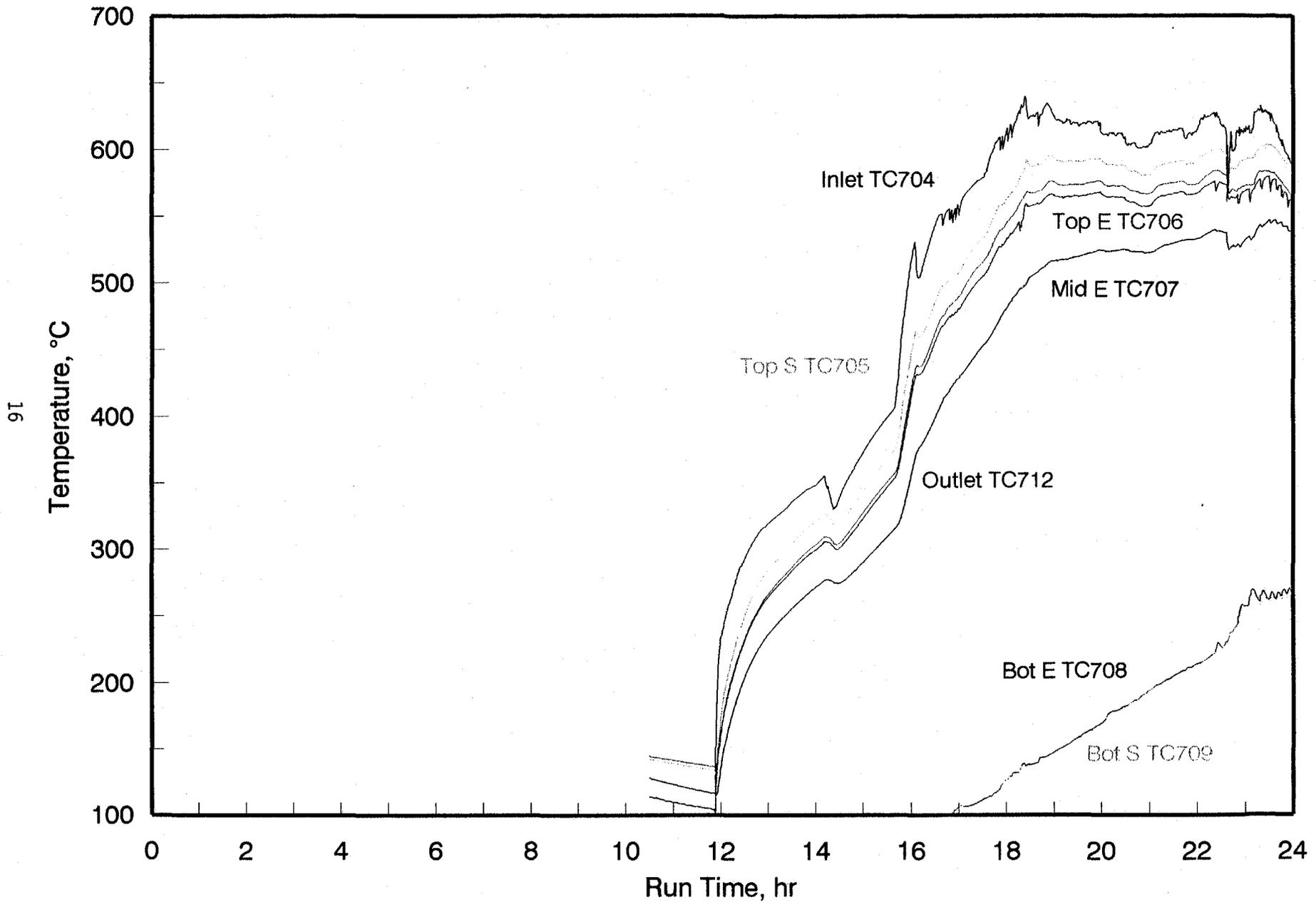
Figure 5. Hot-gas filter vessel temperature profile for 07/08/97.
