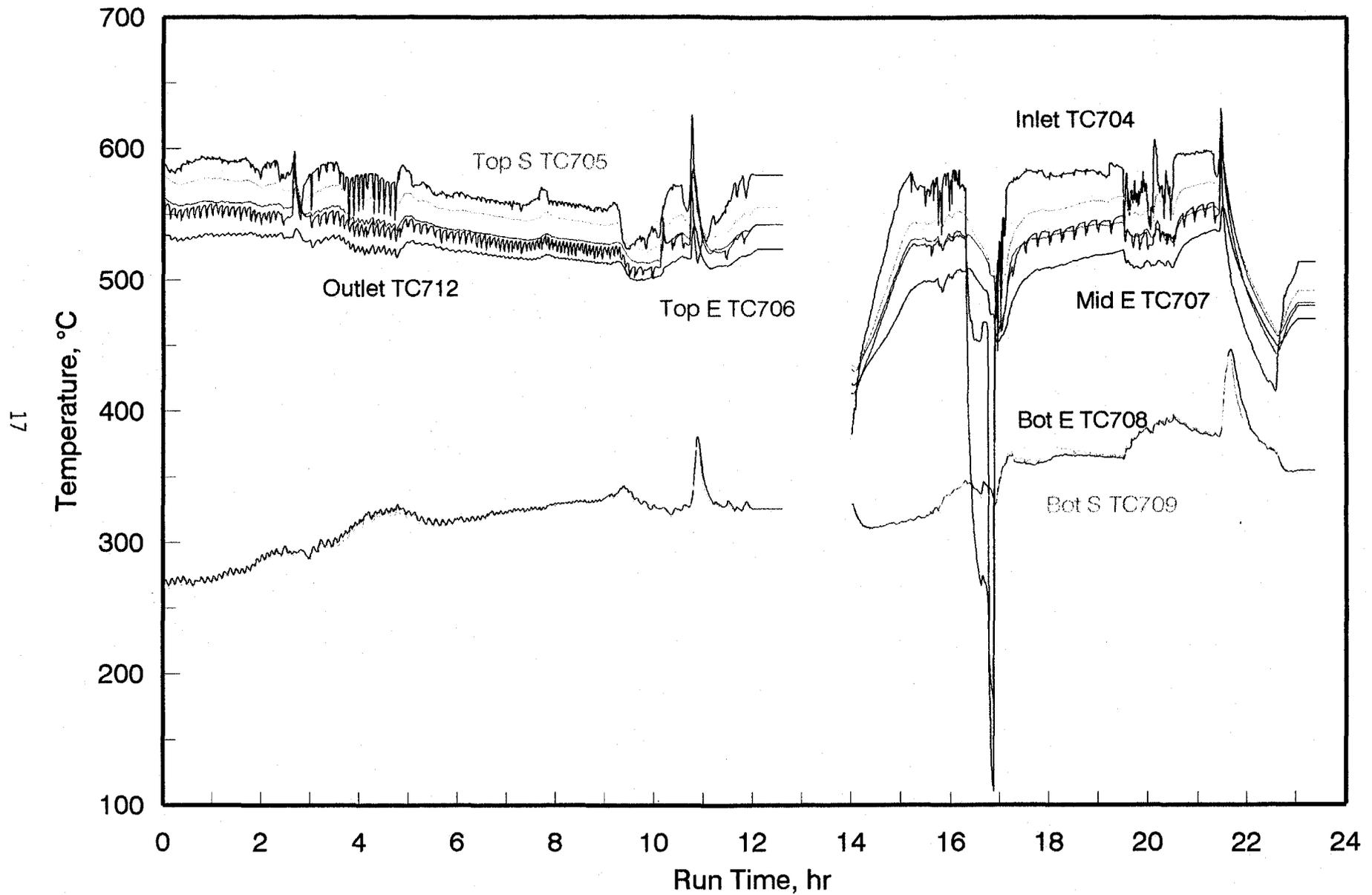
Figure 6. Hot-gas filter vessel temperature profile for 07/09/97.
