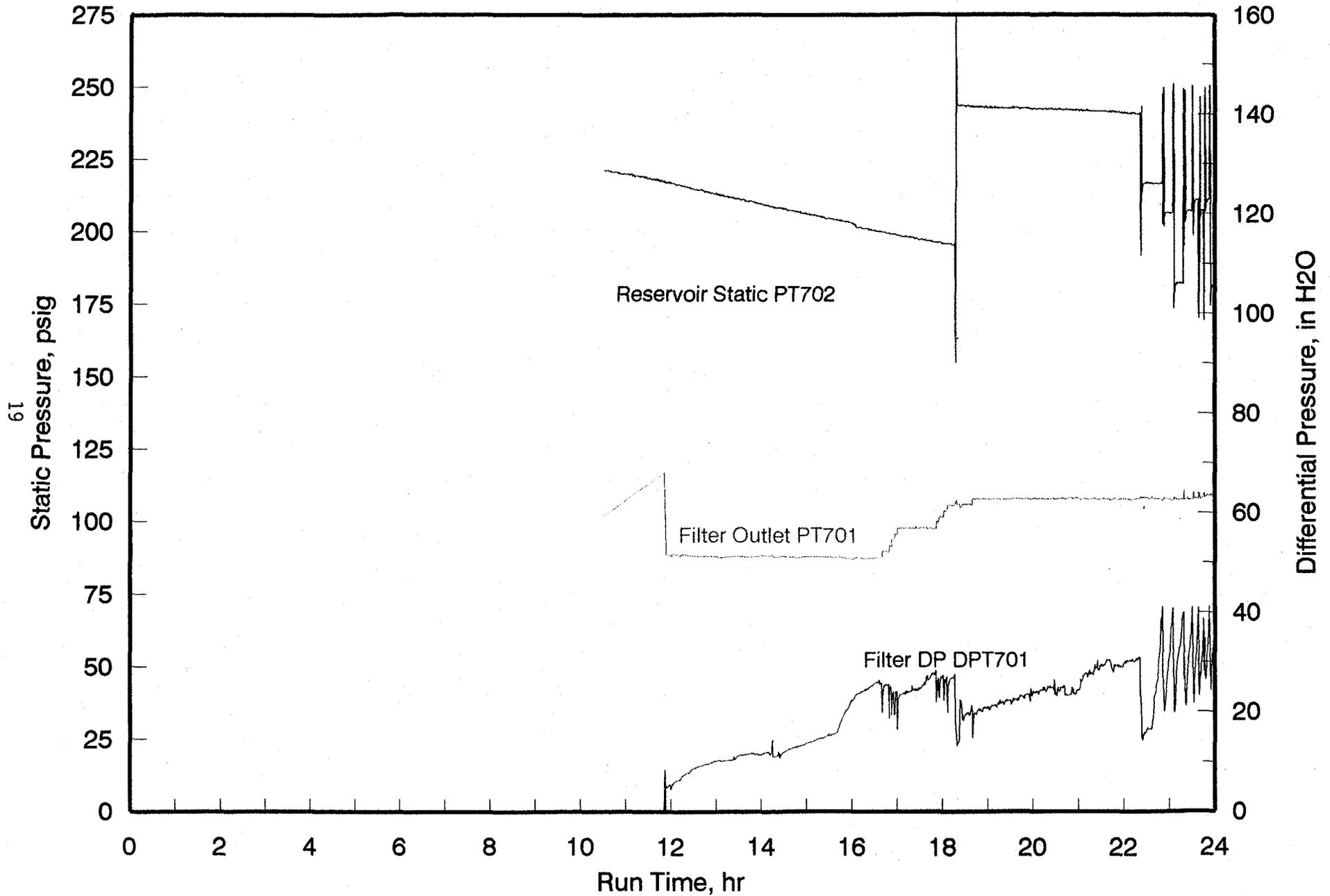
Figure. 8 Hot-gas filter vessel pressure profile for 07/08/97.
