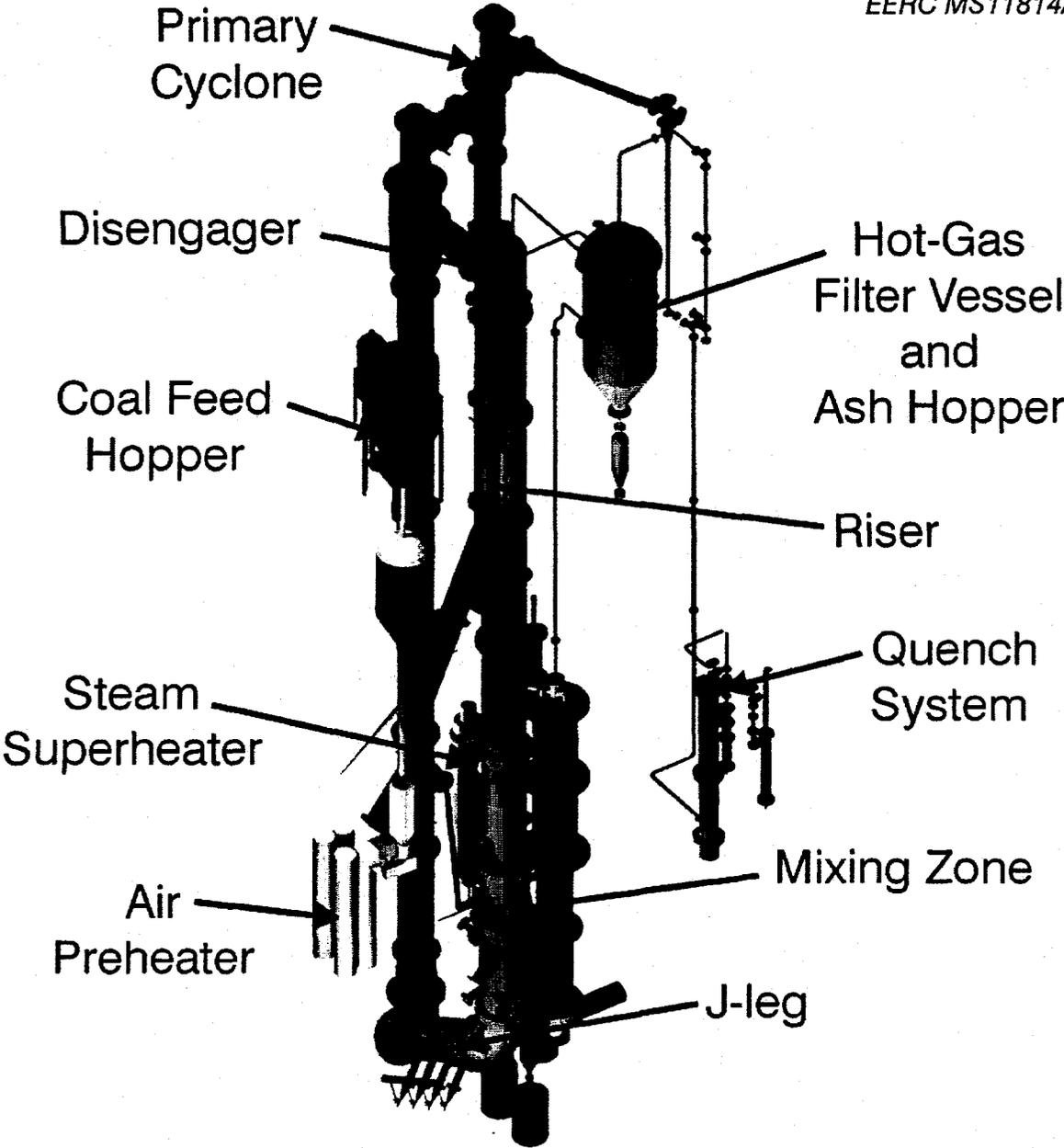
Figure 1. TRDU and hot-gas vessel in the EERC gasification tower.
