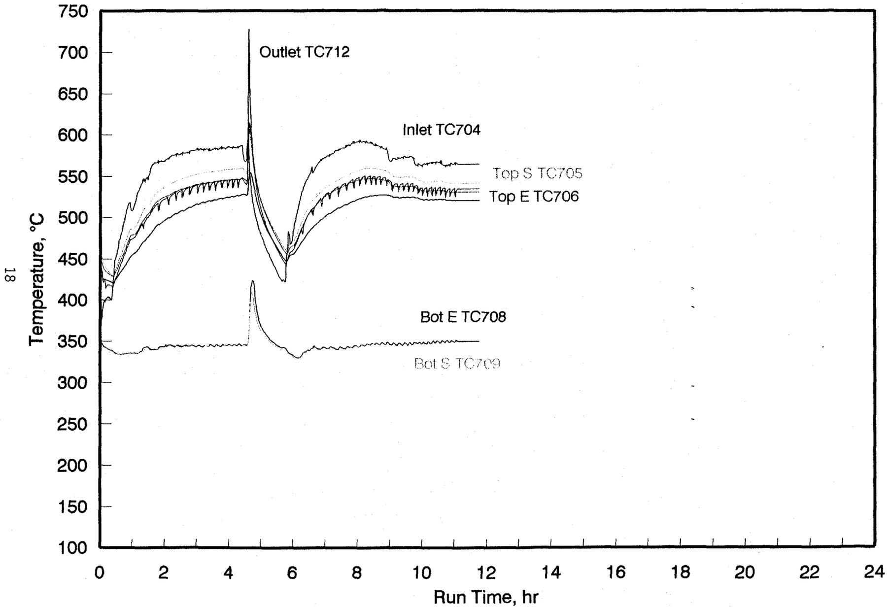
Figure 7. Hot-gas filter vessel temperature profile for 07/10/97.
