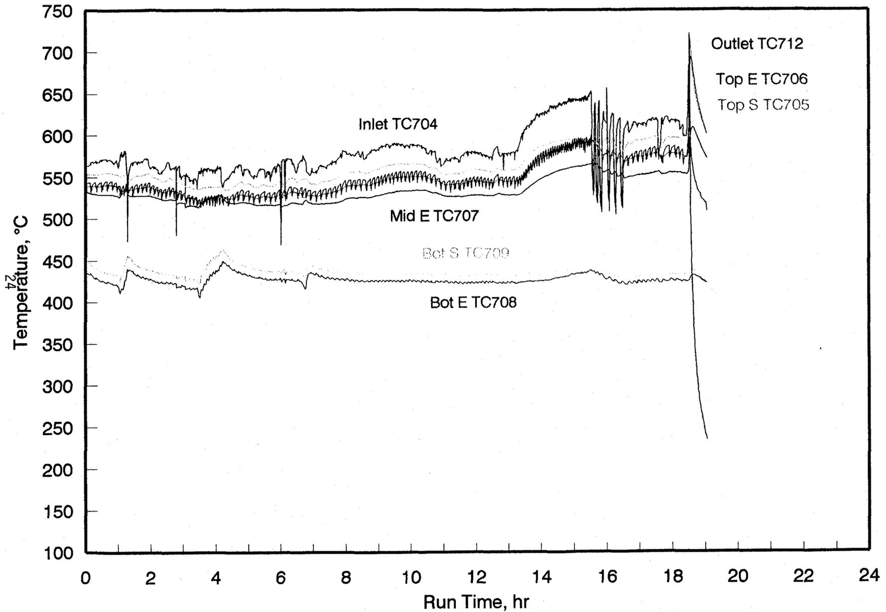
Figure 13. Hot-gas filter vessel temperature profile for 10/07/97.
