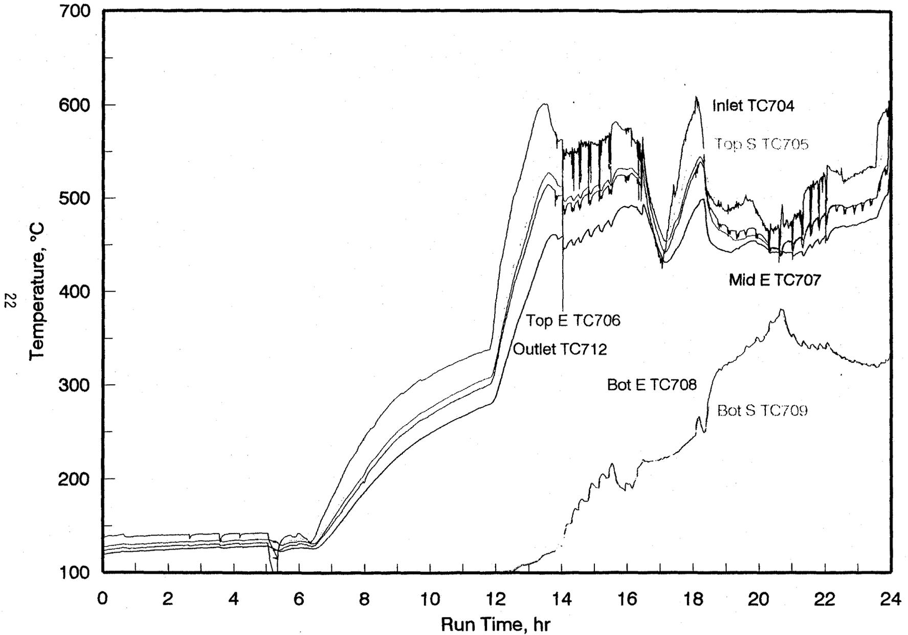
Figure 11. Hot-gas filter vessel temperature profile for 10/05/97.
