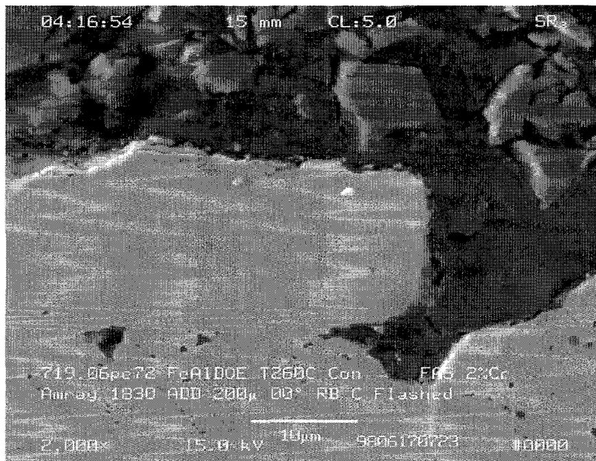
Figure 24: Cross-section of FAS control sample. Preoxidized for seven hours at 800°C. Alumina oxide layer can not be seen.
