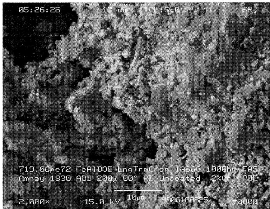
Figure 49: FAS upstream surface. Exposed for 1000 hours.
