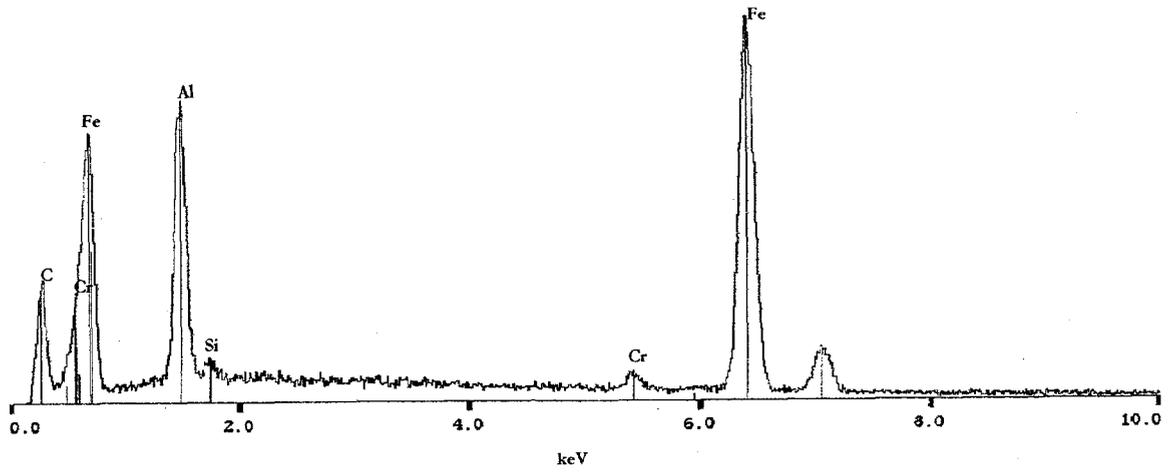
Figure 46: Partial field of base metal in Figure 45. Typical iron aluminide signature. No sulfur penetration.
