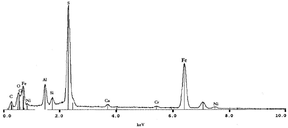
Figure 50: Full screen spectrum of Figure 49. High sulfur and iron. Strong indication of iron sulfide.
