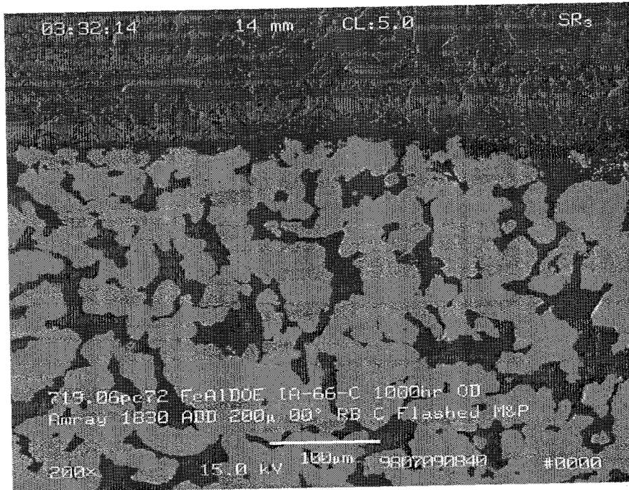
Figure 44: FAS cross-section. Upstream edge shown. Exposed for 1000 hours.
