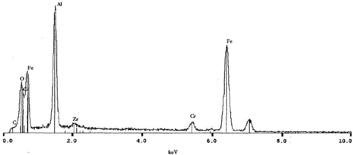
Figure 63: Full screen spectrum of Figure 62. Typical iron aluminide signature.
