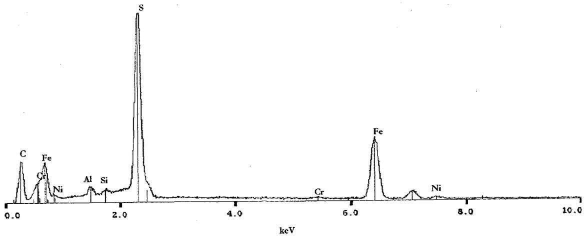
Figure 47: Partial field of upstream edge of Figure 45. High sulfur and iron. A strong indication of iron sulfides.
