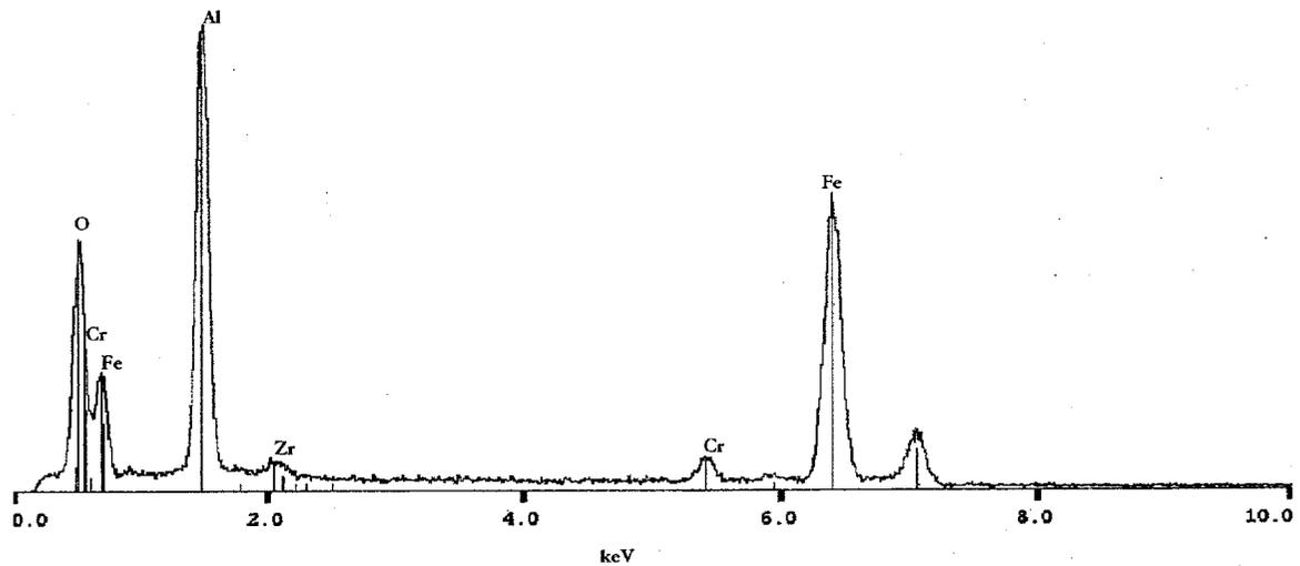
Figure 53: Full screen spectrum of Figure 52. Oxygen peak indicates a thin alumina layer on the surface of the sample.
