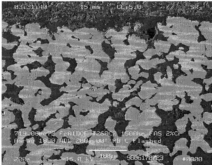
**Figure 54: FAS cross-section. Upstream edge shown. Exposed for 1500 hours. Iron sulfide crystals on upstream edge are barely visible at this magnification.**
