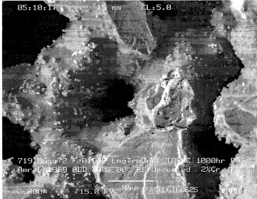
Figure 52: FAS fracture surface. Exposed for 1000 hours. Zirconia nodules, some porosity in the sinter bonds.
