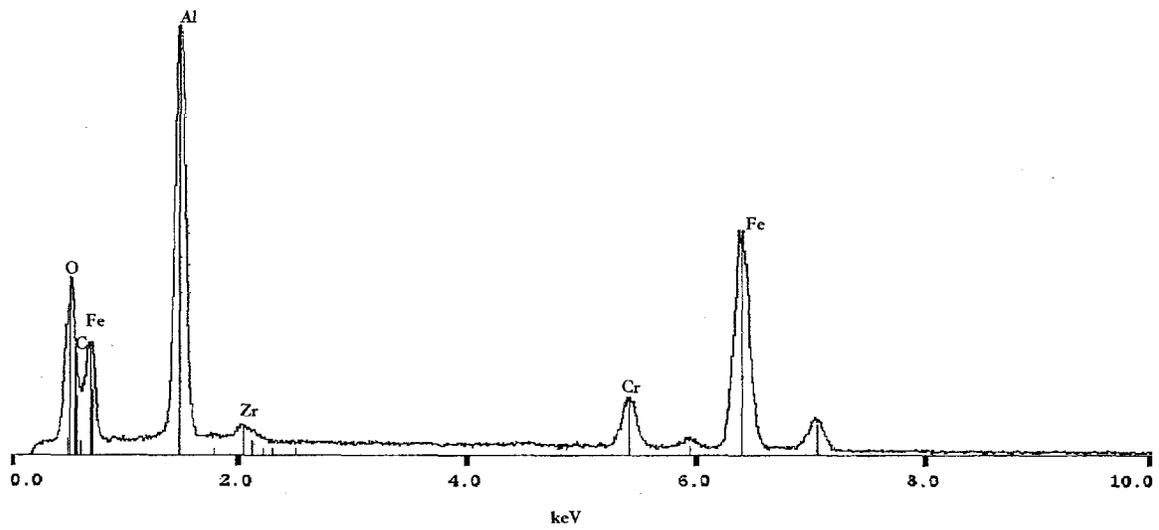
**Figure 72: Full screen spectrum of Figure 71. Typical iron aluminide signature. Alumina layer is detected by the presence of oxygen.**
