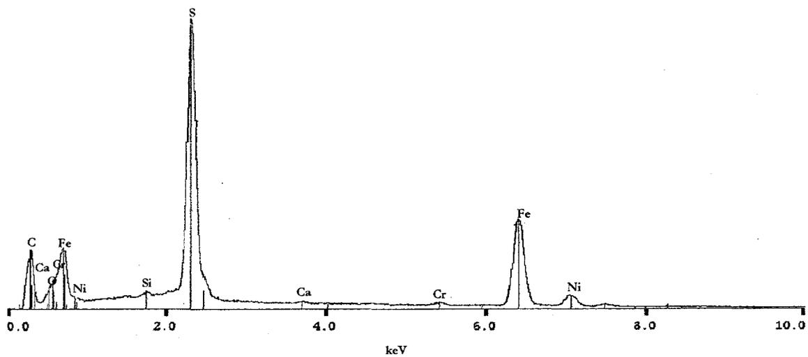
Figure 57: Spectrum of upstream edge of Figure 55. High sulfur and iron. Strong indication of iron sulfides.
