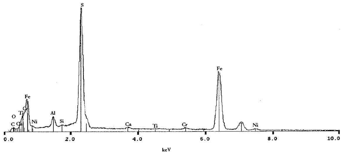
Figure 60: Full screen spectrum of Figure 59. High sulfur and iron. Strong indication of iron sulfides.
