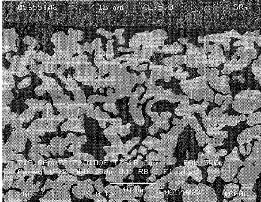
Figure 64: Cross-section of FAL control sample. Preoxidized for seven hours at 800°C.
