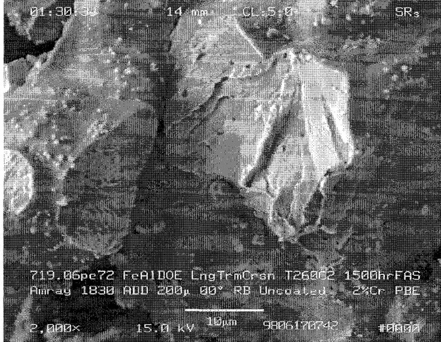
Figure 62: FAS fracture surface. Exposed for 1500 hours. Typical unexposed iron aluminide fracture surface with some porosity at sinter bond, zirconium/zirconia nodules on surface. Brittle transgranular fracture.
