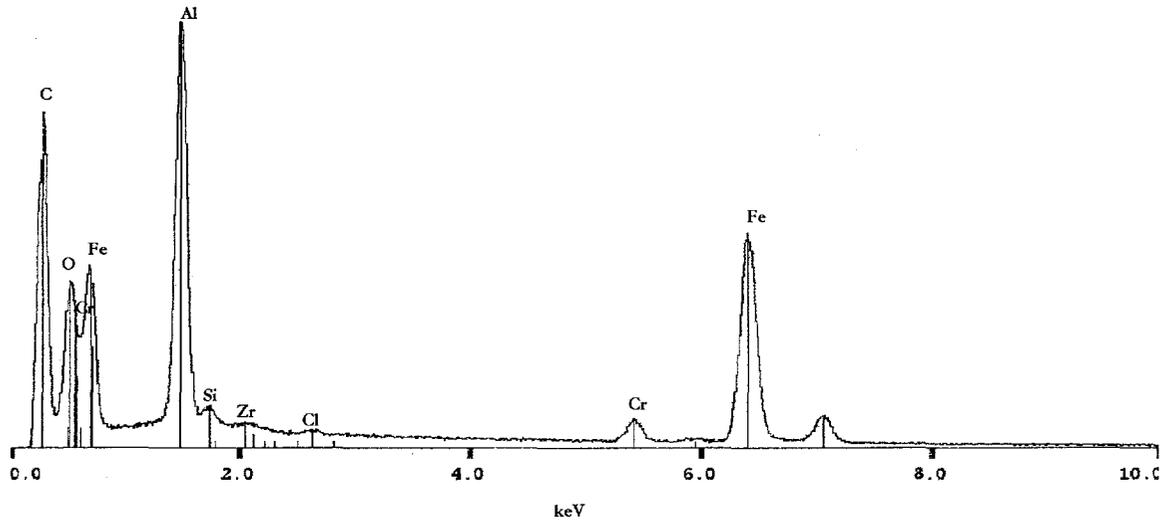
Figure 66: Partial field spectrum of base metal of Figure 65. High carbon is from carbon flashing.
