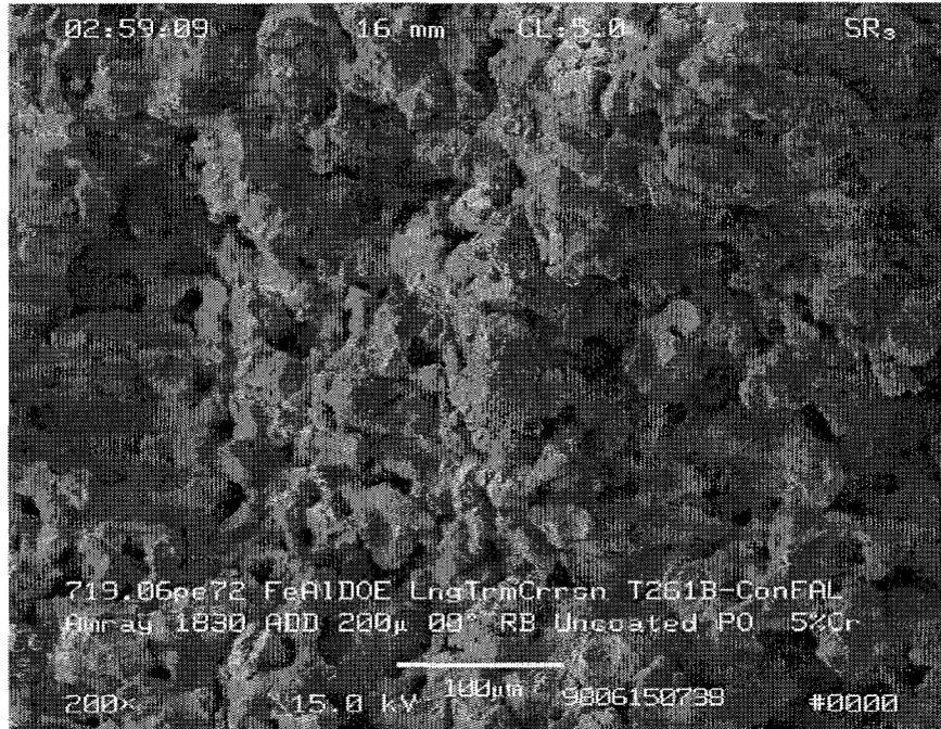
Figure 70: Fracture surface of FAL control sample. Preoxidized for seven hours at 800°C.
