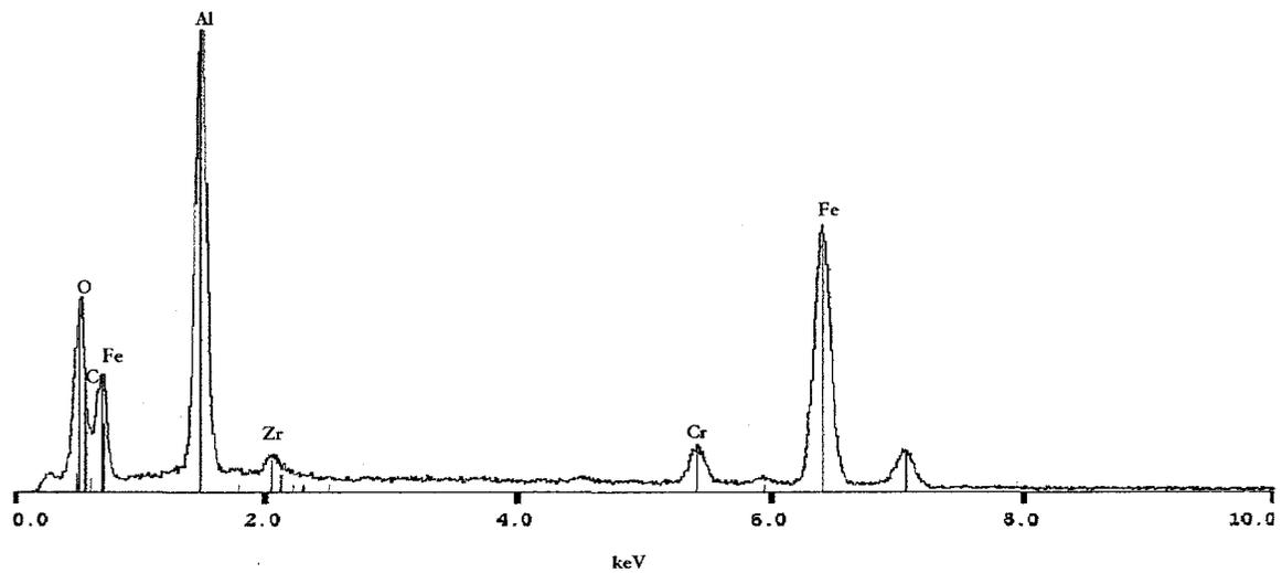
Figure 69: Full screen spectrum of Figure 68. Typical iron aluminide signature.
