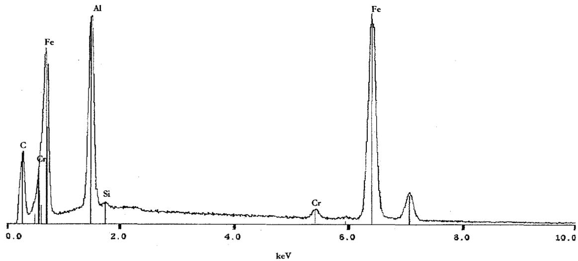
Figure 56: Spectrum of base metal on Figure 55. Typical iron aluminide signature.
