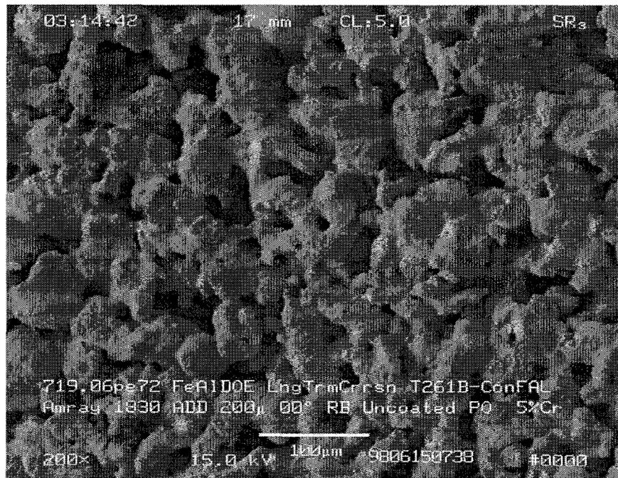
Figure 67: Upstream surface of FAL control sample. Preoxidized for seven hours at 800°C.
