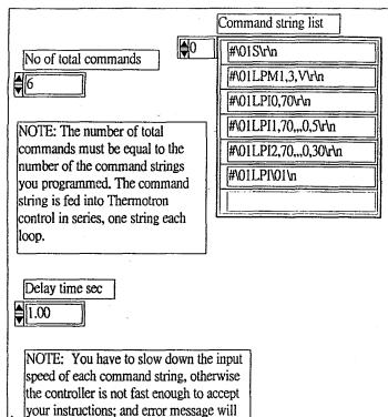
NOTE: The communication between LabVIEW vi to Thermotron temperature controller is via RS-485 serial port. The port number assigned for this system is port number 5.
