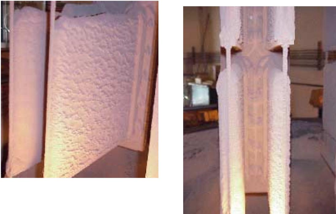
**Figure 4.20 - Ash Accumulation on Sheet Filter Elements During HTHP Testing**
