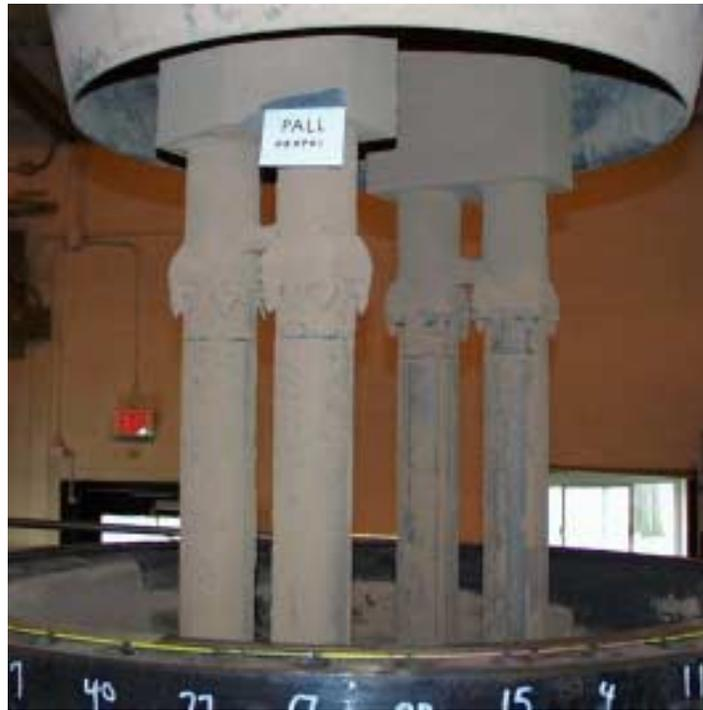
**Figure 3.14 - Pall FeAl Inverted Candle Internals Following Testing**
