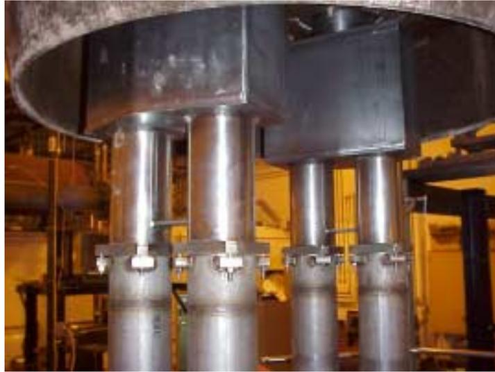
**Figure 3.10 - Plenums with Inverted Candles Installed**
