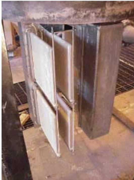
**Figure 4.12 - Blasch Sheet Filter Elements Installed for HTHP Testing**
