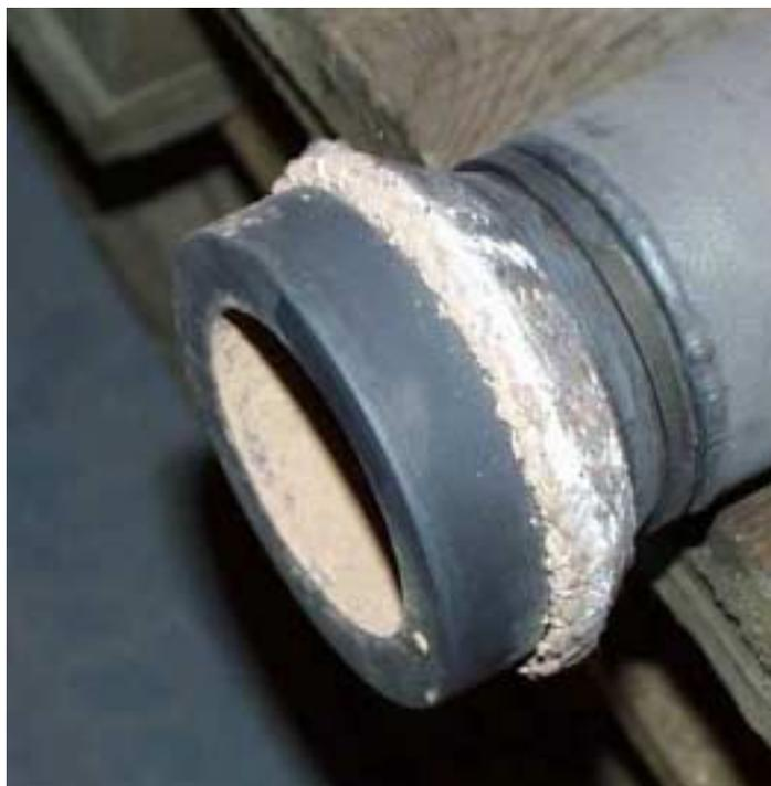
**Figure 3.15 - Condition of Pall Inverted Candle Gaskets Following Testing**
