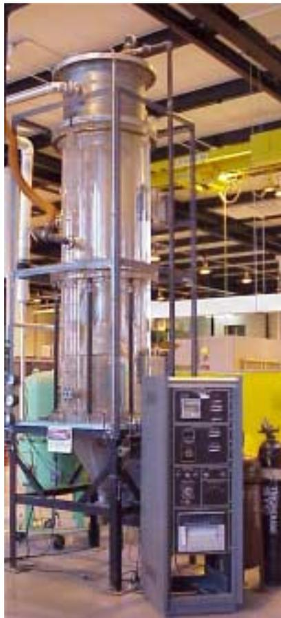
**Figure 3.4 - The Inverted Candle Cold Flow Test Facility**
