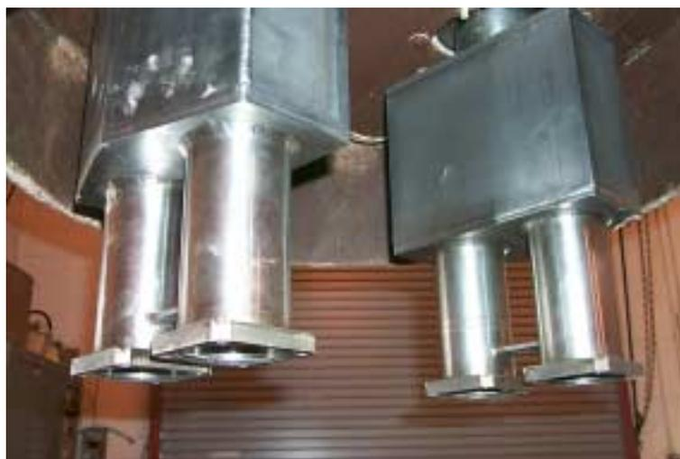
**Figure 3.9 - Initial Installation of Inverted Candle Plenums**
