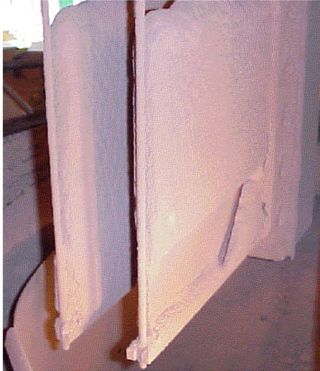
**Figure 4.19 - Broken Blasch Sheet Filter Element in HHP Tests**
