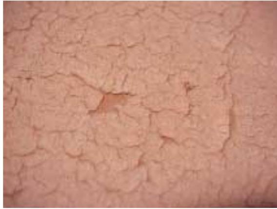
**Figure 4.8 - Damaged Surface of Blasch Sheet Filter Element after Cold Flow Tests**
