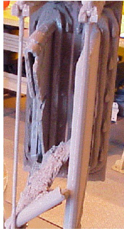
**Figure 4.7 - Damaged IF&P Recrystallized SiC Sheet Filter Element in a Cold Flow Test**
