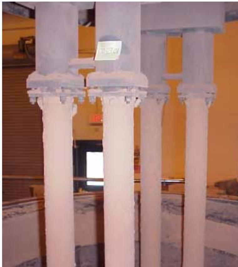
**Figure 3.18 - Standard Candles Following Testing**
