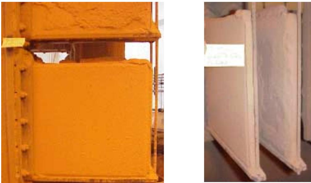
**Figure 4.21 - Bottom Sheet Filter Elements on Pulsed Plenum**
