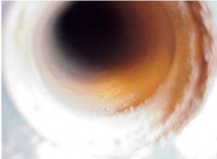
**Figure 3.17 - Ash Cake on the Bore of an Inverted Candle Following Testing**
