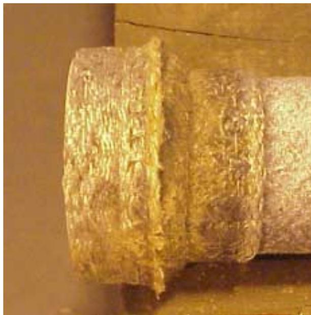
**Figure 3.16 - Condition of McDermott Inverted Candle Gasket Following Testing**
