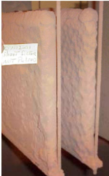
**Figure 4.22 - Bottom Sheet Filter Elements on Non-pulsed Plenum**
