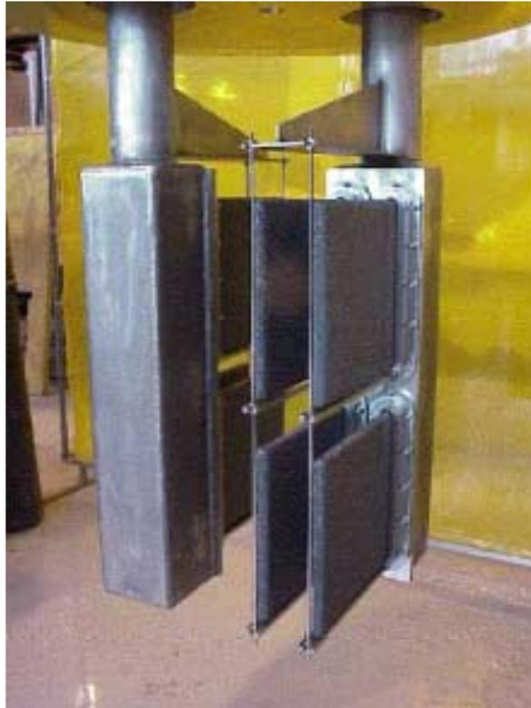
**Figure 4.5 - Sheet Filter Test Clusters**
