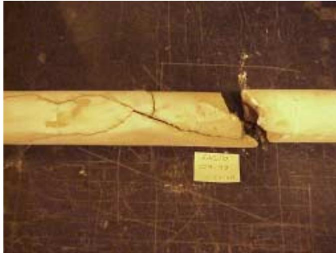
**Figure 3.13 - Fractured ENSTO Inverted Candle**
