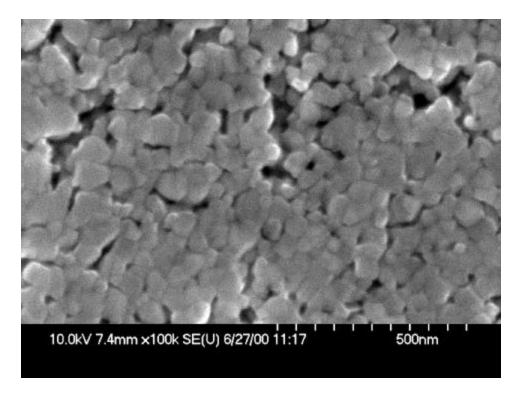
Figure 9. Surface of Ceria film on sapphire which was sintered at 1000°C.
