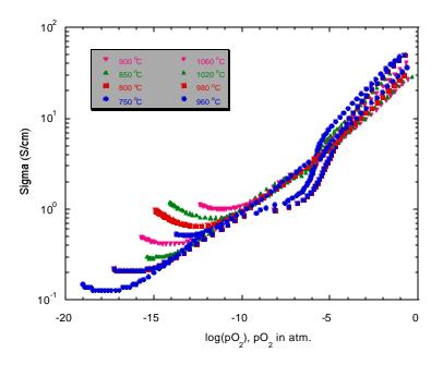
Figure 4 Conductivity Data for La<sub>0.2</sub>Sr<sub>0.8</sub>Fe<sub>0.8</sub>M<sub>0.2</sub>O<sub>3-x</sub>
