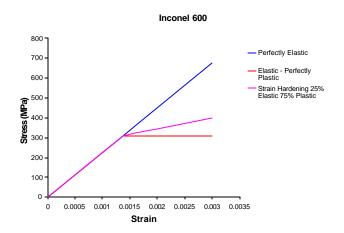
Figure 9: Simulated strain-hardening stress strain curve for Inconel 600 at room temperature.
