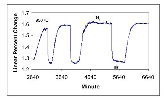
Figure 4. Thermal Expansion of dense (La<sub>0.59</sub>Sr<sub>0.40</sub>)<sub>0.99</sub>FeO<sub>3</sub>
