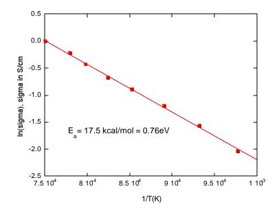
Figure 6 Ionic conductivity of La<sub>0.2</sub>Sr<sub>0.8</sub>Fe<sub>0.8</sub>M<sub>0.2</sub>O<sub>3-x</sub>
