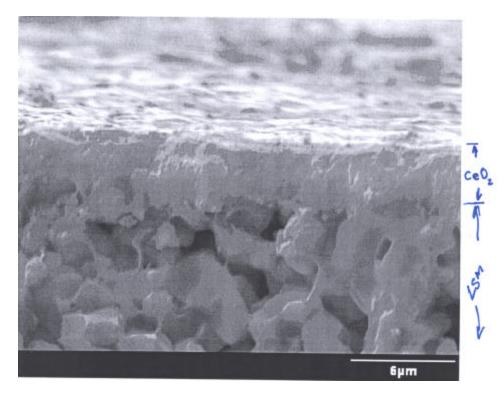
Figure 12. Colloidal ceria planarizing layer. Cross section, high resolution. Sintering temperature of composite =  $1000^{\circ}$ C.
