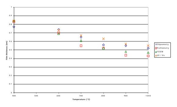
Figure 5. Variation in the film thickness of porous  $CeO_2$  thin films as a function of annealing temperature as measured with different techniques.
