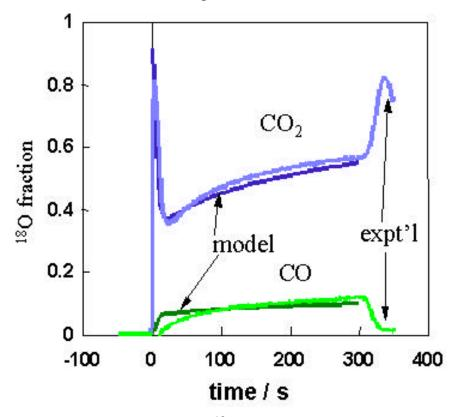
Figure 1. The data and model predictions for the <sup>18</sup>O distribution between CO and CO<sub>2</sub>.
