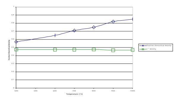
Figure 8. Variation in the density of porous  $CeO_2$  thin films measured with UV/Vis spectrophotometry as a function of annealing temperature.
