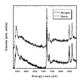
Figure 12: EELS of bright and dark columns in (La.Sr)FeO<sub>3</sub> at 451° C
