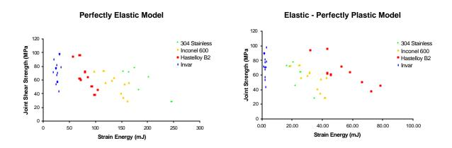
Figure 8: Correlation between elastic strain energy predictions and experimental data
