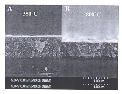
Figure 6. SEM cross-sections of  $CeO_2$  coatings on the sapphire substrate. A, B – after sintering at 400°C and 800°C correspondingly.
