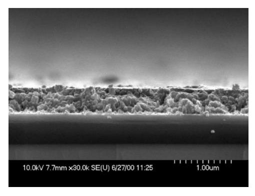
Figure 10. Cross-section of Ceria film on sapphire sintered at 1000°C.
