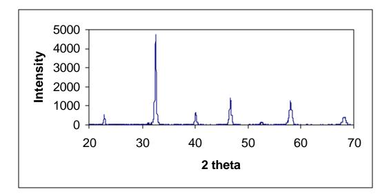
Figure 1. XRD pattern of disk La<sub>0.60</sub>Sr<sub>0.40</sub>Fe<sub>0.85</sub>Ga<sub>0.15</sub>O<sub>3</sub> (A), a major Perovskite phase
