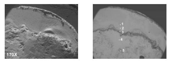
Figure 1: (L) Wetting of Alloy 1 on ceramic surface. (R) EDS data points (Table 2)
