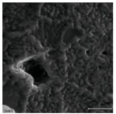
Fig. 3 Fracture initiation flaws – a) Surface and b) volume.
