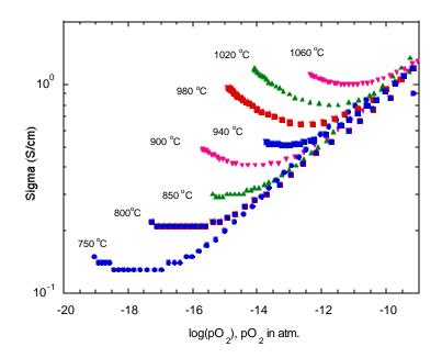
Figure 5. Low Pressure Conductivity Data for La<sub>0.2</sub>Sr<sub>0.8</sub>Fe<sub>0.8</sub>M<sub>0.2</sub>O<sub>3-x</sub>
