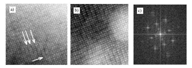
Figure 11: a) Z-Contrast image with marked change in contrast in every second FeO<sub>2</sub> column.
