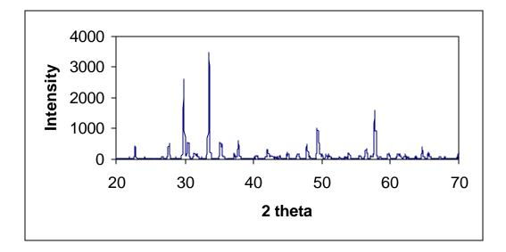
Figure 2. XRD pattern of disk La<sub>0.20</sub>Sr<sub>0.80</sub>GaO<sub>3</sub> (B), a multi-phase of oxides
