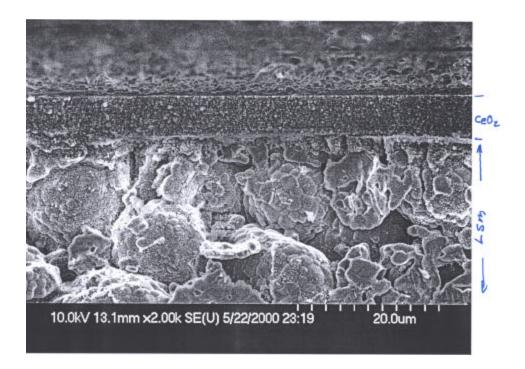
Figure 11. Colloidal CeO<sub>2</sub> porous (60%) th. Density) thin film on porous LSM substrate. Composite was sintered at  $1000^{\circ}$ C.
