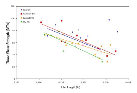
Figure 7: Load supported by concentric metal-ceramic joints. 3.5 mil braze thickness.
