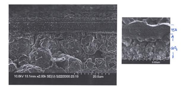
Figure 13. Field-emission SEM micrograph of a YSZ/Colloidal CeO<sub>2</sub>/spray-pyrolized LSM composite. CeO<sub>2</sub> =  $5\mu$ m, YSZ =  $0.5\mu$ m. Composite sintered at 800°C.
