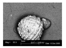
Figure 2: Wetting of Alloy 2 on Ceramic
