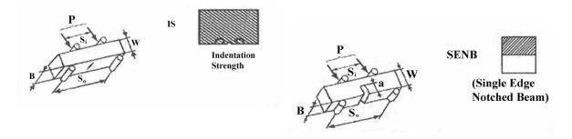
Figure 5 Testing configuration for crack growth studies.
