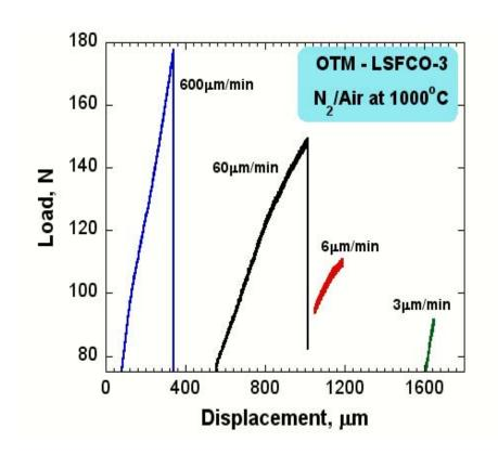
Figure 3 OTM flexural strength at varying stress rates in  $N_2$ /Air at 1000°C.
