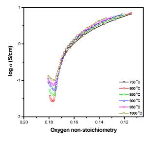
Figure 11 Dependence of conductivity on oxygen non-stoichiometry
