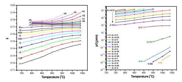
Figure 10 The  $\delta$  dependence on temperature at constant pO<sub>2</sub> (left) and the pO<sub>2</sub> dependence on temperature at constant  $\delta$  (right).
