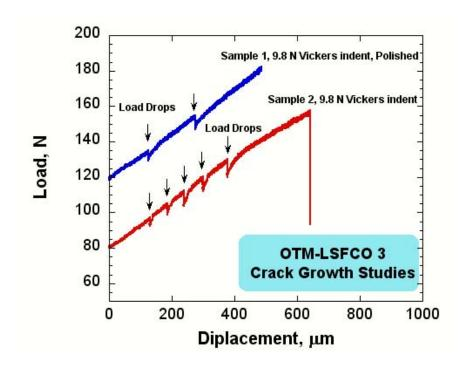
Figure 6 Load-displacement plots for fracture toughness studies in environment. The fracture toughness for the single edge notched beam (SENB) specimen tested in four-point bending,  $K_{INB}$  is calculated using the equations 6 to 7. These equations are valid in the condition 0 < a/W < 1.
