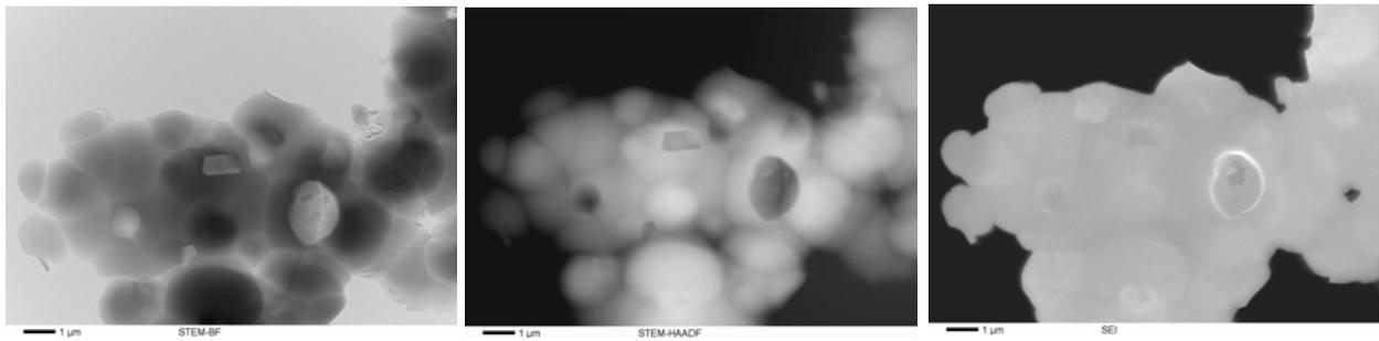
Figure 14: (a) Bright field (b) Z-contrast and (c) secondary electron images of a representative area of the membrane material.
