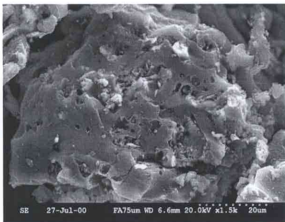
Figure 8. SEM image of the unburned carbon.
