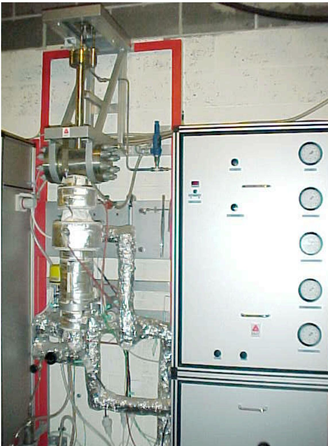
Figure 7.2 High pressure, high temperature thermogravimetric apparatus (DMT-TGA).
