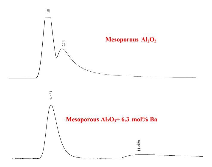
Fig.1. Gas chromatograph when mixtures of  $CO_2$  and  $N_2$  (50/50) gases were passed through columns packed with mesoporous alumina with and without Ba.
