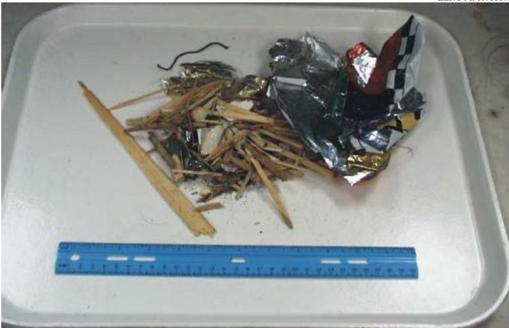
Figure C6. Combined wood, aluminum, ferrous, food waste, glass fraction in RDF.
