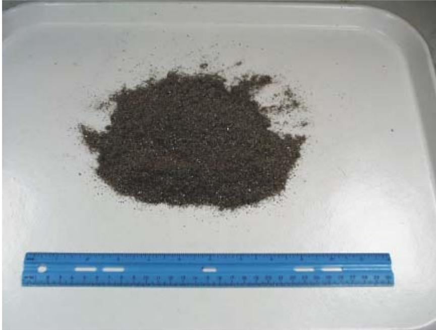
Figure C9. -20-mesh fraction in RDF.
