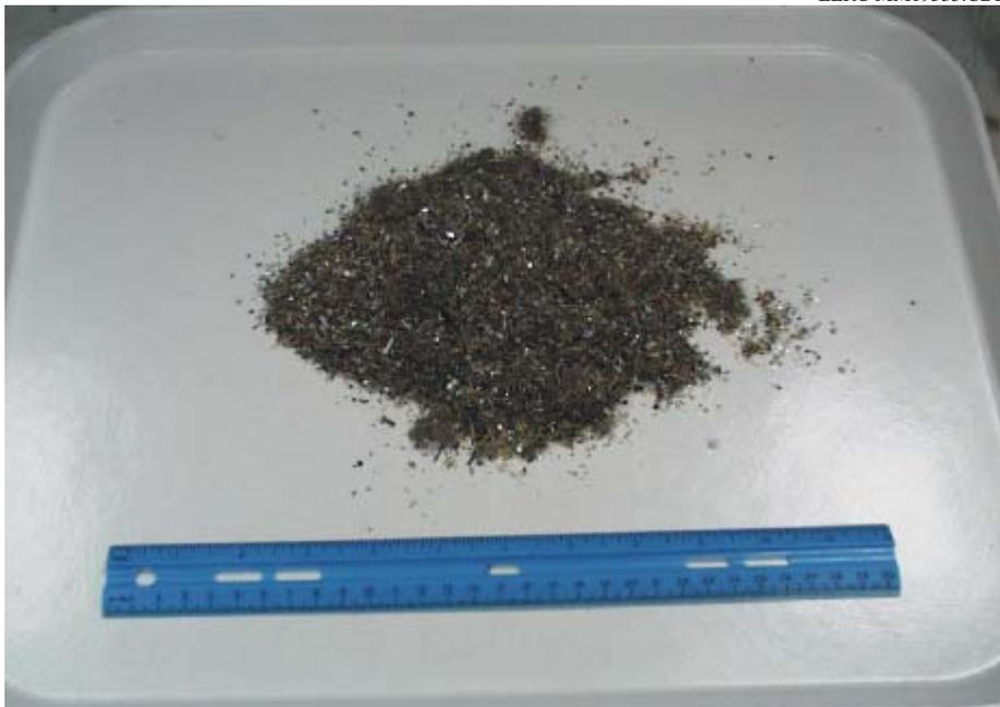
Figure C8.  $\_10\text{-mesh x + 20-mesh}$  fraction in RDF.
