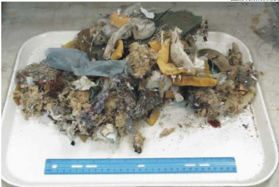
Figure C4. Textiles fraction in RDF.
