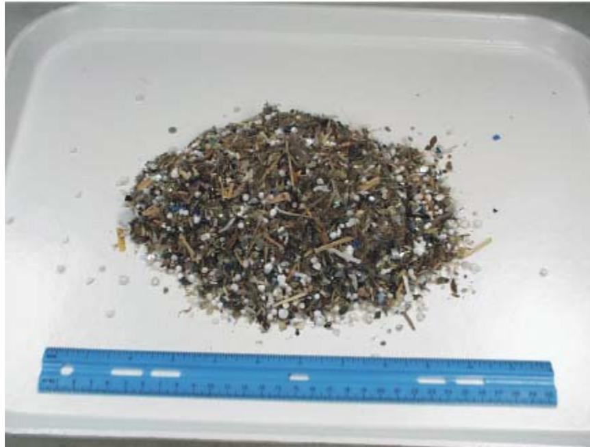
Figure C7.  $\_4\text{-mesh x + 10-mesh}$  fraction in RDF.
