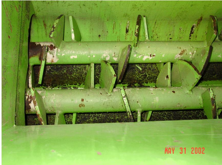
Figure 11. Hopper and overlapping augers of twin-screw feeder.
