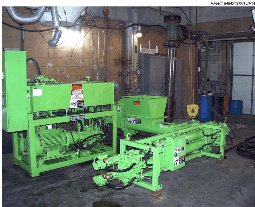
Figure 10. High-solids sludge pump, twin-screw feeder, and power pack used at the EERC.
