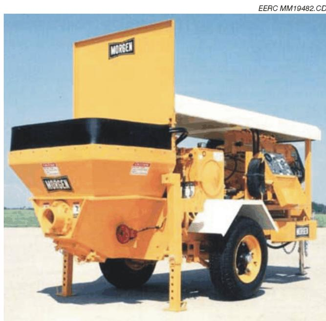
Figure 5. Morgen Mustang trailer-mounted concrete pump.
