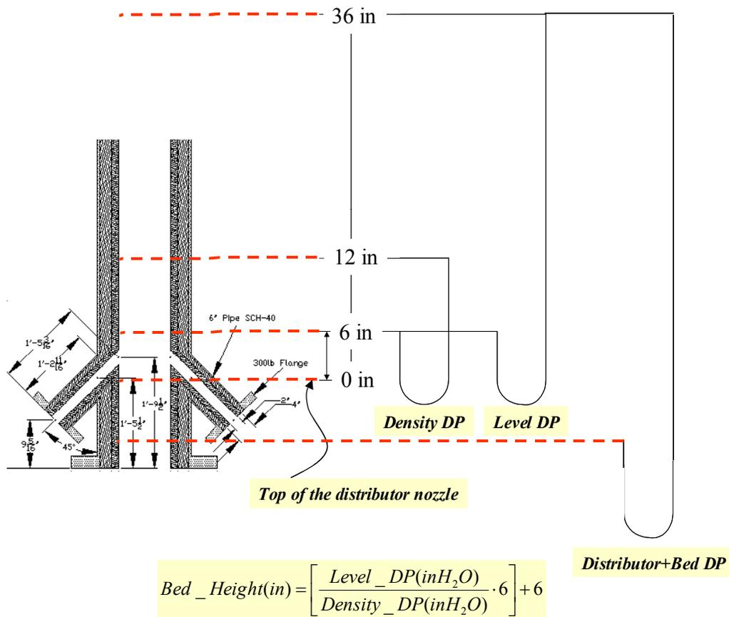
Figure 13. Locations of differential pressure measurements for bed height estimation.
