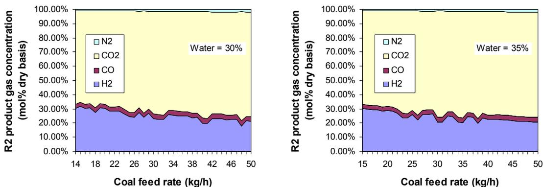
Figure 8. R2 product gas concentration as a function of coal feed rate for different coal-water slurry concentrations (% water in slurry).
