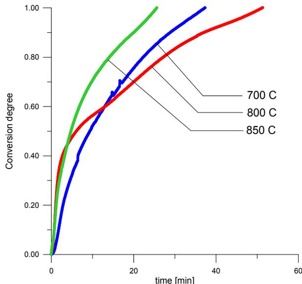
Figure 5. Conversion degree as a function of time for a 90% N<sub>2</sub>, 2% CO, 8% H<sub>2</sub> mixture at a variety of temperatures.
