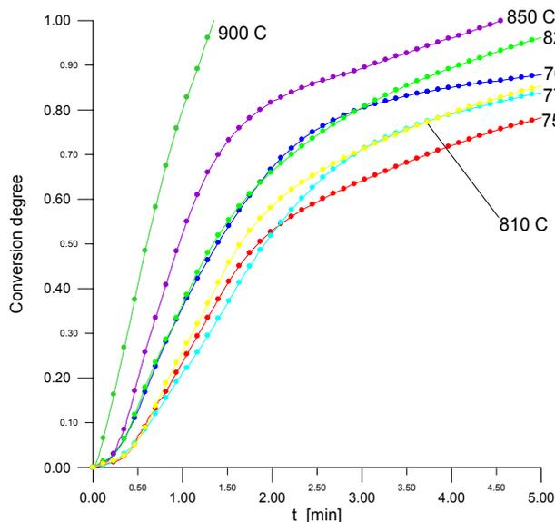
Figure 4. Conversion degree as a function of time for a 90% N<sub>2</sub>, 5.7% CO, 4.3% H<sub>2</sub> mixture at a variety of temperatures.
