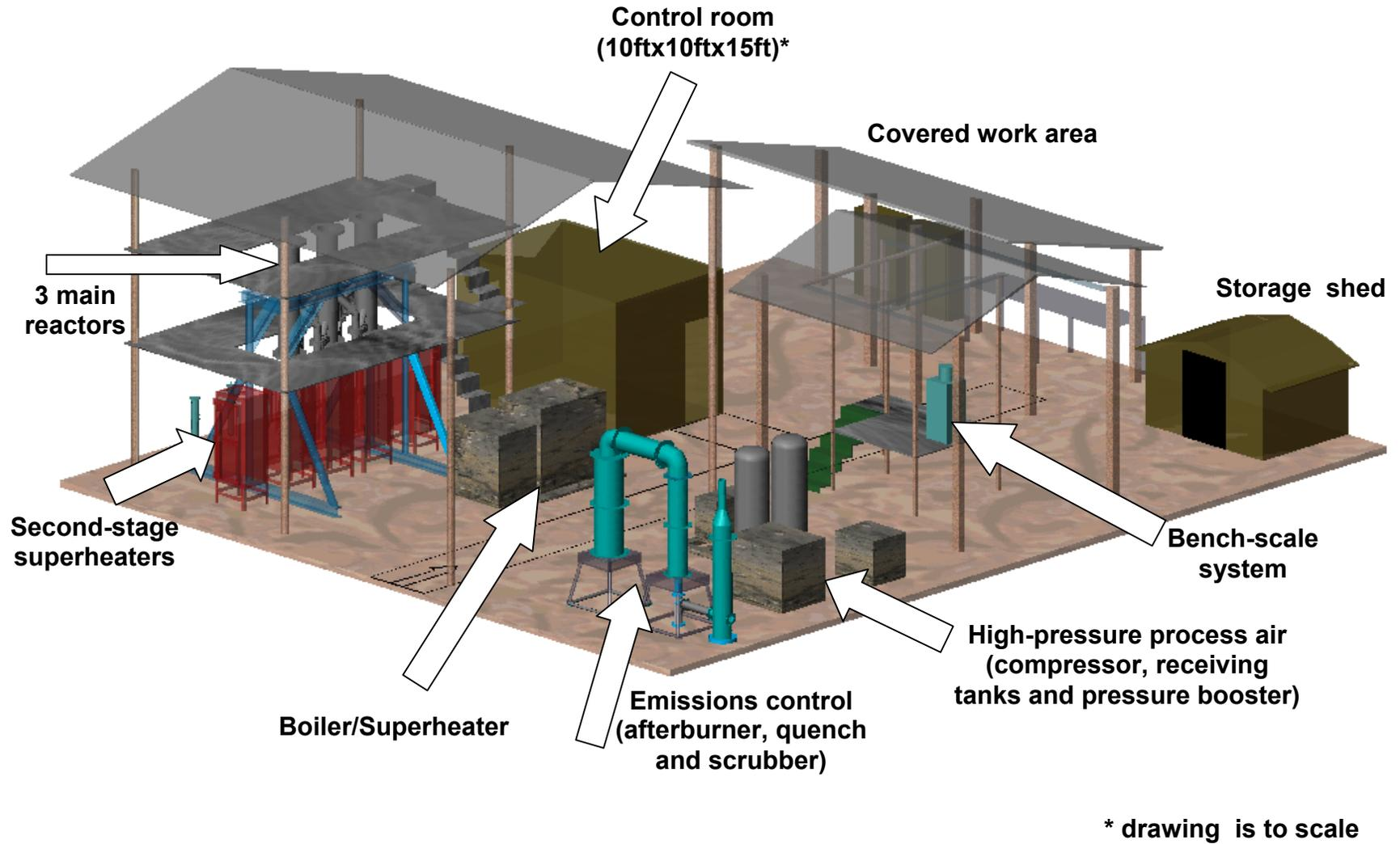
Figure 16. Layout of pilot-scale system.
