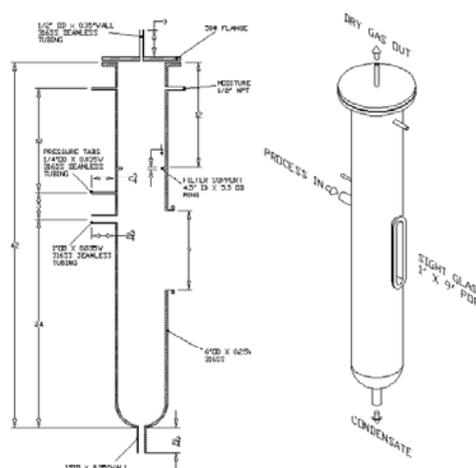
Figure 12. Schematic diagram of mist eliminator for water removal from product gas.
