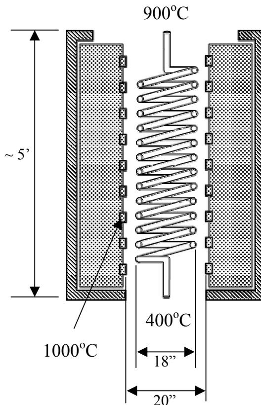
Figure 9. Schematic diagram of second-stage superheater: electric furnace and heating coil.
