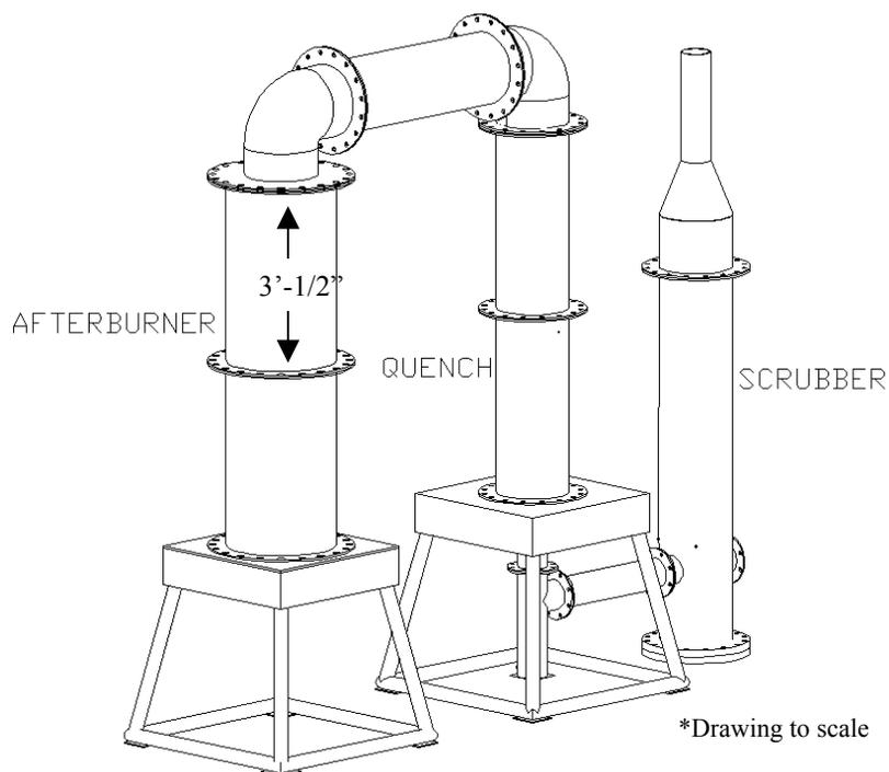
Figure 15. Air pollution control system: afterburner, quench and scrubber.
