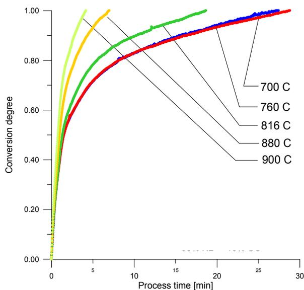
Figure 2. Conversion degree as a function of time for a 90% N<sub>2</sub>, 10% CO mixture at a variety of temperatures.
