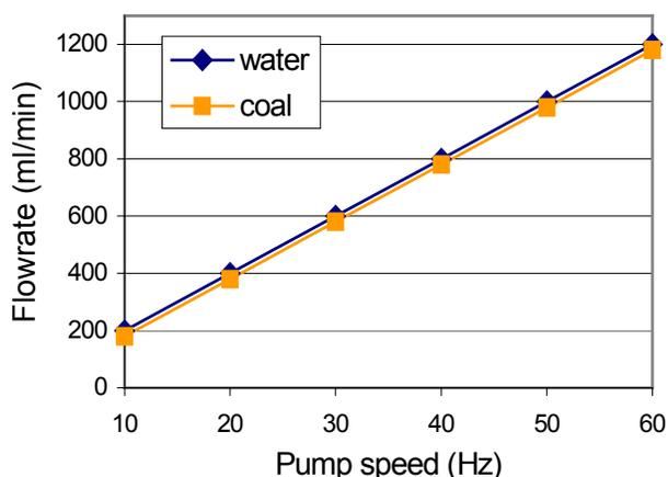
Figure 10. Flow rate of coal and water at increasing slurry pump speeds.
