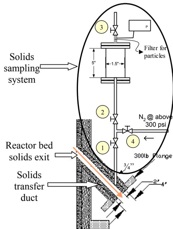
Step A, purging the sampling line between valve 1 and the solids transfer duct will ensure that a representative sample is obtained. Purging the sampling system, Step B, ensures that the sample is recovered under an inert atmosphere, preserving the
