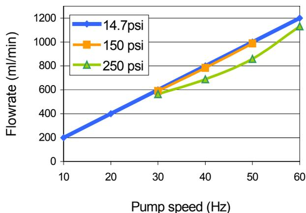
Figure 11. Water flow rate at increasing slurry pump speeds for three pressures.
