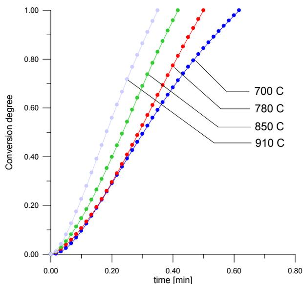
Figure 3. Conversion degree as a function of time for a 90% N<sub>2</sub>, 10% H<sub>2</sub> mixture at a variety of temperatures.
