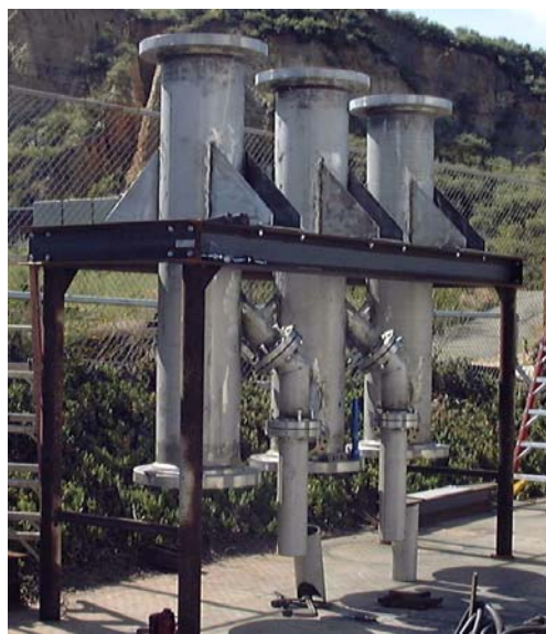
Figure 17. Photo of three pilot-scale reactors mounted on stand.
