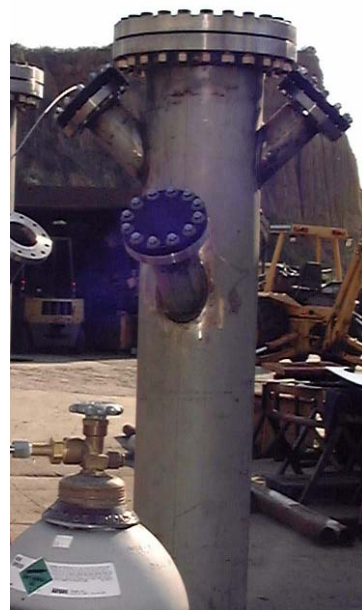
Figure 14. Hydrostatic test of Reactor 2.
