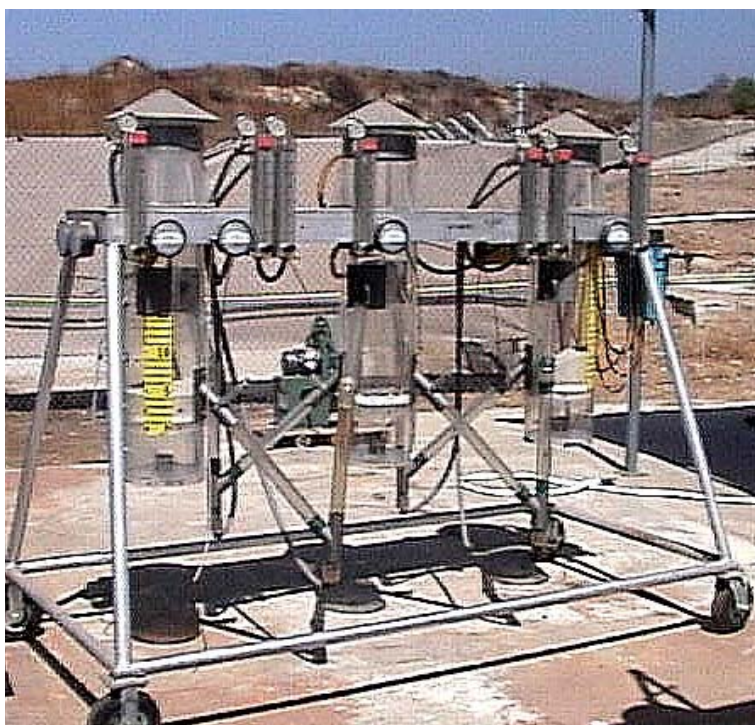
Figure 20. Cold flow model: 3 circulating fluidized beds.
