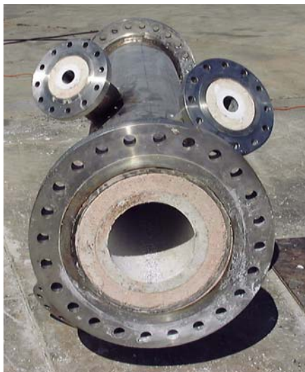
Figure 15. Reactor 1 shell with two-cast refractory layers.
