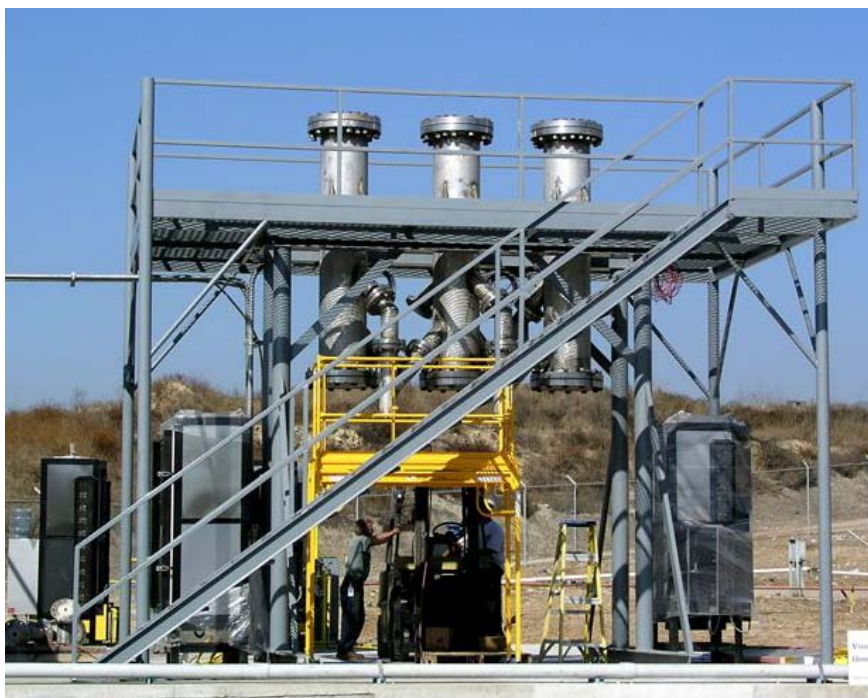
Figure 25. Side view of pilot-scale system with three reactors, scaffolding and second-stage superheaters shown.
