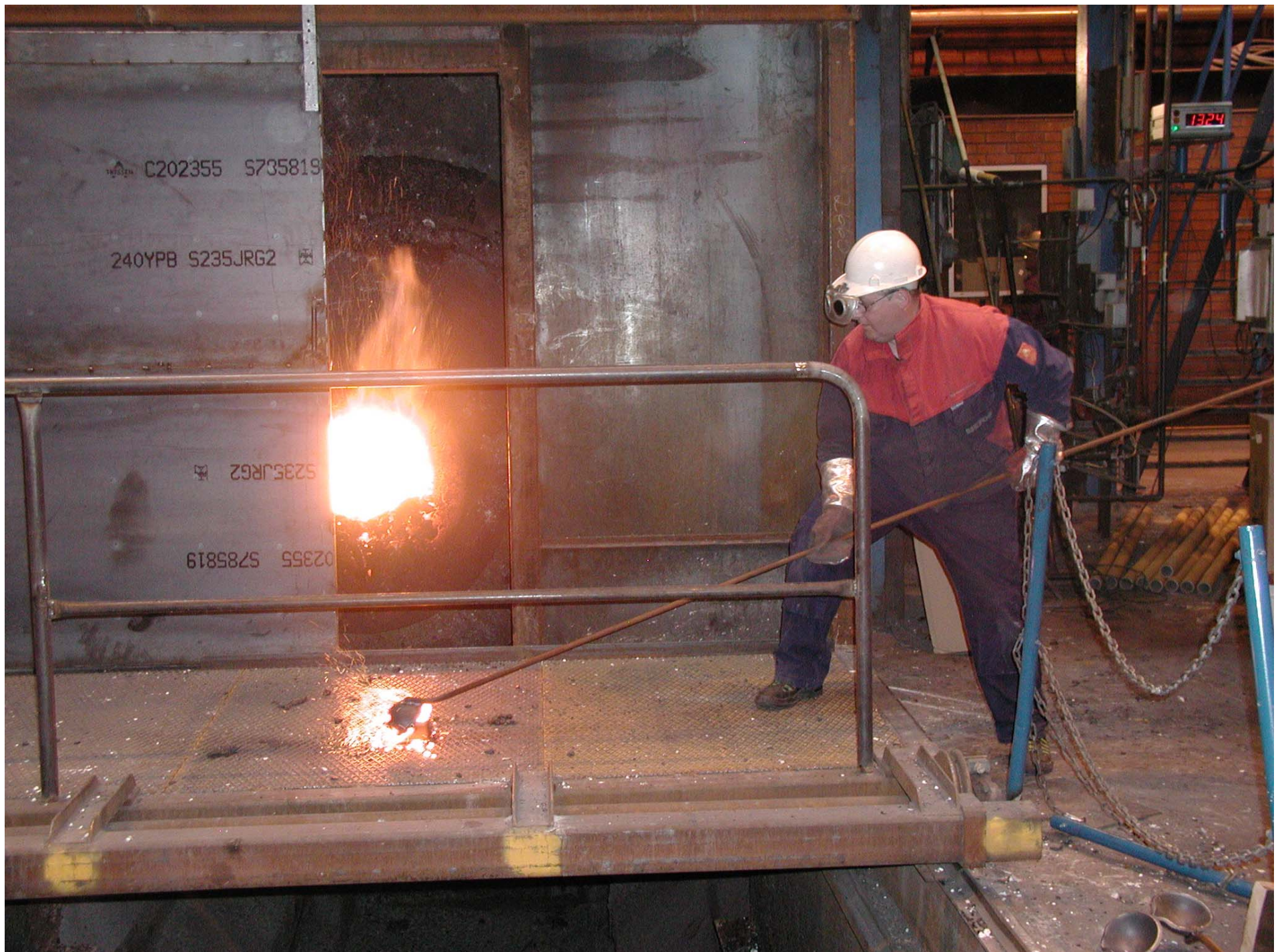
Figure 4 Slag Sampling from Tilted Converter
