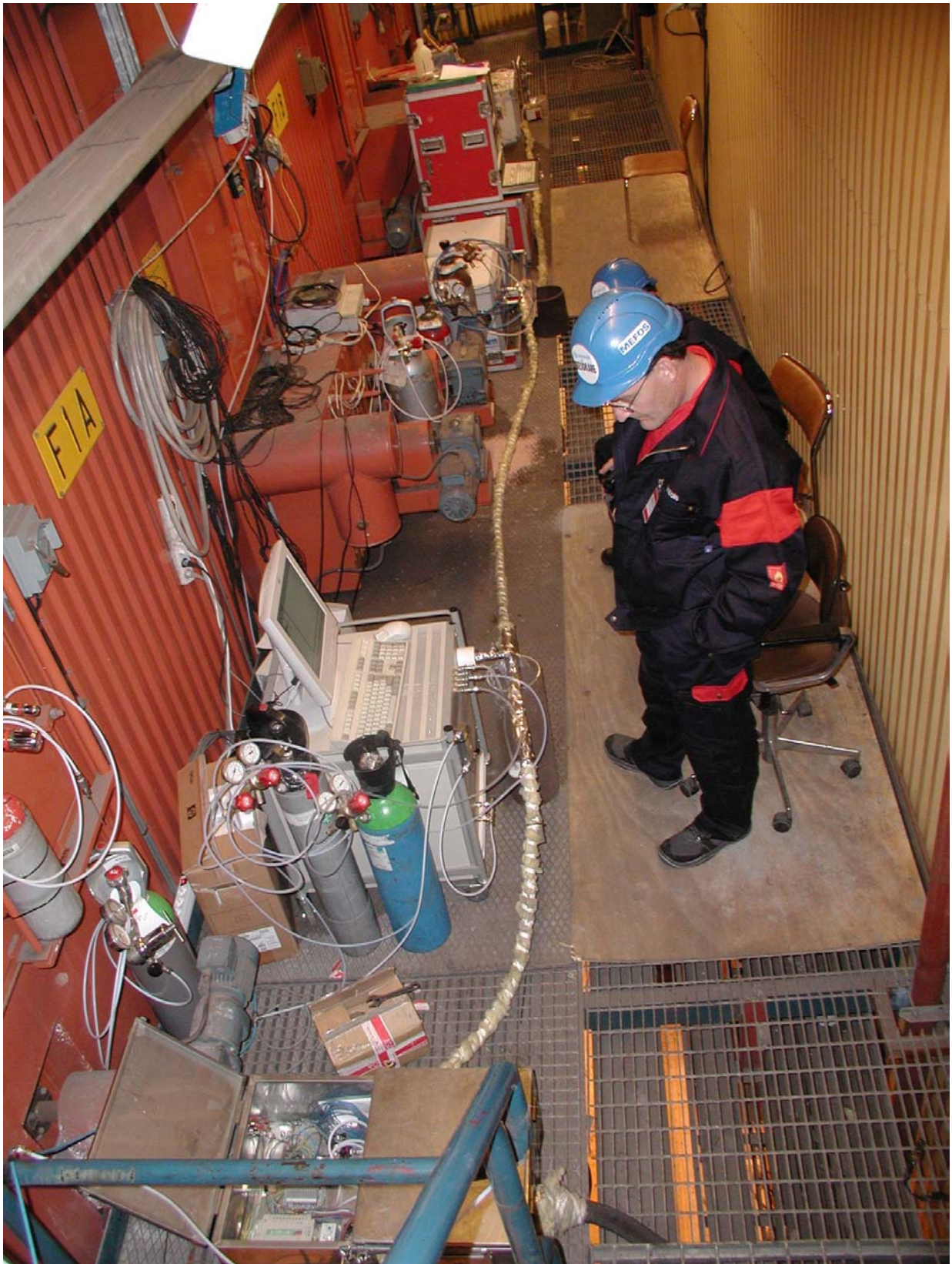
Figure 7. On-Line Mass Spectrometer for Gas Analysis
