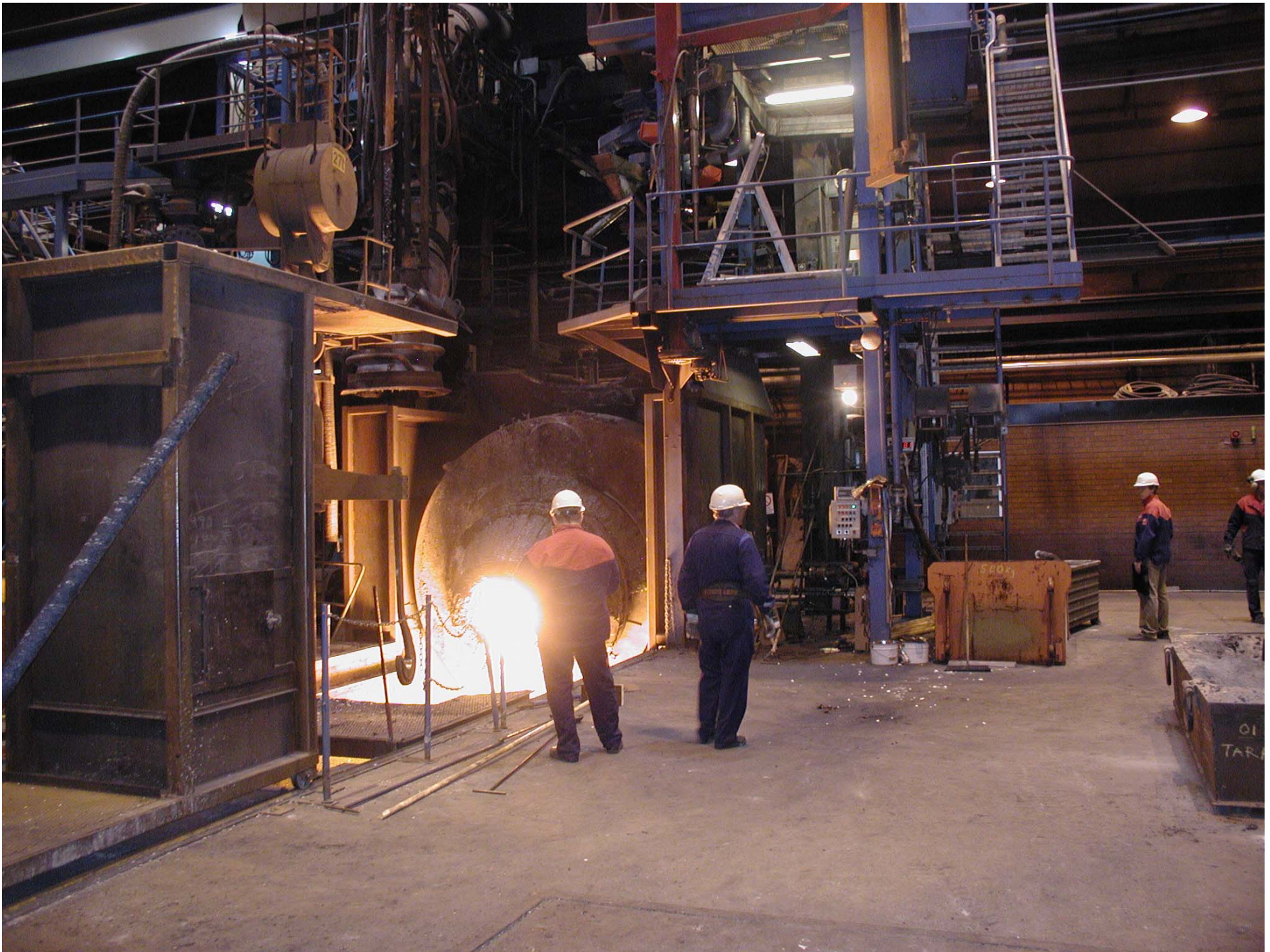
Figure 5 Metal Pour from Converter at Day's End
