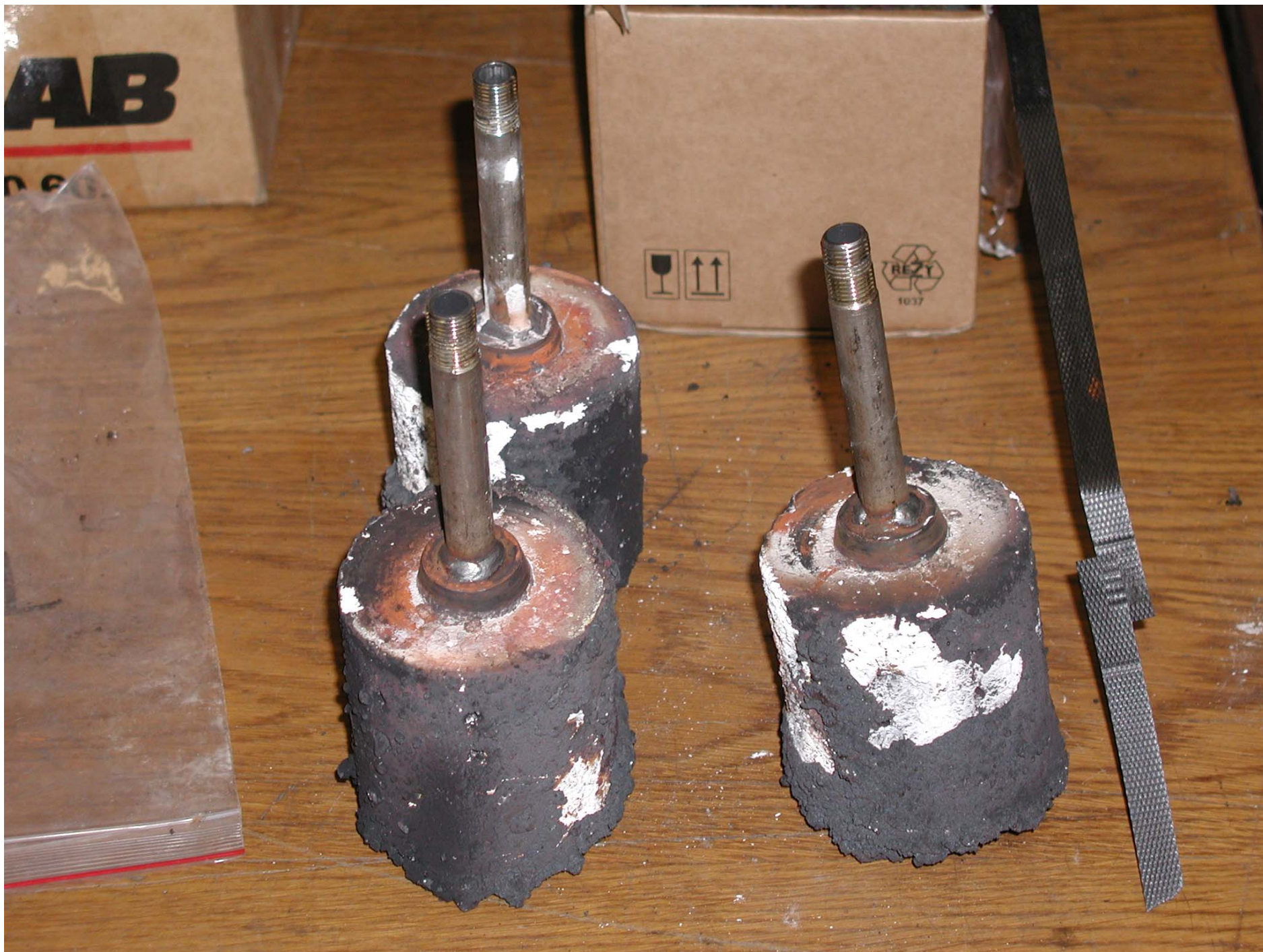
Figure 6 Used Ceramic Filters from Gas Sample Probe
