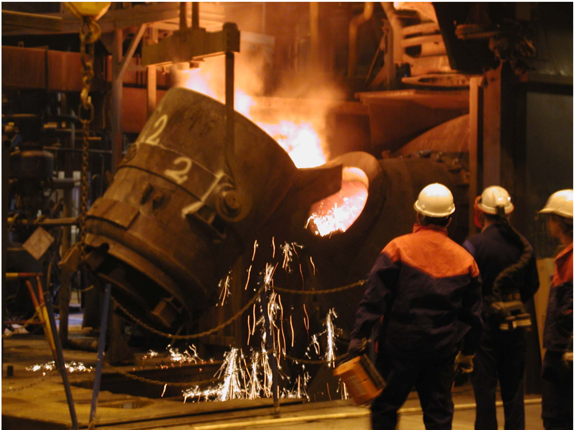
Figure 2 Metal Transfer to the Universal Converter
