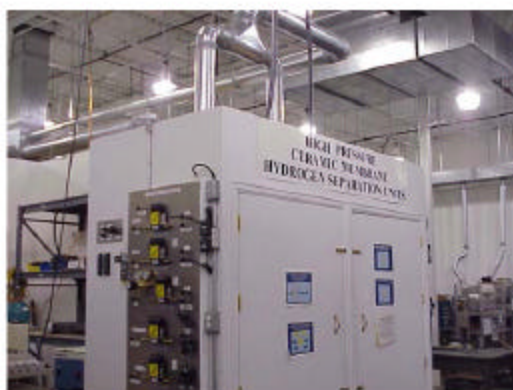
Figure 11. Containment facility designed to capture and vent gases from high pressure units in the event of leaks. Mass flow controllers are seen on the left.
