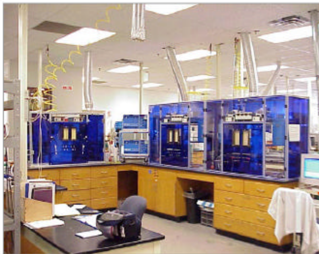
Figure 8. Six new reactor stations built for testing membranes at ambient pressure. On the left are two stations designed to measure hydrogen flux under ideal conditions in the absence of catalyst poisons using purified mixtures of hydrogen and helium in the feed stream. On the right are four reactors which were used for testing membranes in the presence of the sulfur contaminated water-gas shift mixture and steam at ambient pressure. These four systems were designed to contain and vent H 2 S, COS, and CO in the event of leaks. In the center are two gas chromatography instruments used for measuring hydrogen concentration on the permeate side of the membranes.
