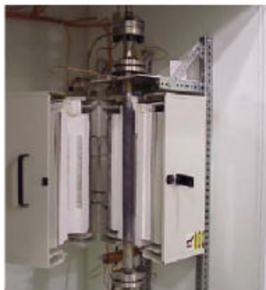
Figure 12. One of two high pressure reactors dedicated to testing hydrogen transport membranes. The unit shown is designed to operate at up to 900°C (1173 K) and 300 psi (20 bar) differential pressure. Furnace surrounds reactor tube. A pressure relief valve is at the top of the unit.
