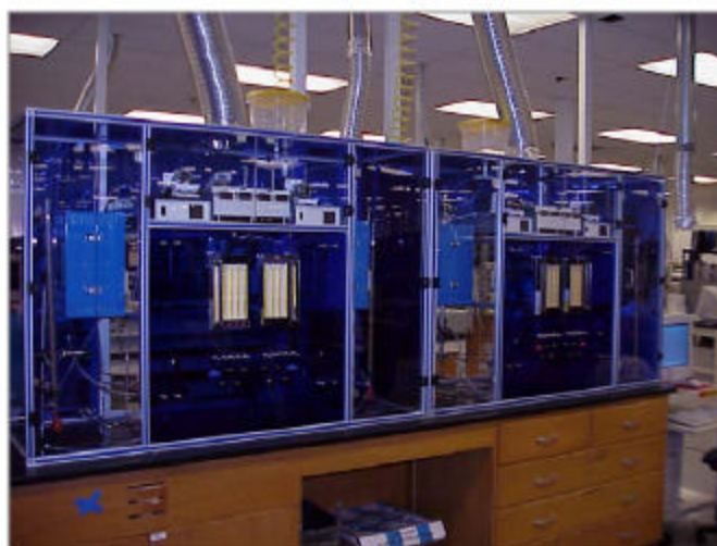
Figure 10. The four reactor stations built which were used to test the membranes under steam and water-gas shift gas components at ambient pressures. The cabinets and exhaust vents were designed to contain and vent toxic H_2S , CO and COS in the event of a leak in the gas lines. Carbon monoxide sensors placed within the cabinets sound an alarm in the event that CO levels exceed safety guidelines. Air flow in the cabinets and vents is calculated to dilute H_2S in the exhaust to levels below OSHA allowed guidelines. Calibrated peristaltic pumps were used to inject liquid water, which was converted into steam and mixed with the dry components of the water-gas shift mixture.
