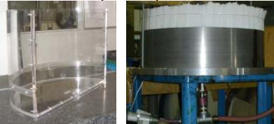
material in a filled CFRP mould of full scale. The tests will give us information regarding flow of resin/leveling in the mould, adhesion of resin to the membranes and canister and most important possible formation of cracks due to exothermic reaction/thermal expansion.
