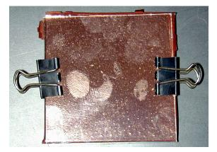
Figure 1 –Copper film (3  $\mu$ m) on PVA; sample is sandwiched between two pieces of glass
