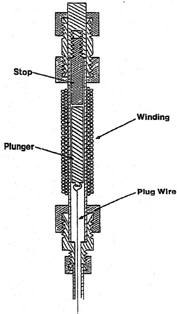
Figure 6.6. A Schematic Cross-Sectional Diagram of a Solenoid Used to Actuate the Sliding Plug.
