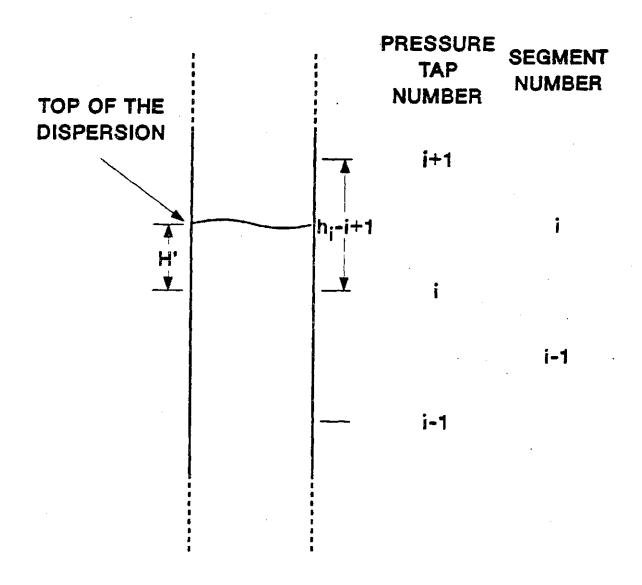
Figure B-1. Schematic diagram of the top of the dispersion with respect to pressure tap locations
