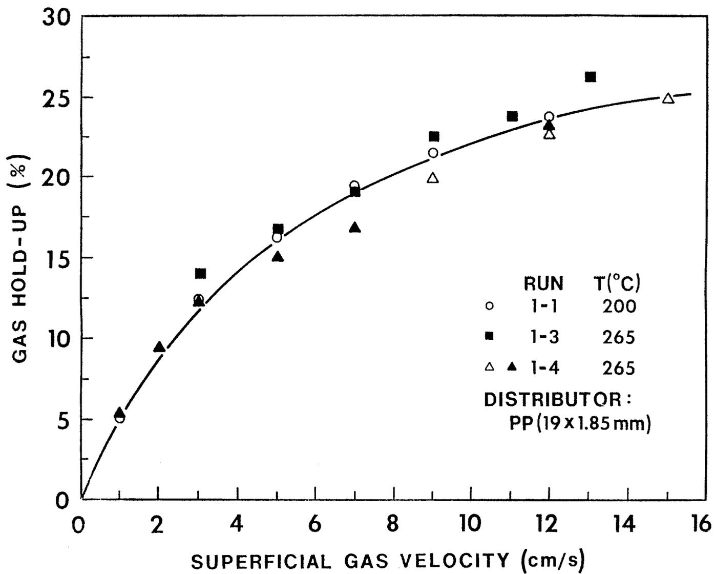
Figure 2. Effect of temperature and gas velocity on hold-up in the "nonfoamy" flow regime (AM-9G column; Open symbols: increasing gas flow rate; Solid symbols: decreasing gas flow rate).
