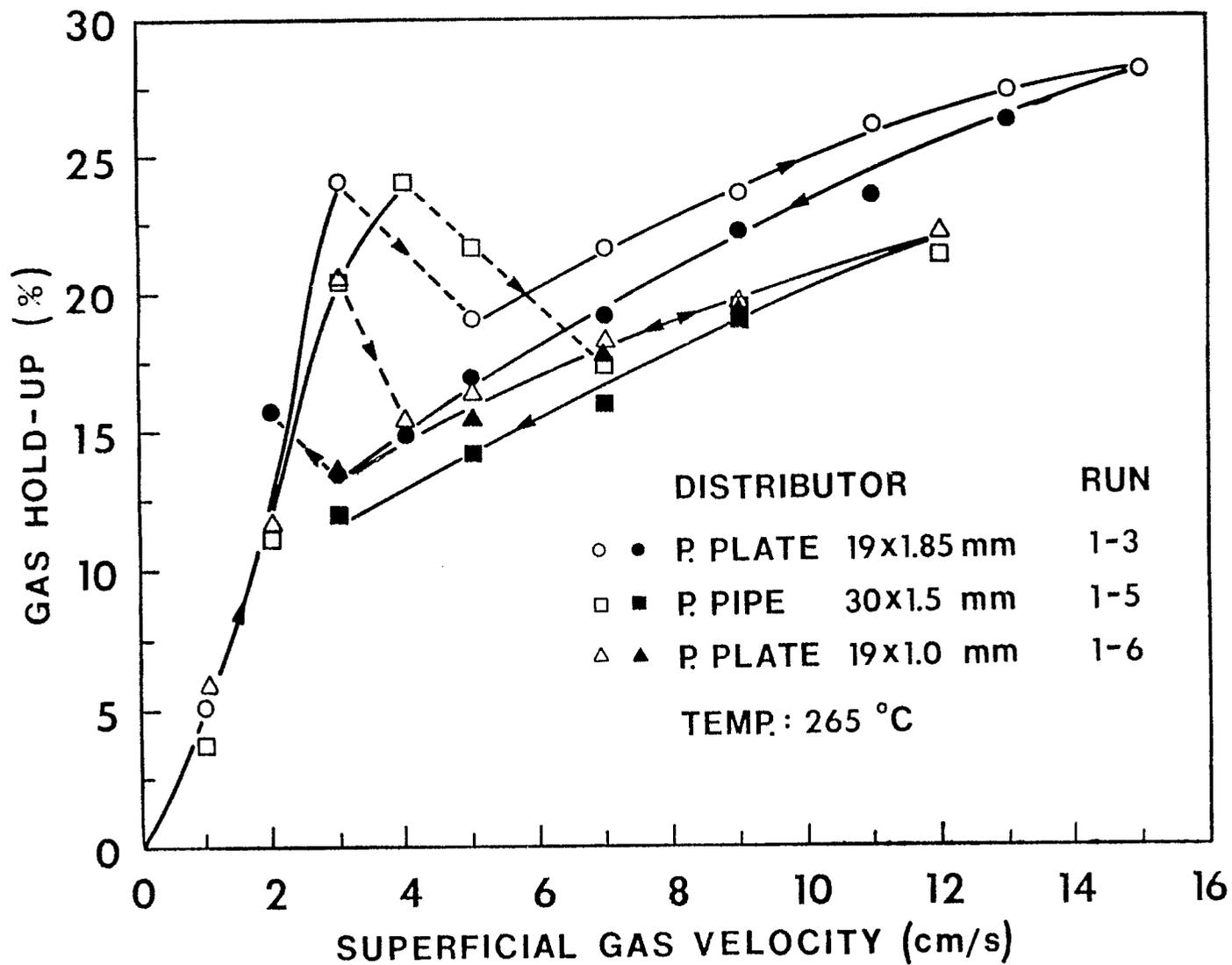
Figure 3. Effect of gas distributor type on gas hold-up in the AM-9G column (Open symbols: increasing gas flow rate; Solid symbols: decreasing gas flow rate).
