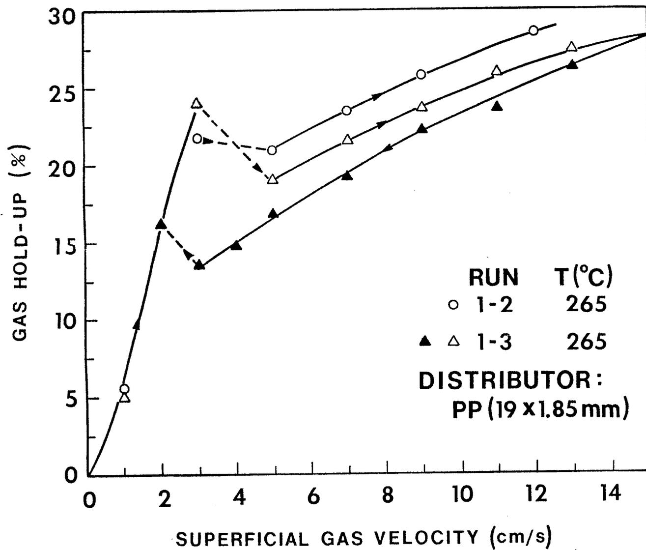
Figure 1. Effect of superficial gas velocity on gas hold-up in the AM-9G column (Open symbols: increasing gas flow rate, Solid symbols: decreasing gas flow rate).
