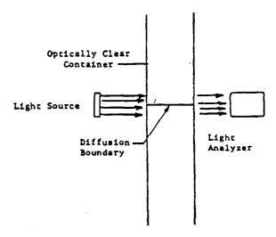
Figure 2.2. Illustration of the diaphragm cell and optical interference techniques.
