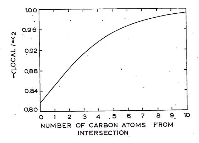
Figure 2: Ratio of  $\alpha_{local}$  to  $\alpha_2$  as a function of number of carbon atoms from intersection.  $\alpha_1$  = 0.6;  $\alpha_2$  = 0.9.
