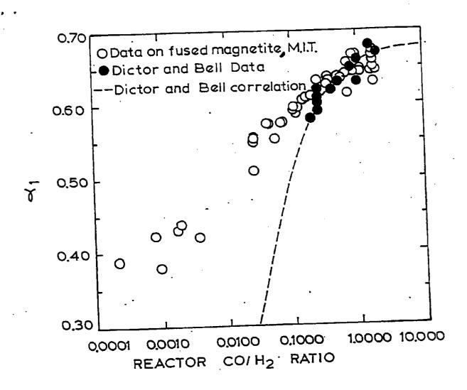
Figure 7 Comparison of present data and that of Huff<sup>18</sup> with data of Dictor and Bell<sup>20</sup>, all obtained on fused magnetite catalyst C73.
