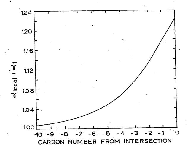
Figure 3: Ratio of  $\alpha_{local}$  to  $\alpha_{l}$  as a function of number of carbon atoms from intersection.  $\alpha_{l} = 0.6$ ;  $\alpha_{2} = 0.9$ .
