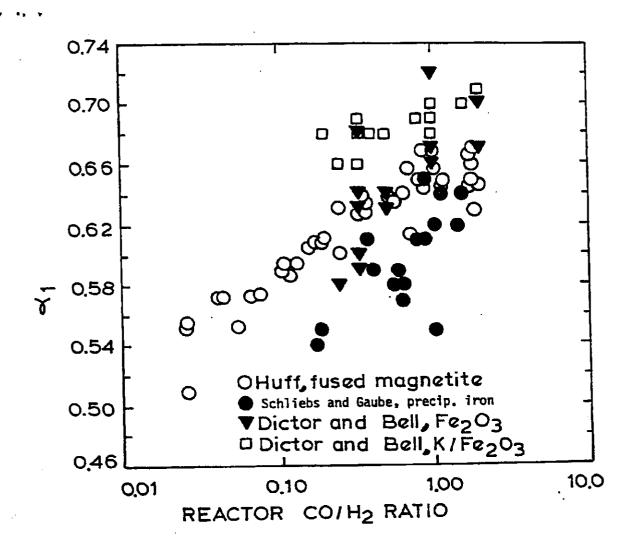
Figure 8 Comparison of  $\alpha_1$  versus CO/H $_2$  ratio from several iron catalysts.
