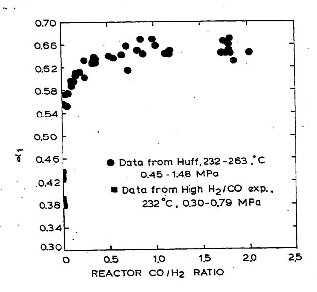
Figure 5 Effect of reactor  $CO/H_2$  ratio on  $\alpha_1$ .
