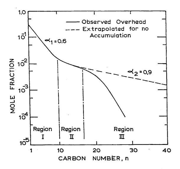
Figure 1: General form of Schulz-Flory plot for reactor effluent from an iron catalyst (after Huff<sup>18</sup>).
