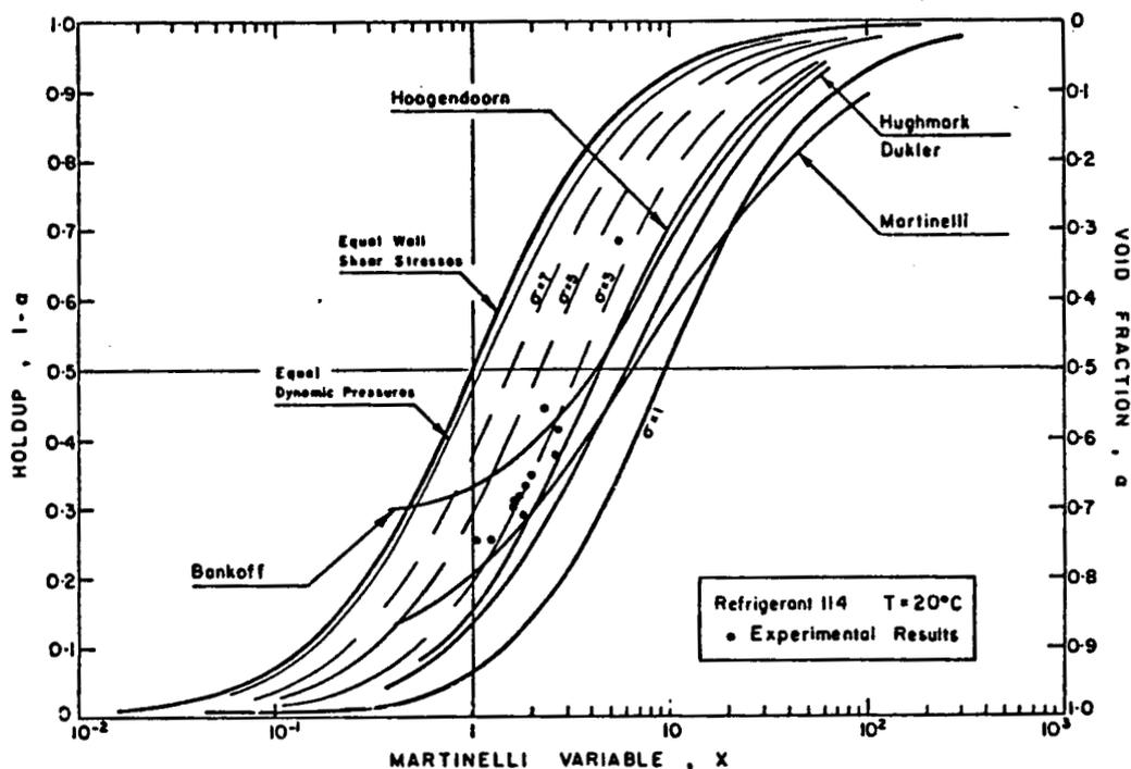
Fig. 10. Holdup as a function of Martinelli variable.
