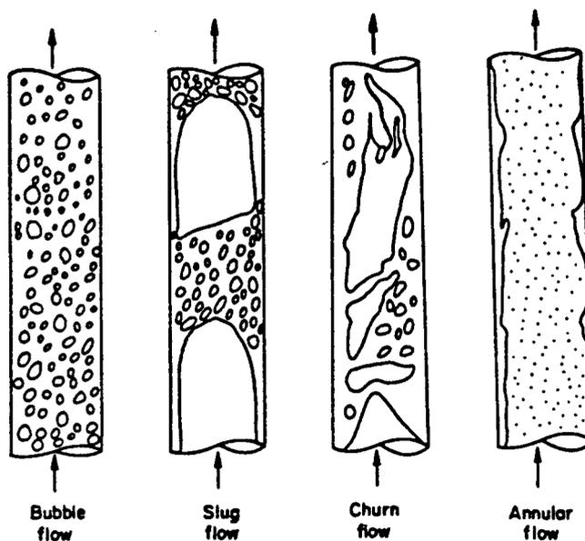
Fig. 2. Flow patterns for vertical two-phase flow.
