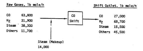
deeper CO shift (lower residual Co) is desired. For evaluation of the present accuracy, a value of 0.5 mole/mole dry gas may be taken as a guideline for the advanced gasifiers in conventional F-T plants.
