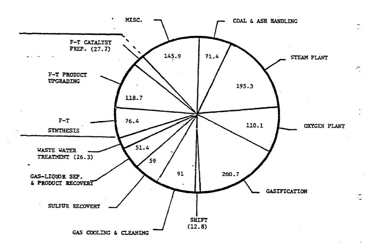
Figure 5-2. Plant Construction Costs for Mixed-output Case
