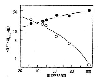
Figure 6-10. n-Butane Hydrogenolysis as a Function of Dispersion. The rates were measured at 473K (e), for low-temperature reduction and at 573K (e) for high-temperature reduction.
