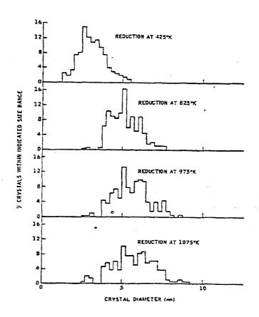
Figure 6-4. Variation of Particle Size Distribution with Reduction Temperature for Pt on Titanium Oxide
