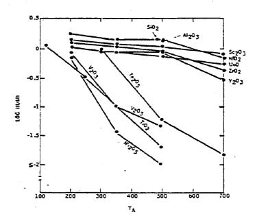
Figure 6-1. H<sub>2</sub> Chemisorption versus Temperature of Activation for Supported Iridium Catalysts. H/M = atoms hydrogen adsorbed at 25°C per atom iridium present in catalysts; T<sub>A</sub> = temperature of activation in hydrogen; wt% iridium = 1 for SiO<sub>2</sub>, Al<sub>2</sub>O<sub>3</sub>, V<sub>2</sub>O<sub>3</sub>, and HfO<sub>2</sub>; wt% iridium = 2 for all other catalysts.
