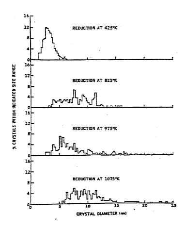
'Figure 6-7. Variation of Particle Size Distribution with Reduction Temperature for Pt on Carbon
