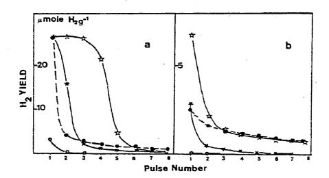
Figure 6-3. H<sub>2</sub> Yield from Pulses of Water Injected on Anatase-Supported Metals Reduced at (a) 773K and (b) 473K. One pulse = 27.5  $\mu$ mole.
