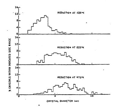
Figure 6-5. Variation of Particle Size Distribution with Reduction Temperature for Pt on Aluminum Oxide
