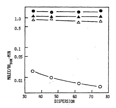
Figure 6-11. Cyclohexane Hydrogenolysis (ο)/Dehydrogenation (Δ) as a Function of Dispersion. The rates were measured at 573K for both low-temperature reduction (solid) and high-temperature reduction (open).
