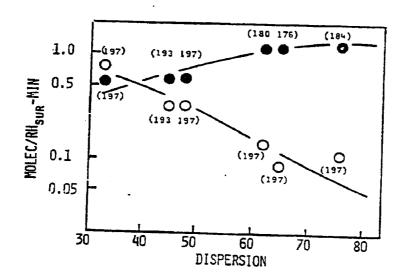
Figure 6-9. Ethane Hydrogenolysis as a Function of Dispersion. The number in parentheses by each point is the apparent activation energy in units of kJ/mol. The rates were measured at 523K (•) for low-temperature reduction and 623K (o) for high-temperature reduction.
