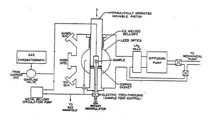
Figure 7-2. Schematic of UHV Surface Analysis System Equipped with Sample Isolation Cell for High-pressure (1-20 atm) Catalytic Studies
