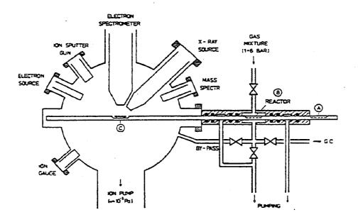
Figure 7-5. Schematic of UHV Apparatus with Attached Sample Transfer System and Microreactor for Catalytic Rate Measurements. The sample, located at the surface analysis position "C" (in the center of the UHV chamber), can be moved by pulling the stainless steel rod to position "B" (reactor for chemical reaction) or position "A" (the atmospheric loading position).
