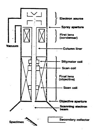
Figure 7-10. SEM Illumination System Showing the Parts of the System that Can Usually Be Controlled by the Operator.
