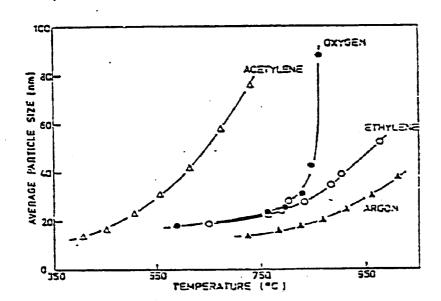
Figure 7-13. Variation of Palladium Average Particle Size with Temperature in Various Gaseous Environments (Graphite Support)
