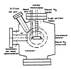
Figure 7-8. Schematic Diagram of the Spectrometer Chamber Showing the SIMS, Sample Carousel, Liquid Nitrogen Cooling System, and Ion Bombardment Gun.
