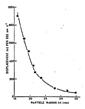
Figure 7-12. Variation of Particle Displacement Rate with Particle Radius for Silver Heated in 2.0 torr Hydrogen at 365°C
