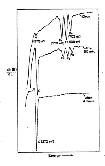
Figure 7-4. Auger Spectra of the Iron Surface before and after 30 min and after 4 h of Reaction. Reaction conditions: 6 atm, 3:1  $H_2$ :CO, 300°C.
