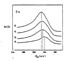
Figure 7-6. Carbon 1s XPS Data after Reaction.  $CO/H_2 = 1:20$ , T = 530K, reaction times: (a) 3 sec, (b) 23 sec, (c) 83 sec, and (d) 600 sec. Note shift in maximum.
