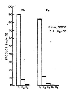
Figure 7-3. Comparison of Product Distributions Obtained over Initially Clean Polycrystalline Iron and Rhodium Foils
