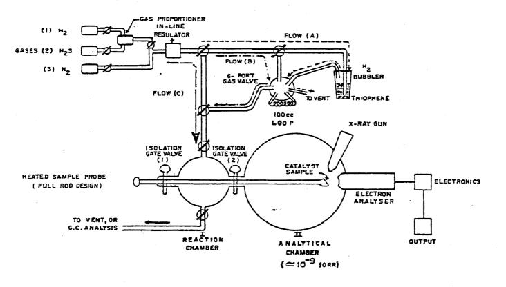
Figure 7-1. Schematic of the Experimental Configuration Used for the Direct Surface Examination of Reacted Catalyst Samples by XPS. Flow (A) (----) is used to load the 100 ml loop with hydrogen gas saturated with thiophene. Flow B (-----) is used to flush the loaded loop of thiophene/H<sub>2</sub> into the reactor. Flow C (- - -) is used to pass H<sub>2</sub>, H<sub>2</sub>S/H<sub>2</sub>, or N<sub>2</sub> directly into the reactor.
